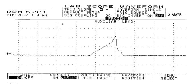
Fig. 15: Single Injector w/Normal Current Flow - Current Pattern
