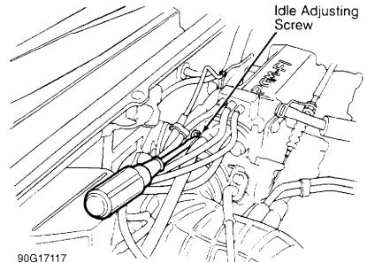
Fig. 9: Locating Idle Adj. Screw (Accord Shown; Other Models Similar) Courtesy of American Honda Motor Co., Inc.
