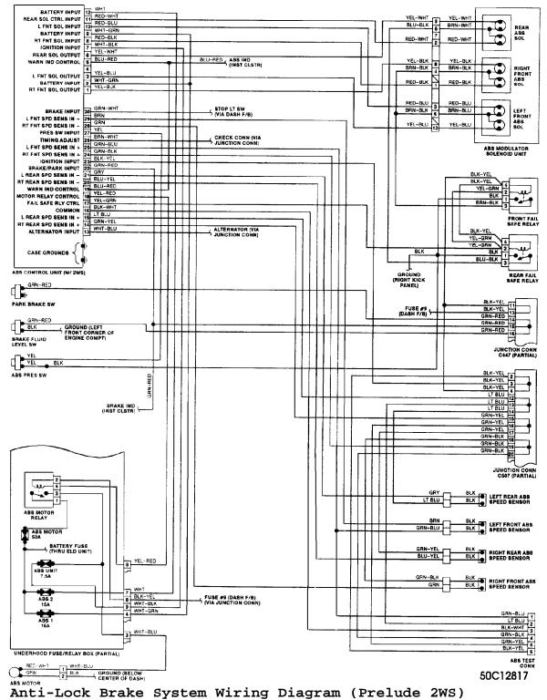
Fig. 34: Anti-Lock Brake System Wiring Diagram (Prelude 2WS)
