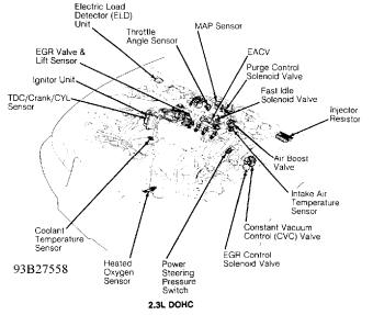
2.3L DOHC On rear of cylinder head, ELECTRICAL COMPONENT LOCATOR Article Text (p? 22)1958 Ptomose Parallel & Port Side Centre Nsk CA 950
