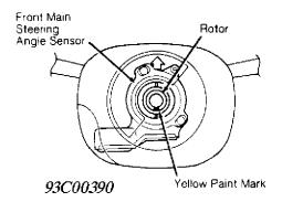
Fig. 3: Adjusting Front Main Steering Angle Sensor Courtesy of American Honda Motor Co., Inc.
