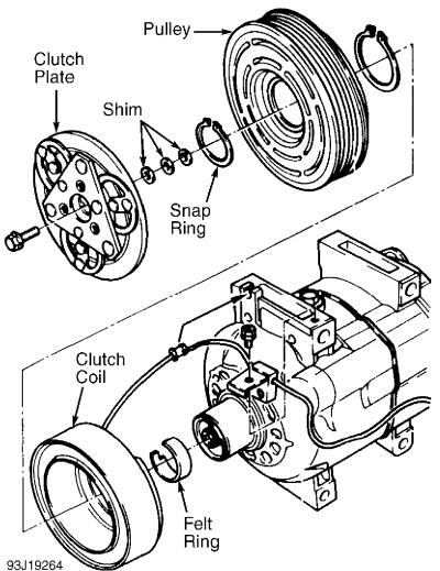
Fig. 20: Exploded View Of Compressor (Zexel 6-Cylinder) Courtesy of Audi of America, Inc.
