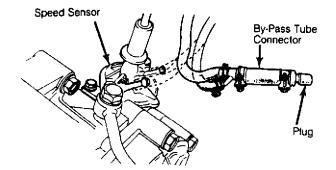
Fig. 3: Simulating High Speed Assist With By-Pass Tube Connector Courtesy of American Honda Motor Co., Inc.
