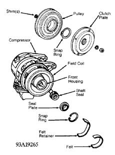
Fig. 13: Exploded View Of Compressor (Nippondenso 10-Cylinder)
