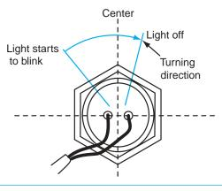
**Figure 13-35** Adjusting the front sub steering angle sensor.
