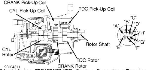
Fig. 5: Identifying TDC/CRANK/CYL Sensor Connector Terminals Courtesy of American Honda Motor Co., Inc.
