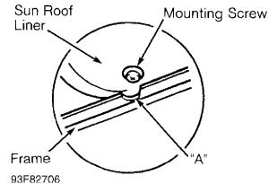
Fig. 5: Removing Sun Roof (Prelude) Courtesy of American Honda Motor Co., Inc.
