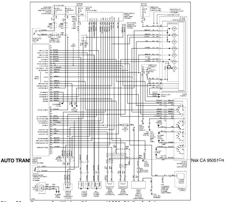
Fig. 53: Transaxle Wiring Diagram (1993-94 Prelude)
