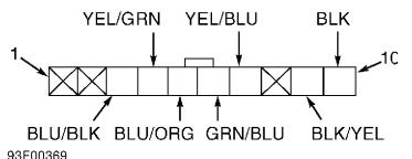
Fig. 1: Identifying Power Mirror Switch Connector Courtesy of American Honda Motor Co., Inc.
