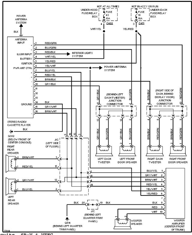
Radio Circuits, SR-V & VTEC SYSTEM WIRING DIAGRAMS Article Text (p. 10)1993 Honda PreludeFor Cadi Centre Nsk CA 95051Copyright
