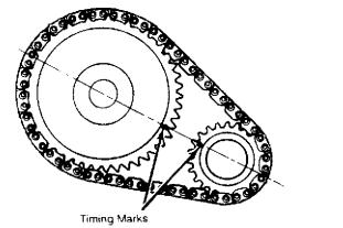
Fig. 24: Timing Gear Mark Alignment - Typical This Graphic For General Information Only
