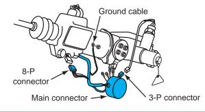
Figure 13-24 Installing wiring connectors on the rear steering actuator.
