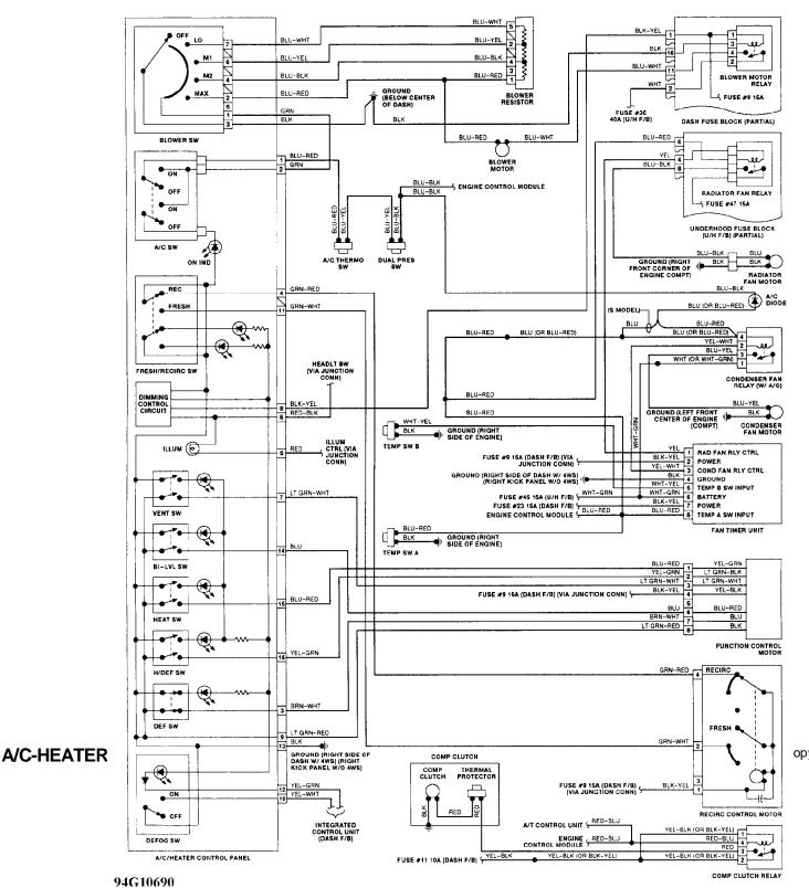
Fig. 11: Manual A/C-Heater System Wiring Diagram
