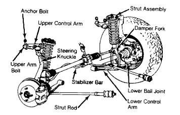
Fig. 1: Identifying Front Suspension Components (Typical) Courtesy of American Honda Motor Co., Inc.
