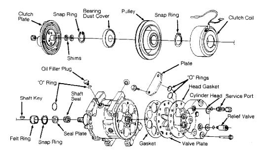
93119263 Fig. 18: Exploded View Of Compressor (Sanden 7-Cylinder) Courtesy of Hyundai Motor Co.
