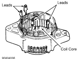
Fig. 6: Testing Stator Assembly Courtesy of American Honda Motor Co., Inc.
