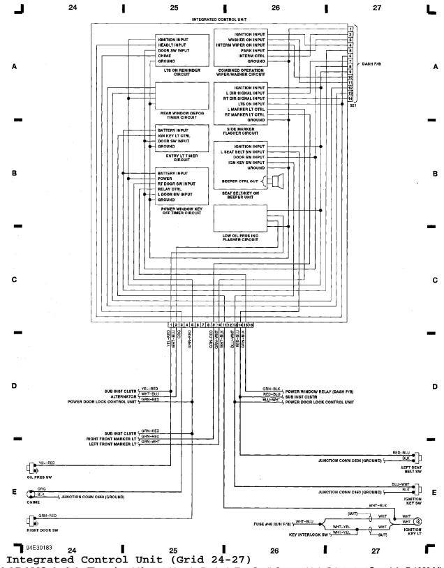
Fig. 7: Integrated Control Unit (Grid 24-27) WIRING DIAGRAMS Article Text (p. 10)1993 Honda PreludeFor Cadi Centre Nsk CA 95051Copyright © 1998 Mitche
