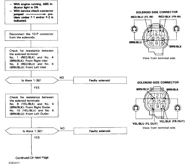
Fig. 29: Code 7-1 & 7-2 Flow Chart (1 Of 3), Front Solenoid Courtesy of American Honda Motor Co., Inc.
