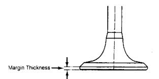
Fig. 9: Measuring Valve Head Margin - Typical This Graphic For General Information Only
