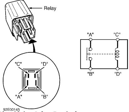
Fig. 2: Identifying Relay Terminals Courtesy of American Honda Motor Co., Inc.
