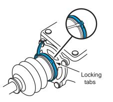
**Figure 13-19** Tightening and staking the inner tie-rod boot clamps.
