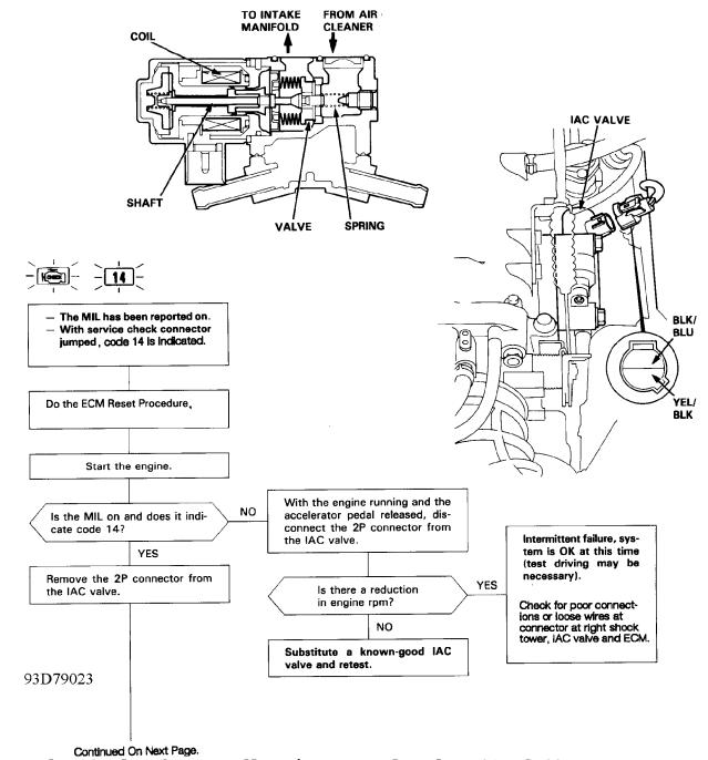
Fig. 28: Code 14 Flowchart, Idle Air Control Valve (1 of 2) Courtesy of American Honda Motor Co., Inc.
