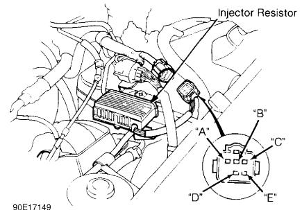
Fig. 9: Injector Resistor Connector Term. ID (Accord Shown; Prelude Similar) Courtesy of American Honda Motor Co., Inc.
