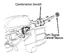
Fig. 4: Removing Turn Signal Cancel Sleeve & Combination Switch (Typical)
