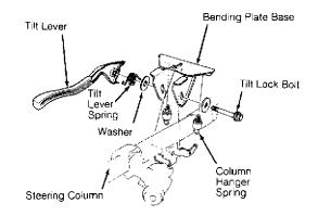
Fig. 5: Exploded View Of Tilt Lock Assembly (Typical) Courtesy of American Honda Motor Co.
