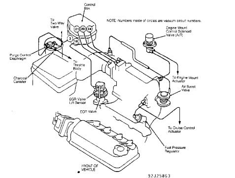
Fig. 3: Vacuum Diagram With Components (Accord - F22A1 Engine) Courtesy of American Honda Motor Co., Inc.
