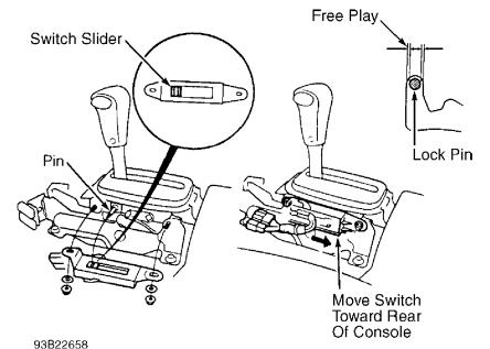
Fig. 29: Installing A/T Gear Position Switch Courtesy of American Honda Motor Co., Inc. AUTO TRANS DIAGNOSIS - MP1A Article Text (p. 35)1993 Honda PreludeFor Cadi Centre Nsk CA 95051<sup>Cor</sup>
