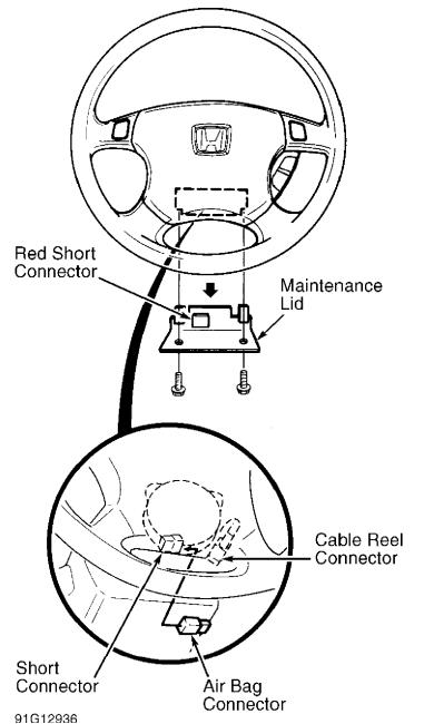
Fig. 1: Connecting Red Short Connector To Air Bag Connector Courtesy of American Honda Motor Co., Inc.
