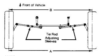
26695 Fig. 2: Adjusting Tie Rod Sleeves (Top View)
