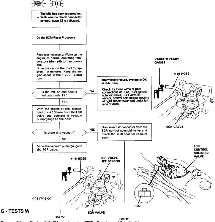
Fig. 22: Code 12 Flowchart, EGR System (1 of 5) Courtesy of American Honda Motor Co., Inc.
