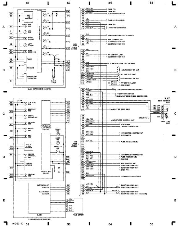
**Fig. 14:** Sub Instrument Cluster, Main Instrument Cluster (Grid 52-55) WIRING DIAGRAMS Article Text (p. 17)1993 Honda PreludeFor Cadi Centre Nsk CA 95051Copyright © 1998 Mitche
