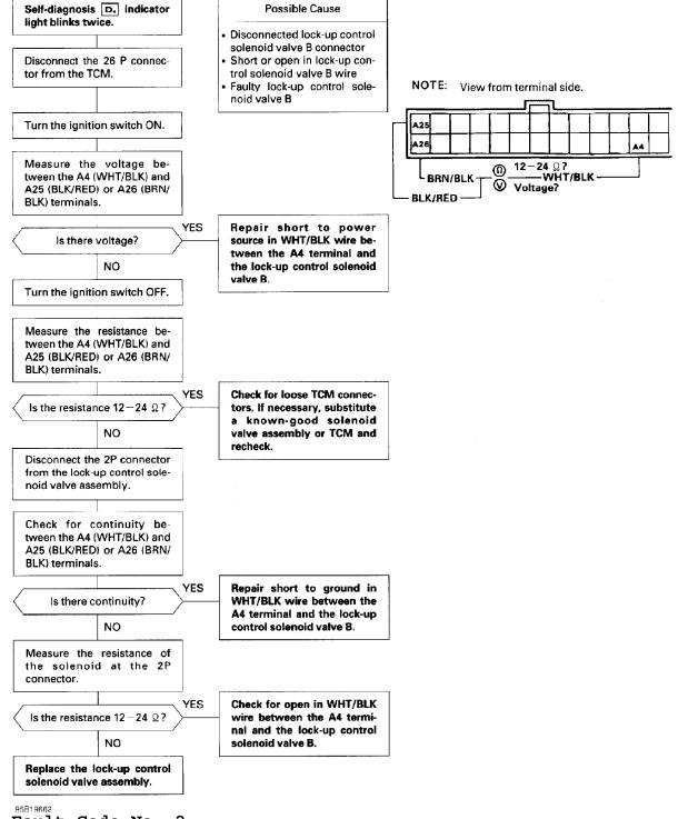
Fig. 36: Fault Code No. 2
