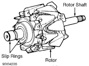
Fig. 5: Testing Rotor Assembly Courtesy of American Honda Motor Co., Inc.
