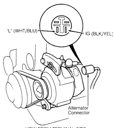
93H00346 VIEW FROM TERMINAL SIDE Fig. 1: Testing Alternator Output On Harness Connector Terminals Courtesy of American Honda Motor Co., Inc.
