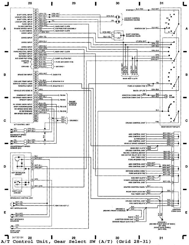
Fig. 8: A/T Control Unit, Gear Select SW (A/T) (Grid 28-31) WIRING DIAGRAMS Article Text (p. 11)1993 Honda PreludeFor Cadi Centre Nsk CA 95051Copyright © 1998 Mitche
