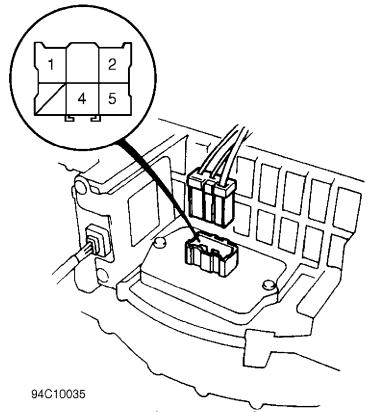
Fig. 3: Blower Motor Resistor Terminal ID Courtesy of American Honda Motor Co., Inc.
