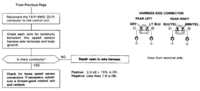
DTC 5, 5-4 & 5-8: (2 OF 2) SPEED SENSOR(S) PRELUDE
