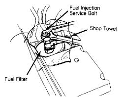
Fig. 4: Releasing Fuel System Pressure Courtesy of American Honda Motor Co., Inc.
