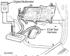
Fig. 4: Connecting Test Harness Courtesy of American Honda Motor Co., Inc.
