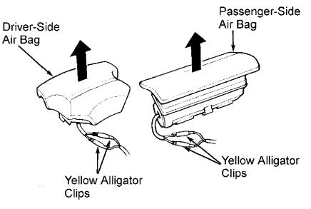
93J75100 Fig. 7: Deploying Air Bag Module Out Of Vehicle Courtesy of American Honda Motor Co., Inc.
