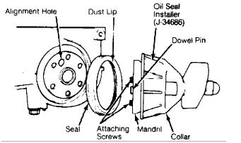
Fig. 27: Installing Typical One-Piece Oil Seal This Graphic For General Information Only
