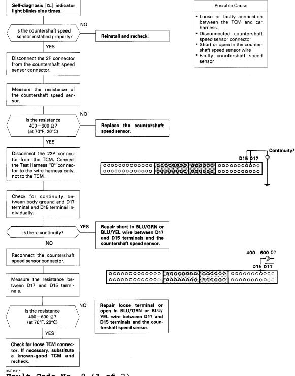
Fig. 45: Fault Code No. 9 (1 of 2)
