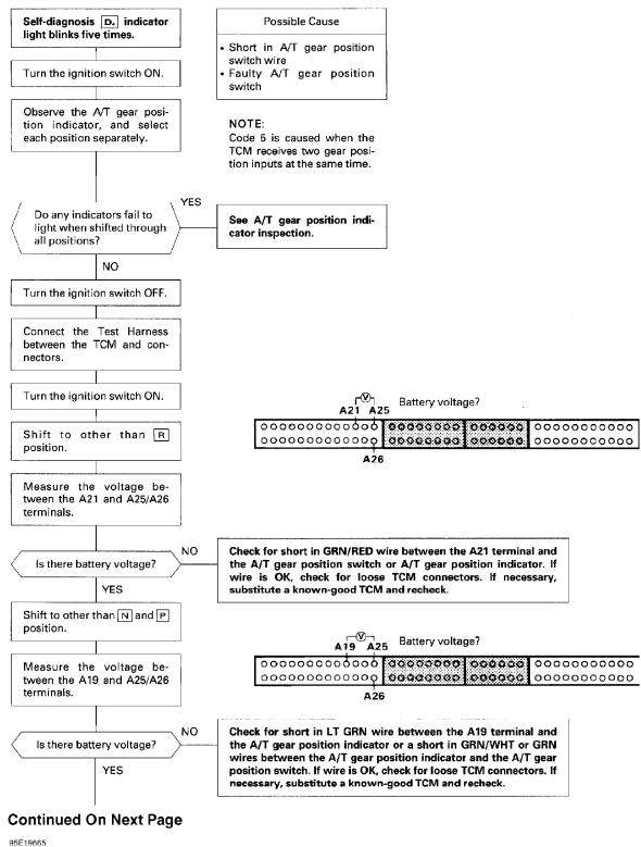
Fig. 39: Fault Code No. 5 (1 of 2)
