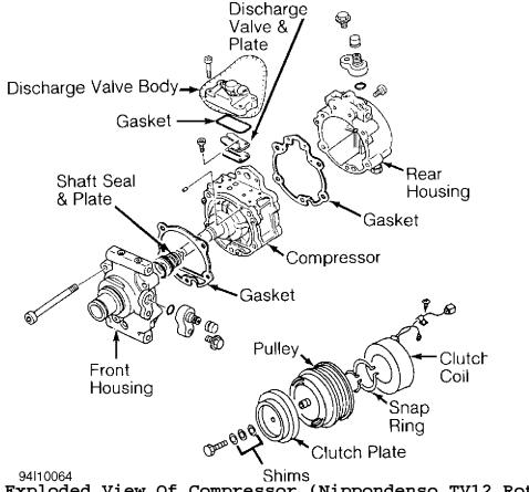
Fig. 12: Exploded View Of Compressor (Nippondenso TV12 Rotary Vane) Courtesy of Mazda Motors Corp.
