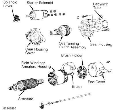
Fig. 7: Exploded View Of Starter (Mitsuba) Courtesy of American Honda Motor Co., Inc. STARTER Article Text (p. 7)1993 Honda PreludeFor Cadi Centre Nsk CA 95051Copyright© 1998 Mitchell Repair Informa
