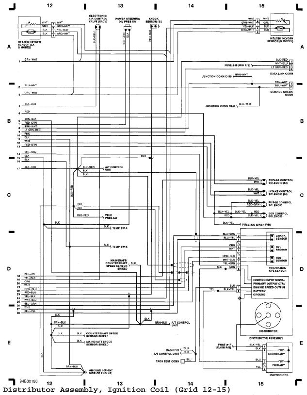
Fig. 4: Distributor Assembly, Ignition Coil (Grid 12-15) WIRING DIAGRAMS Article Text (p. 7)1993 Honda PreludeFor Cadi Centre Nsk CA 95051Copyright © 1998 Mitchell
