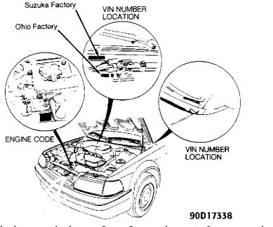
Fig. 3: Civic & Civic Del Sol Engine Code Location Courtesy of American Honda Motor Co., Inc.
