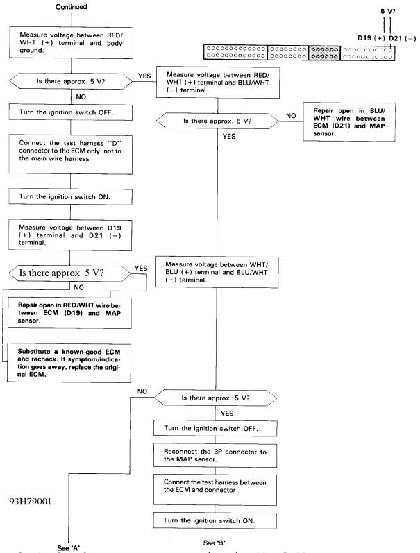
Fig. 10: Code 3 Flowchart, MAP Sensor Circuit (2 of 3) Courtesy of American Honda Motor Co., Inc.
