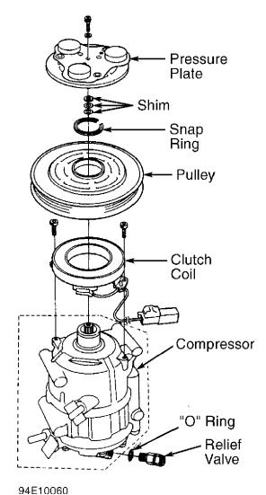
Fig. 7: Exploded View Of Compressor (Hadsys 7-Cylinder) Courtesy of American Honda Motor Co., Inc.
