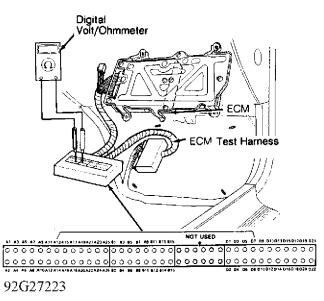
Fig. 2: Installing PGM-FI ECM Test Harness & Identifying Terminals Courtesy of American Honda Motor Co., Inc.
