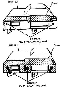
Fig. 18: Identifying SRS Control Units (Accord) Courtesy of American Honda Motor Co., Inc.
