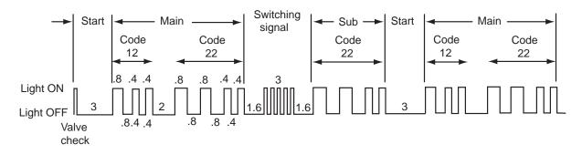
Figure 13-2 Trouble codes in main and sub processors obtained with engine running.
