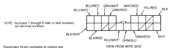
Disconnect 18-pin connector to control unit.
