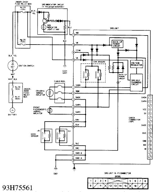
Fig. 28. SRS Wiring Diagram (Civic With Passenger-Side Air Bag) AIR BAG RESTRAINT SYSTEM Article Jext (p. 34)1993 Honda PreludeFor Cadi Centre NSK CA 95051 Copyrig Courcesy of American Honda Motor (p. ., Inc.
