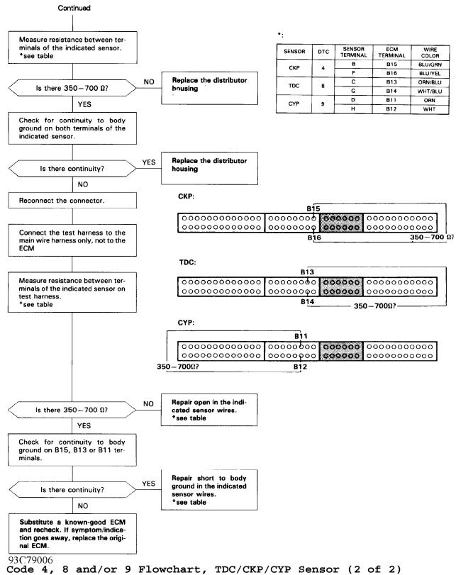
Fig. 13: Code 4, 8 and/or 9 Flowchart, TDC/CKP/CYP Sensor (2 of 2) Courtesy of American Honda Motor Co. Inc. G-TESTS W/CODES Article Text (p. 16) 1993 Honda PreludeFor Cadi Centre Nsk CA 95051 Copyright © 1998 Mitc
