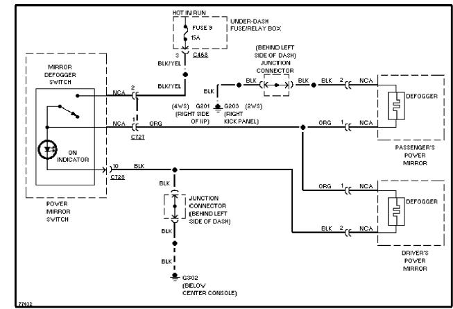
Heated Mirrors Circuit
