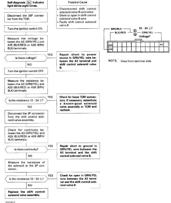
Fig. 44: Fault Code No. 8
