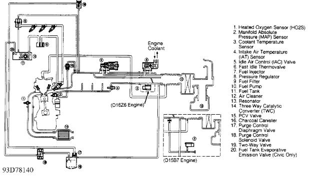
Fig. 7: Vacuum Diagram W/O Components (Civic/Del Sol D15B7 & D16B6 Eng.)
