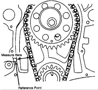
Fig. 23: Measuring Timing Chain Stretch - Typical This Graphic For General Information Only
