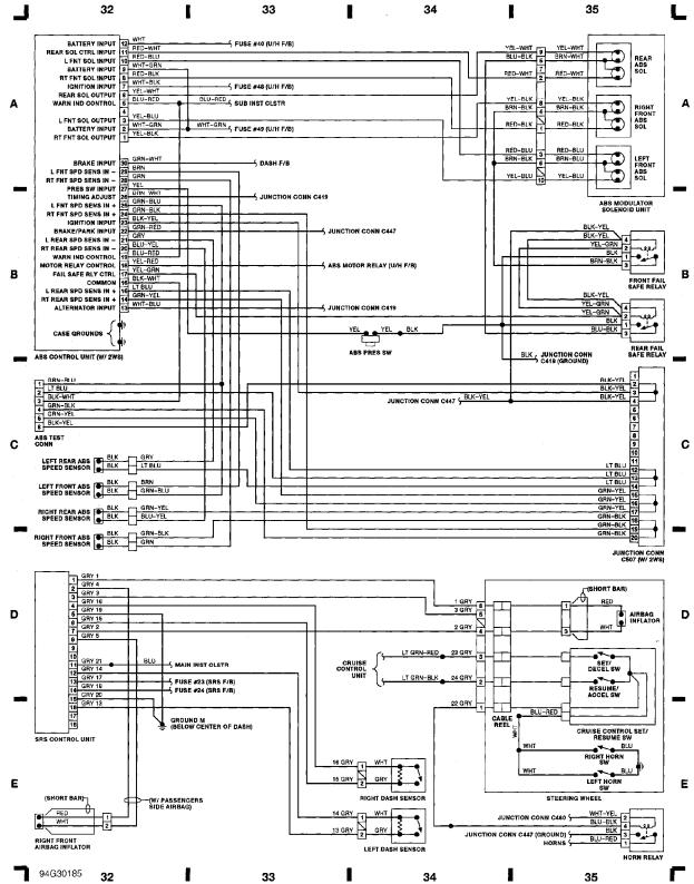
94G3018532333435Fig.Fig. 9: ABS Control Unit (W/ 2WS), SRS Control Unit (Grid 32-35)WIRING DIAGRAMS Article Text (p. 12)1993 Honda PreludeFor Cadi Centre Nsk CA 95051Copyright © 1998 Mitche
