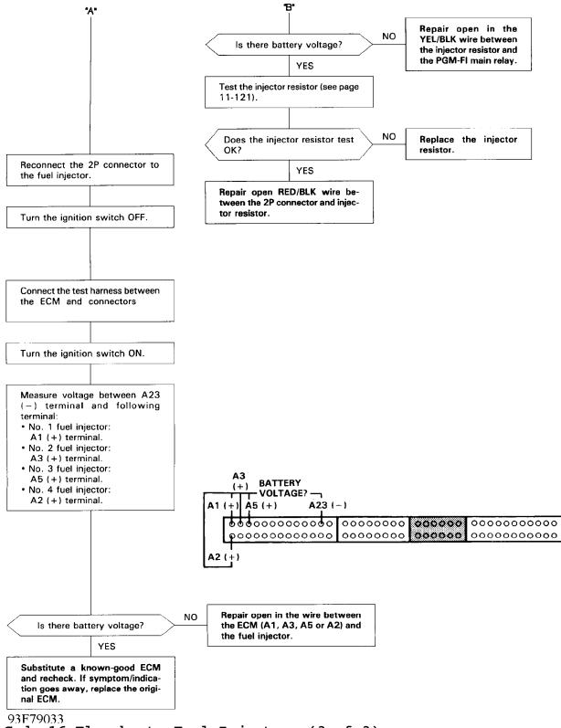
Fig. 34: Code 16 Flowchart, Fuel Injectors (3 of 3) Courtesy of American Honda Motor Co., Inc.
