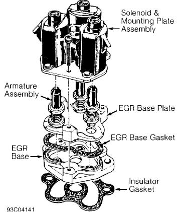
Fig. 11: Typical Digital EGR Valve Courtesy of General Motors Corp.
