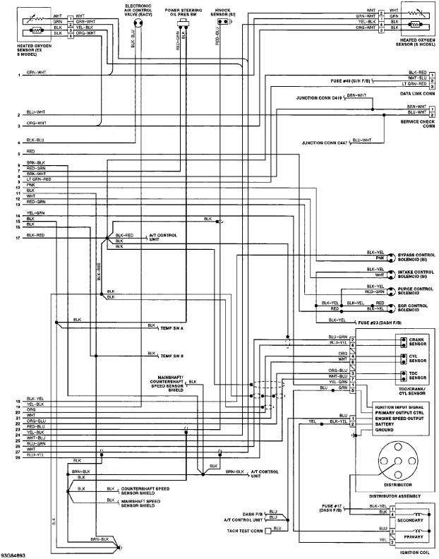
Fig. 7: Wiring Diagram (Prelude 2.2L & 2.3L - 2 Of 2)
