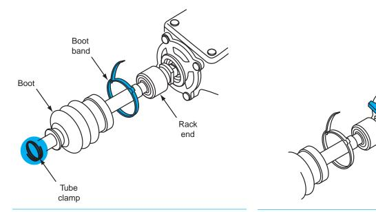
**Figure 13-10** Removing boot bands and clamps from the inner tie-rod end.
