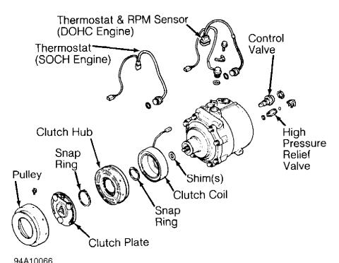
Fig. 16: Exploded View Of Compressor (Sanden Scroll) Courtesy of Chrysler Corp.
