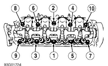
Fig. 7: Tightening Sequence For Cylinder Head Bolts (2.2L DOHC & 2.3L)
