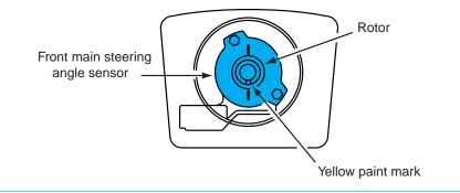
**Figure 13-32** Yellow paint mark on the front main steering angle sensor indicating the electronically neutral sensor position.
