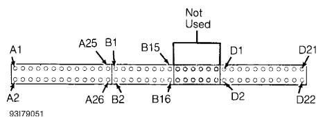
Fig. 3: Identifying ECM Terminals Courtesy of American Honda Motor Co., Inc.
