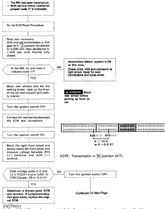
Fig. 35: Code 17 Flowchart, Vehicle Speed Sensor (1 of 2) Courtesy of American Honda Motor Co., Inc.
