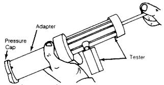
Fig. 2: Testing Radiator Pressure Cap
