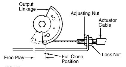
93H01480 Fig. 1: Adjusting Cruise Control Actuator Cable Courtesy of American Honda Motor Co., Inc.
