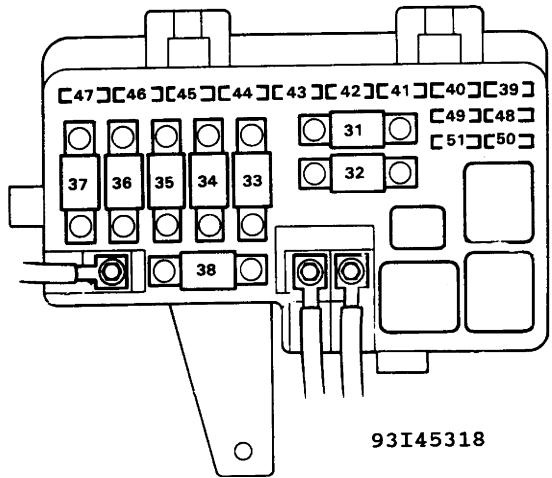
Fig. 2: Underhood Fuse & Relay Panel Identification (1992-94) Courtesy of American Honda Motor Co., Inc.
