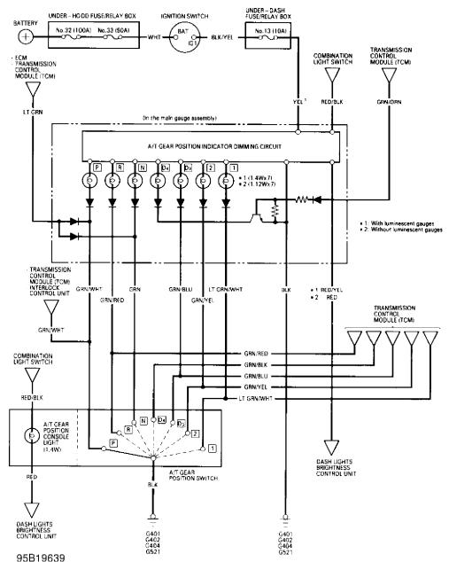
Fig. 19: A/T Gear Position Indicator Wiring Schematic (1994) ANTO TRANS DIAGNOSIS - MPTA ANTORNO (p. 23) 4993 Honda PreludeFor Cadi Centre Nsk CA 95051Cor
