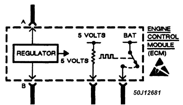
Fig. 2: Sample Schematic Showing Typical ESD Sensitive Device
