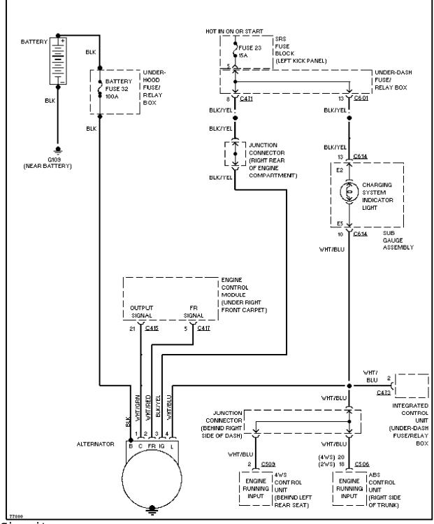
Charging Circuit SYSTEM WIRING DIAGRAMS Article Text (p. 11)1993 Honda PreludeFor Cadi Centre Nsk CA 95051Copyright
