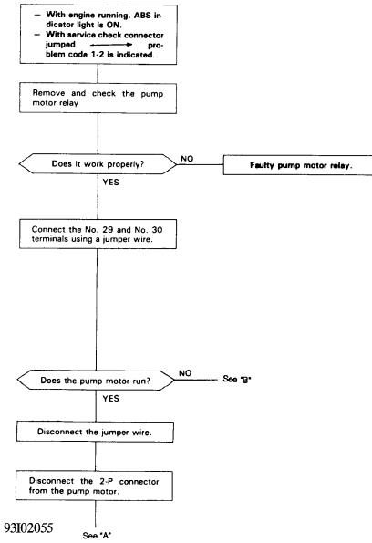
Fig. 12: Code 1-2 Flow Chart (1 Of 3), Pump Motor Circuit Courtesy of American Honda Motor Co., Inc. ANTI-LOCK BRAKE SYSTEM Article Text (p. 18)1993 Honda PreludeFor Cadi Centre Nsk CA 95051Copyright (
