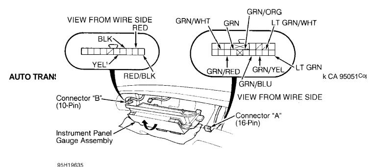
Fig. 15: Testing A/T Gear Position Indicator (1994, 2 of 3) Courtesy of American Honda Motor Co., Inc.
