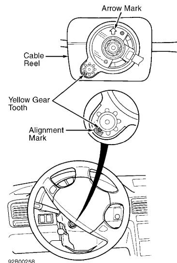
92B00258 Fig. 8: Locating Cable Reel Alignment Marks Courtesy of American Honda Motor Co., Inc.
