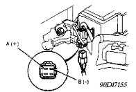
Fig. 11: Identifying EGR System Connector Terminals (Accord) Courtesy of American Honda Motor Co., Inc.
