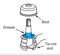
Figure 13-13 Packing the boot and tie-rod end with grease.
