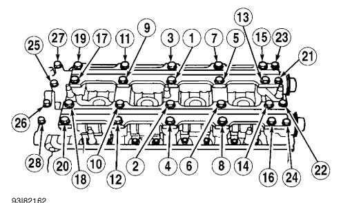
Fig. 11: Tightening Sequence For Camshaft Bolts (2.2L DOHC) Courtesy of American Honda Motor Co., Inc.
