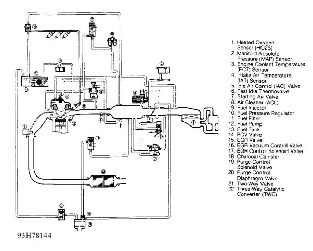
Fig. 1: Vacuum Diagram Without Components (Accord - F22A1 Engine) Courtesy of American Honda Motor Co., Inc.
