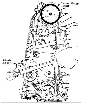
Fig. 26: Timing Belt Tension Adjustment - Typical This Graphic For General Information Only
