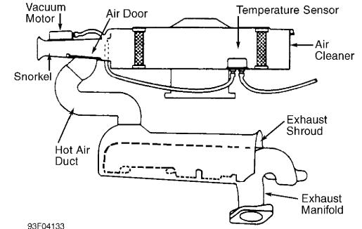
Fig. 3: Typical Thermostatic Air Cleaner System
