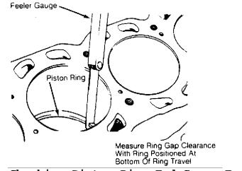
Fig. 15: Checking Piston Ring End Gap - Typical This Graphic For General Information Only
