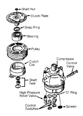
94G10062 Fig. 9: Exploded View Of Compressor (Harrison V5 5-Cylinder) Courtesy of General Motors Corp.
