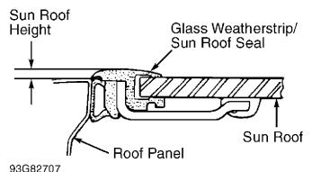
Fig. 1: Measuring Sun roof Height (Prelude) Courtesy of American Honda Motor Co., Inc.
