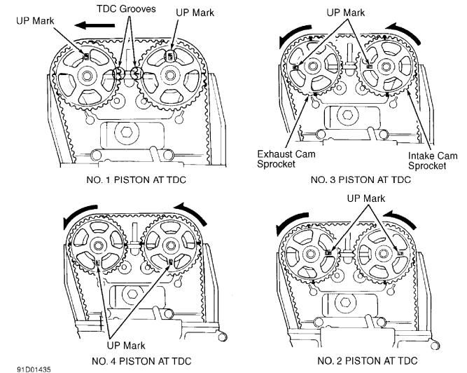
Fig. 2: Positioning Camshaft Sprockets For Valve Clearance (2.2L DOHC & 2.3L)
