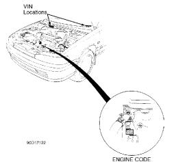
Fig. 1: Accord Engine Code Location Courtesy of American Honda Motor Co., Inc.
