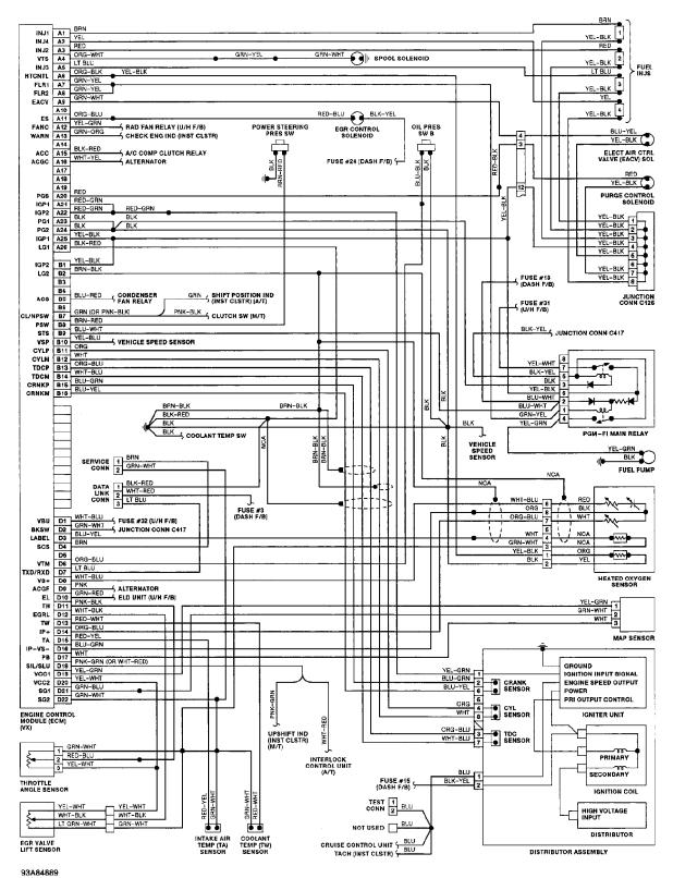
Fig. 3: Wiring Diagram (Civic 1.5L - VX - VTEC-E)
