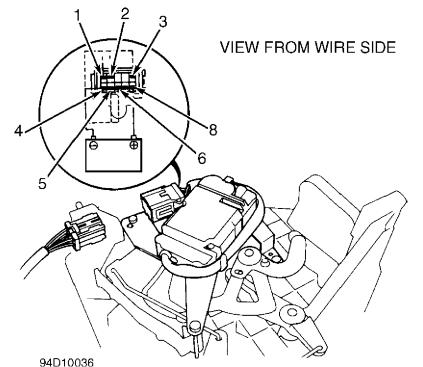
Fig. 8: Function Control Motor Connector Terminal ID Courtesy of American Honda Motor Co., Inc.
