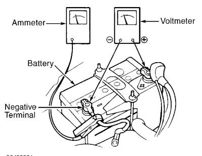
93J82221 Fig. 1: Starter Cranking Test Courtesy of American Honda Motor Co., Inc.
