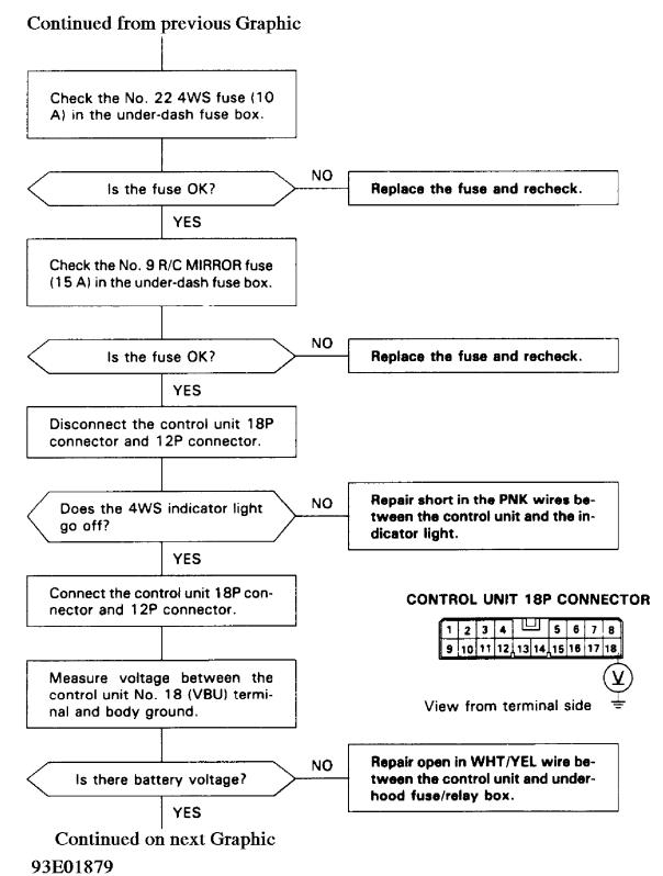
Fig. 12: 4WS Indicator Light Circuit (2 Of 3) Courtesy of American Honda Motor Co., Inc.
