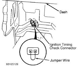
Fig. 8: Locating Ignition Timing Check Connector (Prelude) Courtesy of American Honda Motor Co., Inc.
