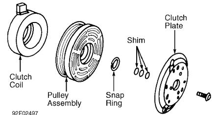
Fig. 6: Exploded View Of Compressor Clutch (Ford FX-15) Courtesy of Mazda Motors Corp.
