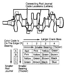
Fig. 17: Connecting Rod Journal & Bearing Identification Codes Courtesy of American Honda Motor Co., Inc. 2.2L 4-CYL & 2.3L 4-CYLArticle Text (p. 27)1993 Honda PreludeFor Cadi Centre Nsk CA 95051<sup>Copyright © 1998</sup>
