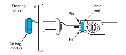
Figure 13-33 Proper alignment of the steering wheel openings and cable reel pins.
