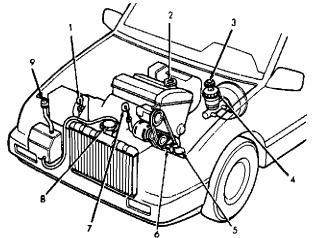
1. Automatic Transmission Dipstick 2. Engine Oil Filler Cap 3. Clutch Fluid Reservoir 4. Brake Fluid Reservoir 5. Washer Fluid Reservoir
