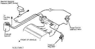
Fig. 8: Vacuum Diagram W/ Components (Civic/Del Sol D15B7 Eng.) Courtesy of American Honda Motor Co., Inc.
