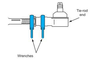
Figure 13-9 Loosening the tie-rod end locknut.
