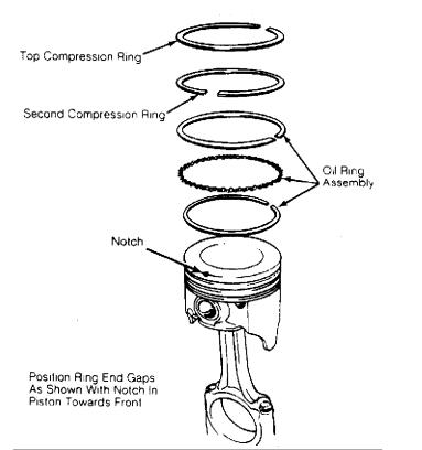
Fig. 16: Typical Piston Ring End Gap Positioning - Typical This Graphic For General Information Only
