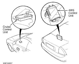
Fig. 28: Identifying Cruise Control Unit & 4WS Control Unit Courtesy of American Honda Motor Co., Inc.
