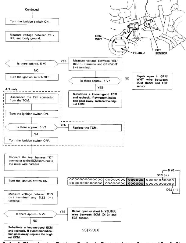
Fig. 17: Code 6 Flowchart, Engine Coolant Temperature Sensor (2 of 2) GouleSTS WCODES: Article Text (pm20) 1993 Honda PreludeFor Cadi Centre Nsk CA 95051 Copyright © 1998 Mitc
