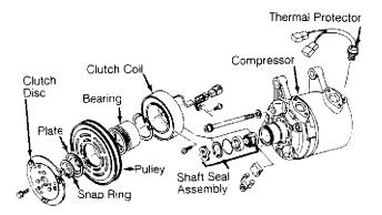
94C10068 Fig. 19: Exploded View Of Compressor (Zexel Rotary Vane) Courtesy of Nissan Motor Co., U.S.A.
