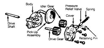
Fig. 32: Typical Gear Type Oil Pump This Graphic For General Information Only
