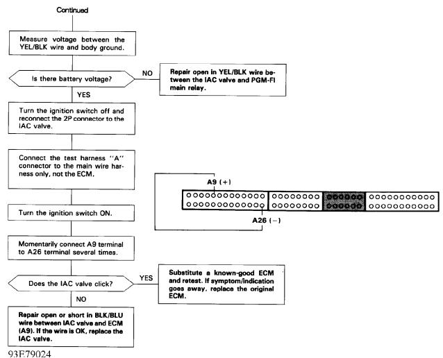
Fig. 29: Code 14 Flowchart, Idle Air Control Valve (2 of 2) Courtesy of American Honda Motor Co., Inc.
