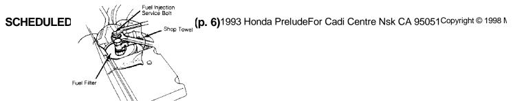
Fig. 4: Releasing Fuel System Pressure Courtesy of American Honda Motor Co., Inc.
