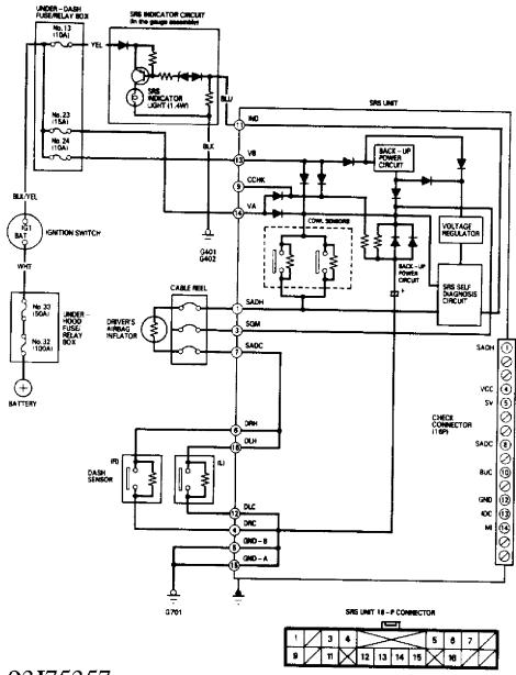
$93J75357_{\mbox{SRS}}$  Wiring Diagram (Prelude Without Passenger-Side Air Bag) Fig. 32: Courtesy of American Honda Motor Co., Inc. AIR BAG RESTRAINT SYSTEM Article Text (p. 38)1993 Honda PreludeFor Cadi Centre Nsk CA 95051Copyrig
