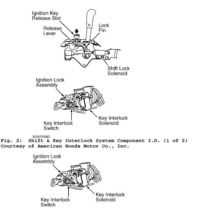
93B22641 Fig. 3: Shift & Key Interlock System Component I.D. (2 of 2) AUTO IBANS DIAGNOSIS - MP1A Articler Text (p. 4)1993 Honda PreludeFor Cadi Centre Nsk CA 95051Copy
