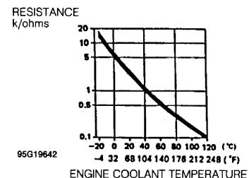
Fig. 23: Checking Engine Coolant Temperature Sensor Resistance Courtesy of American Honda Motor Co., Inc.
