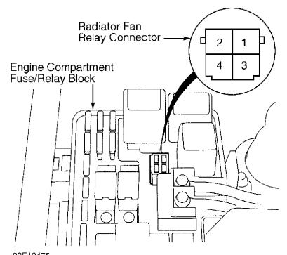
93E19475 Fig. 3: Radiator Fan Relay Connector Terminal ID Courtesy of American Honda Motor Co.
