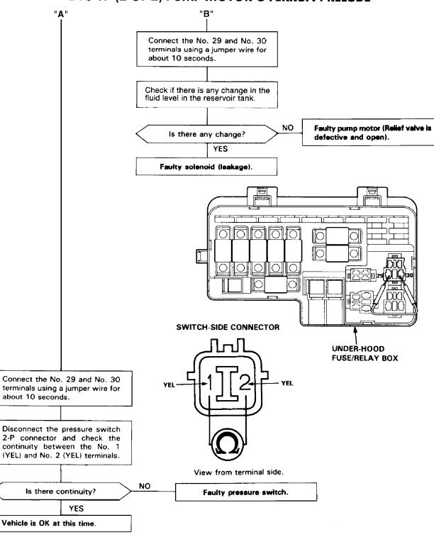
DTC 1: (2 OF 2) PUMP MOTOR OVERRUN PRELUDE
