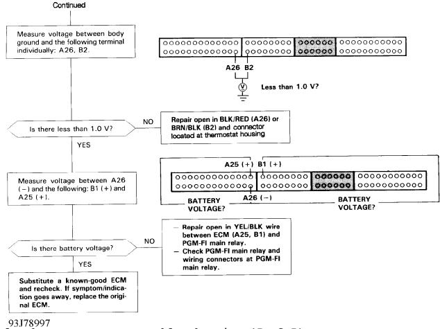
Fig. 7: Flowchart, No Start Trouble Shooting (5 of 5) Courtesy of American Honda Motor Co., Inc.
