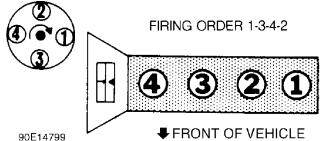
Fig. 1: Firing Order & Distributor Rotation (Accord) Courtesy of American Honda Motor Co., Inc.
