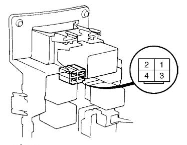
93G19428 Fig. 2: Blower Relay Socket Terminal ID Located Inside Underdash Fuse/Relay Box
