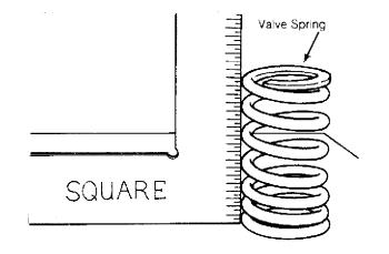
Fig. 4: Checking Valve Spring Squareness - Typical This Graphic For General Information Only
