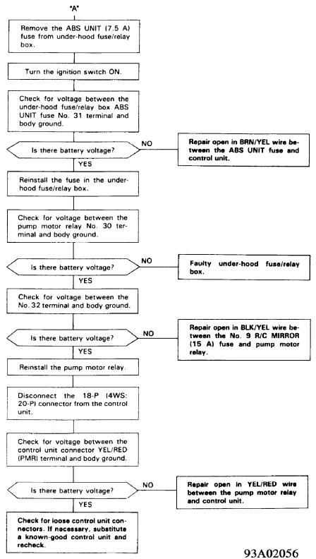
Fig. 13: Code 1-2 Flow Chart (2 Of 3), Pump Motor Circuit Courtesy of American Honda Motor Co., Inc.
