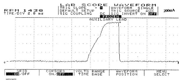
Fig. 12: Single Injector w/Normal Current Flow - Current Pattern WAVEFORMS - INJECTOR PATTERN TUTORIAL Article Text (p. 22)1993 Honda PreludeFor Cadi Centre EXAMPLE #5 - CURRENT CONTROLLED DRIVER The known-good waveform inFig. 13 is from a Chrysler 3.0L V6 PFI VIN [3]. It is a perfect example of the peak and hold theory. The waveform shows a 1-amp per division current flow, ramping to 4 amps and then decreasing to 1-amp to hold the injector open.
