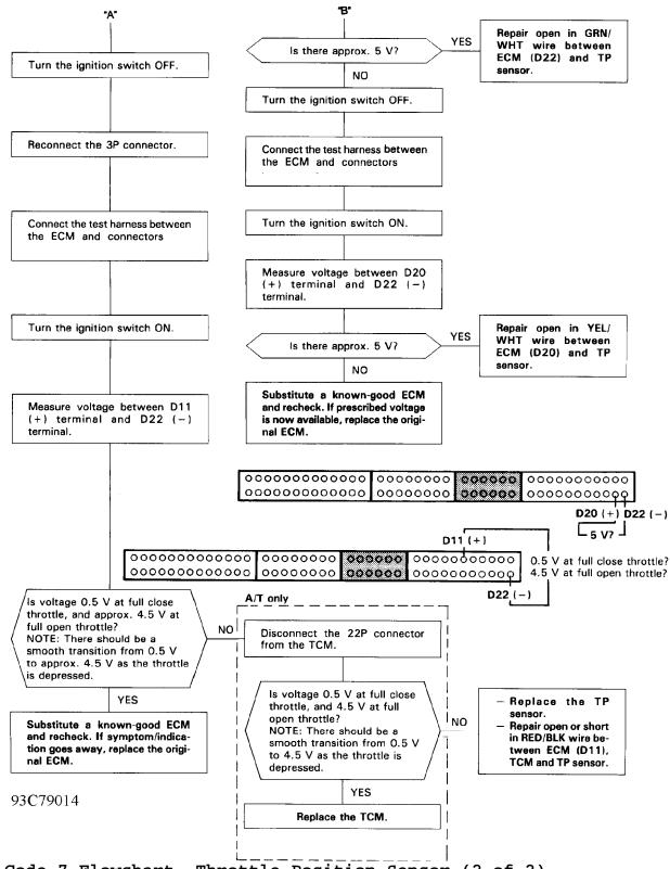
Fig. 19: Code 7 Flowchart, Throttle Position Sensor (2 of 2) Courtesy of American Honda Motor Co., Inc.
