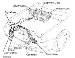
Fig. 1: Manual A/C-Heater System Component ID Courtesy of American Honda Motor Co.
