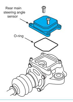
Figure 13-21 Removing the rear main steering angle sensor.
