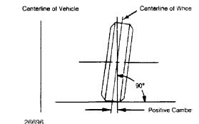
Fig. 3: Determining Camber Angle
