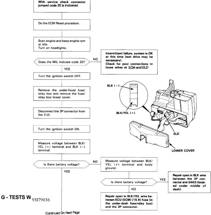
Fig. 37: Code 20 Flowchart, Electrical Load Detector (1 of 2) Courtesy of American Honda Motor Co., Inc.
