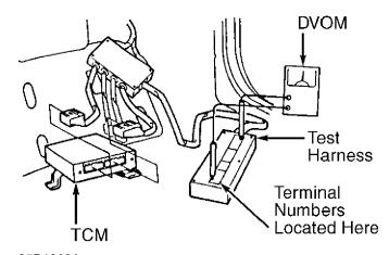
95D19631 Fig. 11: Installing Test Harness Courtesy of American Honda Motor Co., Inc.
