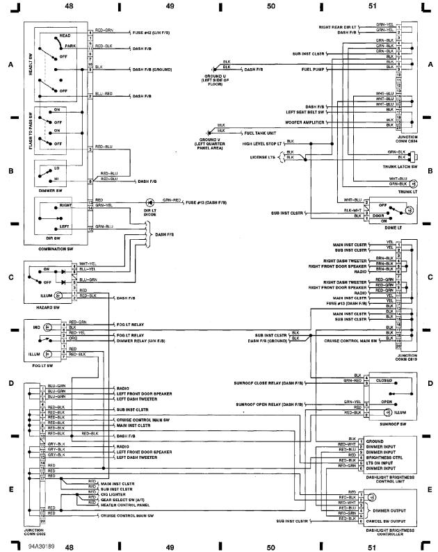
J94A3018948495051FFig. 13:Combination Sw, Sunroof Sw, Dashlights (Grid 48-51)WIRING DIAGRAMS Article Text (p. 16)1993 Honda PreludeFor Cadi Centre Nsk CA 95051Copyright © 1998 Mitche
