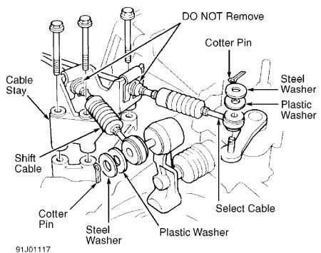
Fig. 2: Removing Shift Cable Assembly Courtesy of American Honda Motor Co., Inc. CLUTCH Article Text (p. 2)1993 Honda PreludeFor Cadi Centre Nsk CA 95051Copyright © 1998 Mitchell Repair Informati
