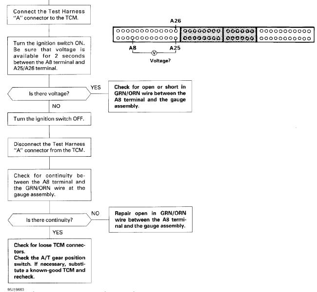
Fig. 34: Circuit Check "D4" Light Will Not Come On (2 of 2)
