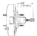
Fig. 4: Adjusting Power Brake Booster Push Rod Length Courtesy of American Honda Motor Co., Inc.
