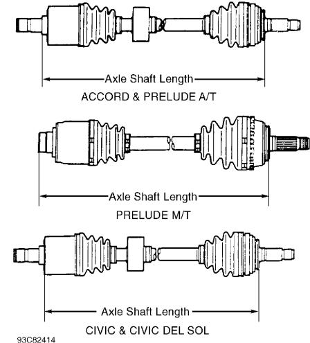
Fig. 3: Measuring Drive Axle Shaft Assembled Length Courtesy of American Honda Motor Co., Inc.
