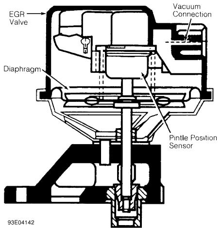
Fig. 12: Cutaway View Of Typical Integrated Electronic EGR Valve Courtesy of General Motors Corp.
