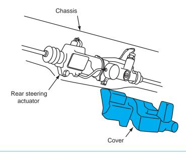
Figure 13-5 Removing the rear steering actuator cover.
