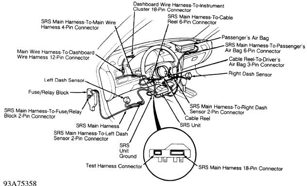
Fig. 14: Locating SRS Components (Accord Shown W/ Pass. Side Air Bag) Courtesy of American Honda Motor Co., Inc.
