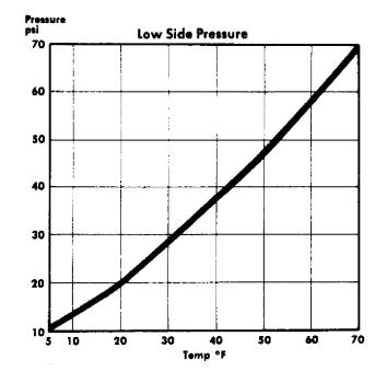
Fig. 2: Evaporator Temperature/Pressure (R-12)
