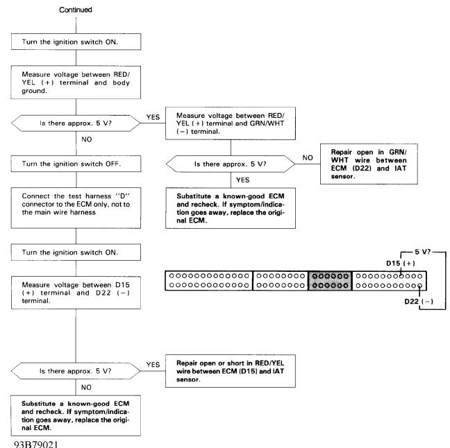
Fig. 21: Code 10 Flowchart, Intake Air Temperature Sensor (2 of 2) Courtesy of American Honda Motor Co., Inc.
