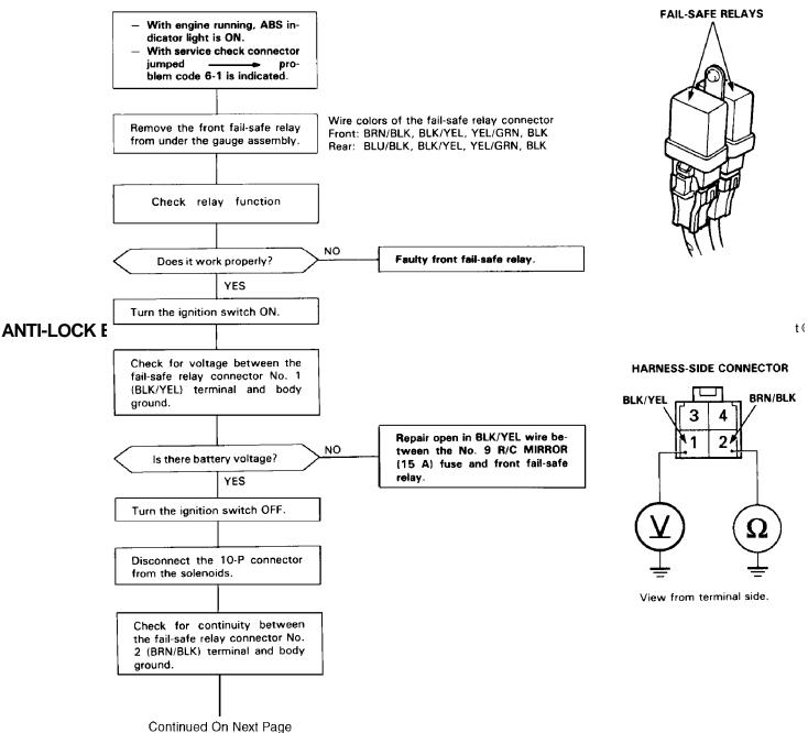
Fig. 23: Code 6-1 Flow Chart (1 Of 3), Front Fail-safe Relay Circuit Courtesy of American Honda Motor Co., Inc.
