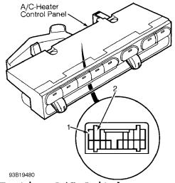
Fig. 9: Testing A/C Switch Courtesy of American Honda Motor Co. A/C-HEATER SYSTEM - MANUAL Article Text (p. 14)1993 Honda PreludeFor Cadi Centre Nsk CA 95051<sup>Cop</sup>
