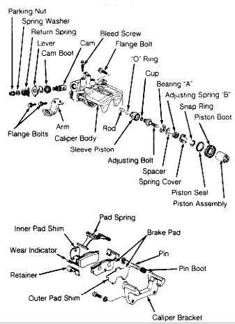
Fig. 6: Exploded View Of Rear Disc Brake Caliper (Typical) Courtesy of American Honda Motor Co., Inc.
