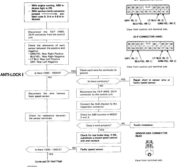
Fig. 21: Code 5 To 5-8 Flow Chart (1 Of 2), Speed Sensor(s) Courtesy of American Honda Motor Co., Inc.
