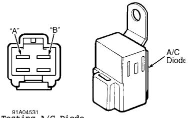
Fig. 8: Testing A/C Diode Courtesy of American Honda Motor Co.
