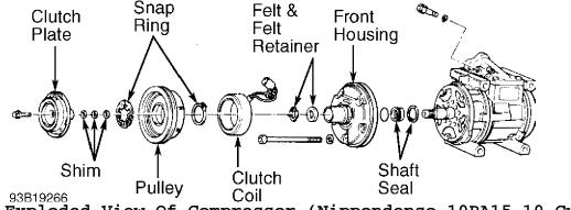
Fig. 14: Exploded View Of Compressor (Nippondenso 10PA15 10-Cylinder) Courtesy of Chrysler Corp.
