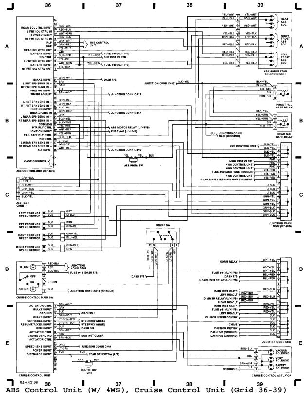
Fig. 10: ABS Control Unit (W/ 4WS), Cruise Control Unit (Grid 36-39) WIRING DIAGRAMS Article Text (p. 13)1993 Honda PreludeFor Cadi Centre Nsk CA 95051Copyright © 1998 Mitche
