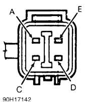
Fig. 6: Heated O2 Sensor Term. ID (Civic D15B7 & D16Z6, Civic Del Sol, & Prelude) Courtesy of American Honda Motor Co., Inc.
