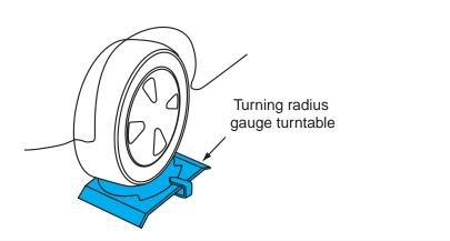
**Figure 13-25** All four wheels must be on radius gauge turntables with the wheels straight ahead and the turntables in the zero-degree position.
