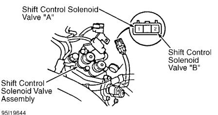
Fig. 26: Identifying Shift Control Solenoid Valve Terminals Courtesy of American Honda Motor Co., Inc.
