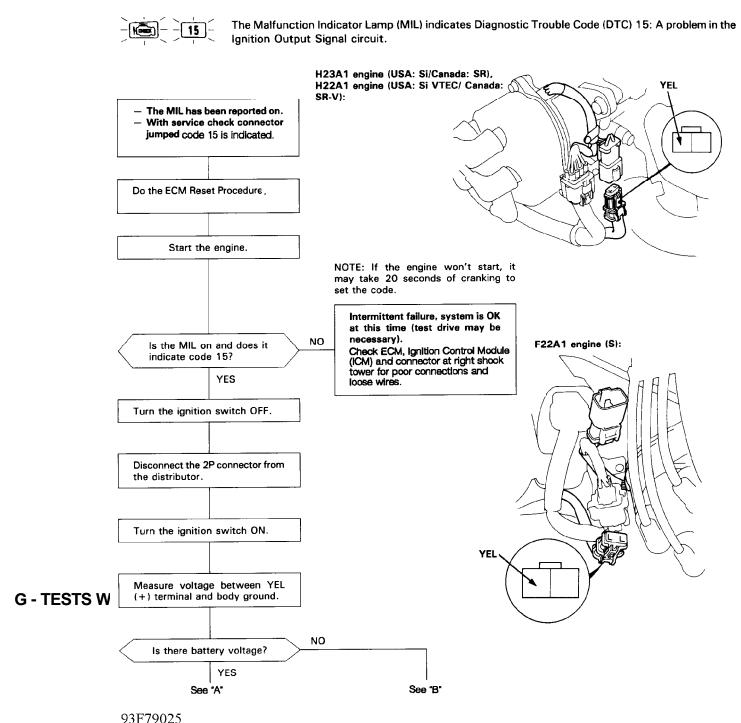
Fig. 30: Code 15 Flowchart, Ignition Output Signal (1 of 2) Courtesy of American Honda Motor Co., Inc.
