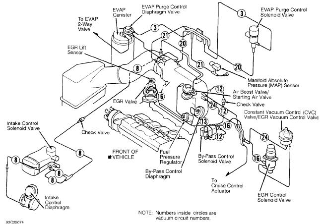
Fig. 15: Vacuum Diagram W/ Components (Prelude H22A1 & H23A1 Engines) Courtesy of American Honda Motor Co., Inc.
