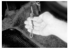
**P13-9** Remove the jumper wire from the service check connector.
