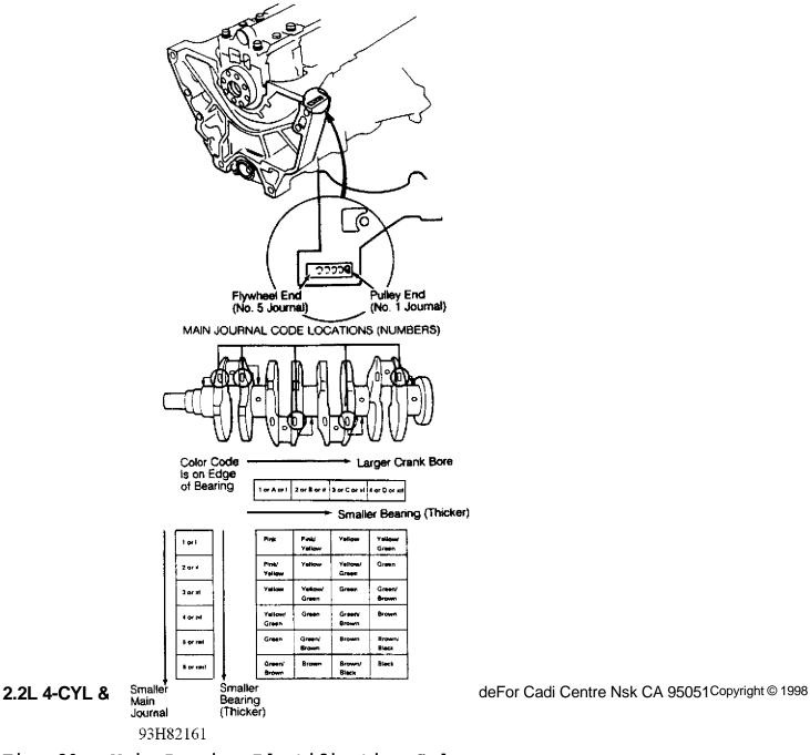
Fig. 20: Main Bearing Identification Codes Courtesy of American Honda Motor Co., Inc.
