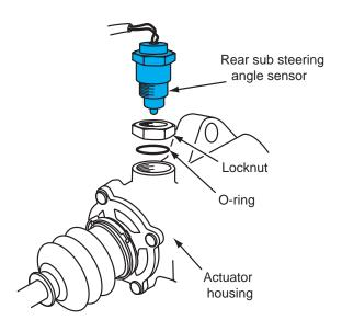
**Figure 13-20** Removing the rear sub steering angle sensor.
