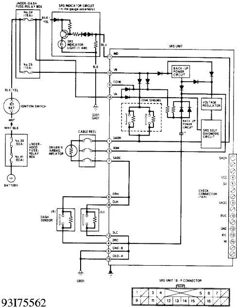
Fig. 29: SRS Wiring Diagram (Civic Without Passenger-Side Air Bag) Courtesy of American Honda Motor Co., Inc.
