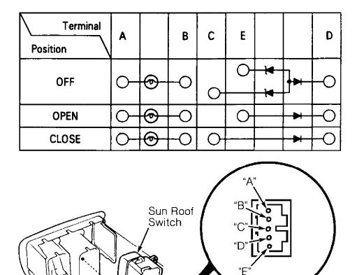
VAD 93F82581 Testing Sun Roof Switch Continuity (Prelude) Fig. 3: Courtesy of American Honda Motor Co., Inc.
