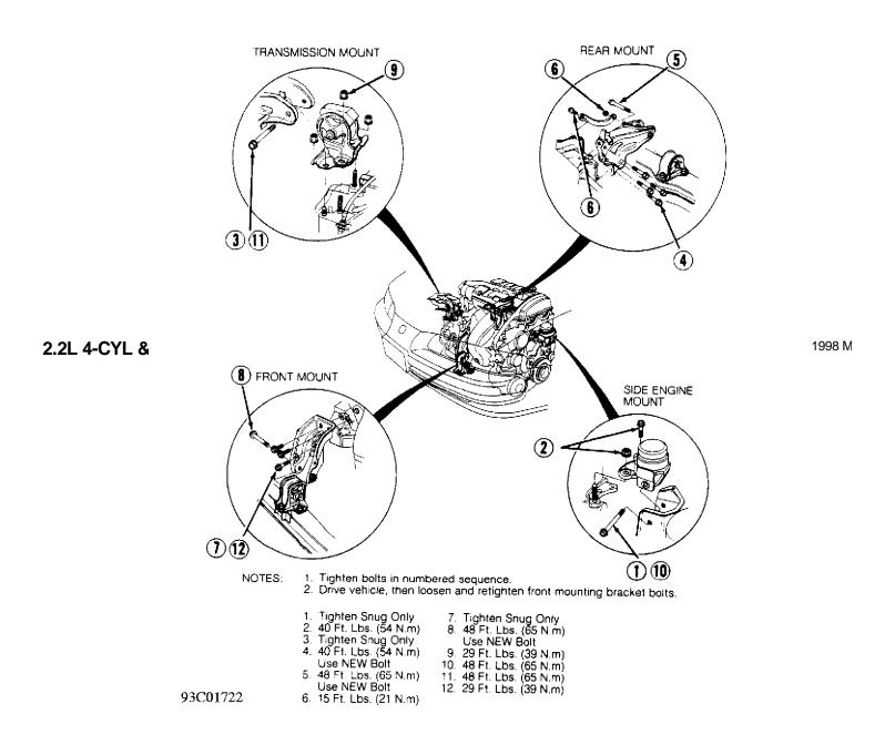
Fig. 5: Tightening Sequence For Engine/Transaxle Mounts Courtesy of American Honda Motor Co., Inc.
