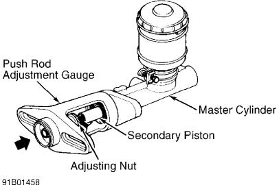
Fig. 1: Setting Push Rod Adjustment Gauge Courtesy of American Honda Motor Co., Inc.
