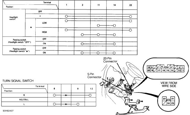
Fig. 2: Testing Headlight/Turn Signal Switch Courtesy of American Honda Motor Co., Inc.
