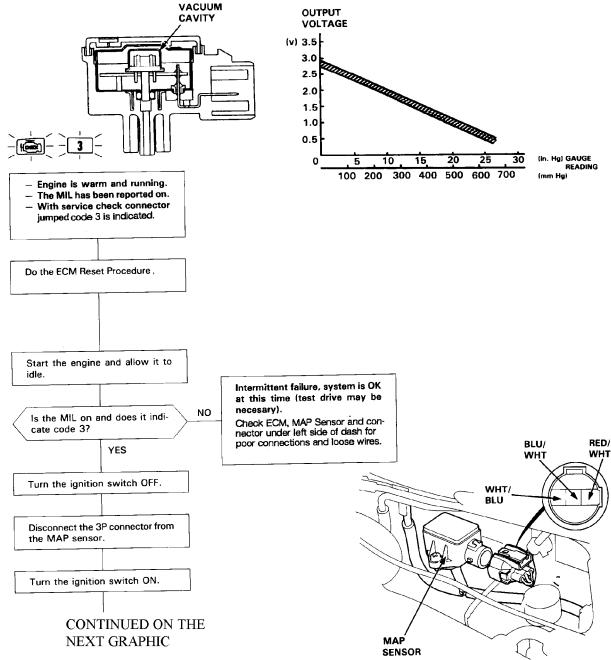
Fig. 9: Code 3 Flowchart, MAP Sensor Circuit (1 of 3) Courtesy of American Honda Motor Co., Inc.
