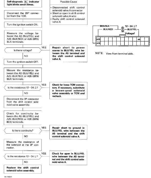
Fig. 43: Fault Code No. 7
