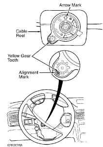
Fig. 3: Locating Cable Reel Alignment Marks (Typical) Courtesy of American Honda Motor Co., Inc.
