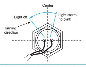
**Figure 13-36** Adjusting the rear sub steering angle sensor.
