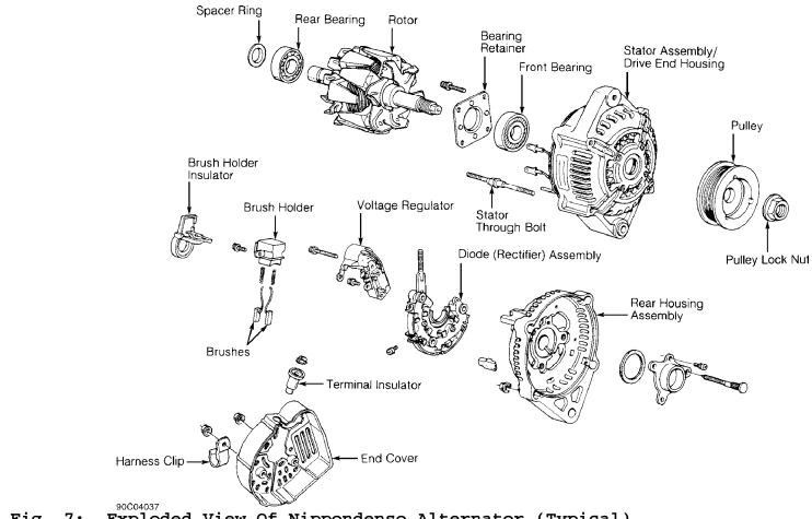
Use illustration for exploded view of alternator. SeeFig. 7.
