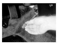
**P13-3** Lower the vehicle and locate the service check connector behind the center console.
