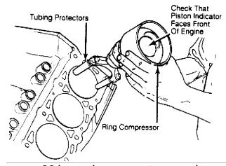
Fig. 17: Installing Piston & Connecting Rod Assembly - Typical This Graphic For General Information Only ENGINE OVERHAUL PROCEDURES - GENERAL INFORMATION Article Text (p. 21)1993 Honda Preluc Carefully tap piston into cylinder until rod bearing is seated on crankshaft journal. Remove protectors. Install rod cap and bearing. Lightly tighten connecting rod bolts. Repeat procedure for remaining cylinders. Check bearing clearance. See MAIN & CONNECTING ROD BEARING CLEARANCE in this article.
