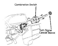
Fig. 9: Removing Turn Signal Cancel Sleeve & Combination Switch (Typical)
