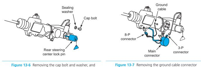
**Figure 13-7** Removing the ground cable connector and all wiring harness connectors on the rear steering actuator.
