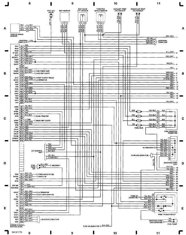
Fig. 3: Engine Control Module, Map Sensor (Grid 8-11) WIRING DIAGRAMS Article Text (p. 6) 1993 Honda PreludeFor Cadi Centre Nsk CA 95051<sup>Copyright © 1998 Mitchell</sup>
