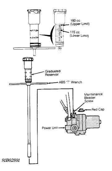
Fig. 2: Relieving Accumulator/Line Pressure (Typical) Courtesy of American Honda Motor Co., Inc.
