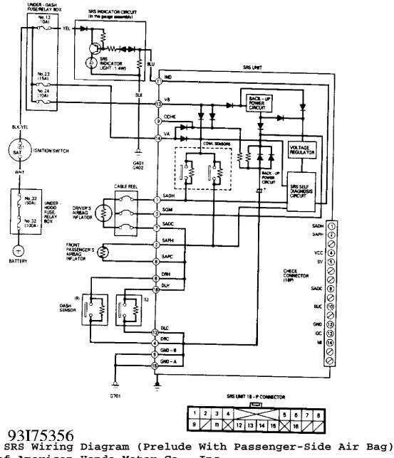
Fig. 31: SRS Wiring Diagram (Prelude With Passenger-Side Air Bag)
