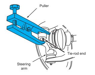
Figure 13-4 Removing a tie-rod end with a special tool.
