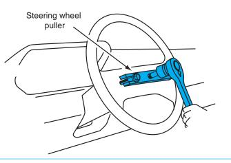
Figure 13-31 Removing the steering wheel.
