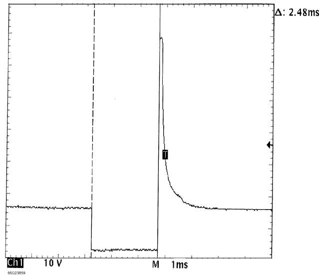
Fig. 21: Injector Bank - Known Good - Voltage Pattern
