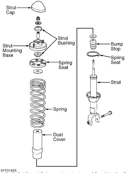
Fig. 3: Exploded View Of Rear Strut Assembly (Typical) Courtesy of American Honda Motor Co., Inc. SUSPENSION - REAR Article Text (p. 4)1993 Honda PreludeFor Cadi Centre Nsk CA 95051Copyright © 1998 Mitch
