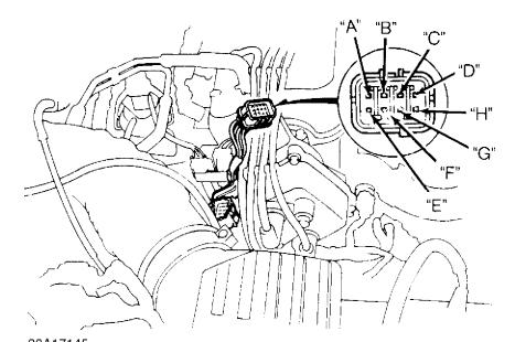
90A17145 Fig. 7: TDC/CKP/CYP Sensor Connector Term. ID (Accord Shown; Other Models Are Similar) Courtesy of American Honda Motor Co., Inc.
