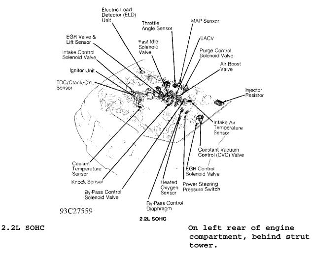
Electronic Air Control Valve (EACV)
