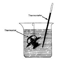
Fig. 1: Testing Thermostat in Anti-Freeze/Water Solution
