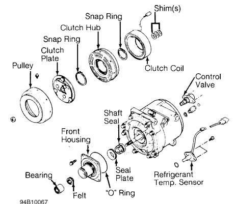
Fig. 17: Exploded View Of Compressor (Sanden FX105V Scroll) Courtesy of Chrysler Corp.
