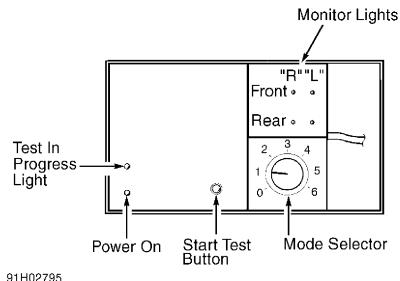
Fig. 3: Identifying ABS Tester Lights & Functions Courtesy of American Honda Motor Co., Inc.
