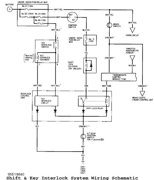
Fig. 20: Shift & Key Interlock System Wiring Schemati Courtesy of American Honda Motor Co., Inc.
