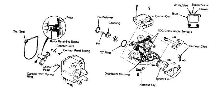
Fig. 2: Exp. View Of Dist. W/ Internal Ignitor (Civic & Civic Del Sol) Courtesy of American Honda Motor Co., Inc.
