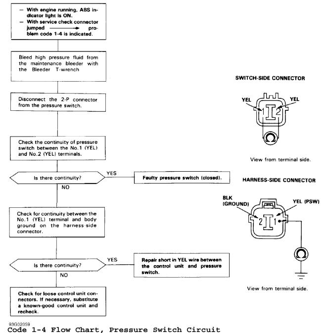
Fig. 16: Code 1-4 Flow Chart, Pressure Switch Courtesy of American Honda Motor Co., Inc.
