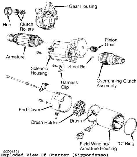
Fig. 8: Exploded View Of Starter (Nippondens Courtesy of American Honda Motor Co., Inc.
