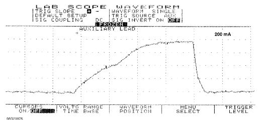
Fig. 10: Single Injector w/Normal Current Flow - Current Pattern WAVEFORMS - INJECTOR PATTERN TUTORIAL Article Text (p. 21)1993 Honda PreludeFor Cadi Centre
