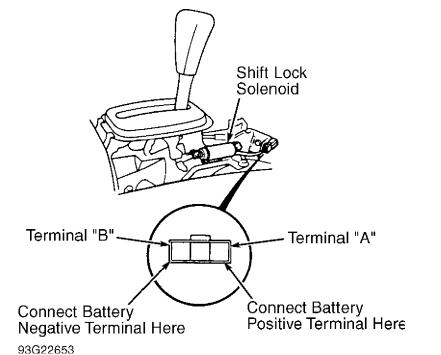
Fig. 27: Identifying Shift Lock Solenoid Connector & Terminals Courtesy of American Honda Motor Co., Inc.
