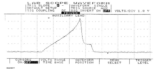
Fig. 16: Single Injector w/Excessive Current Flow - Current Pattern
