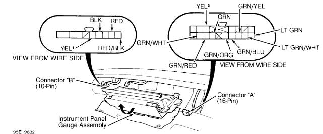
Fig. 12: Testing A/T Gear Position Indicator (1993, 1 of 2) Courtesy of American Honda Motor Contrained Diagnosis - MP1A Article Text (p. 17)1993
