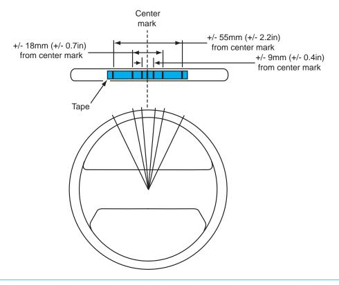
Figure 13-26 Steering wheel marking for electronically neutral check.
