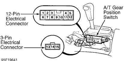
Identifying A/T Gear Position Switch Connector Terminals Fig. 21: Courtesy of American Honda Motor Co., Inc.
