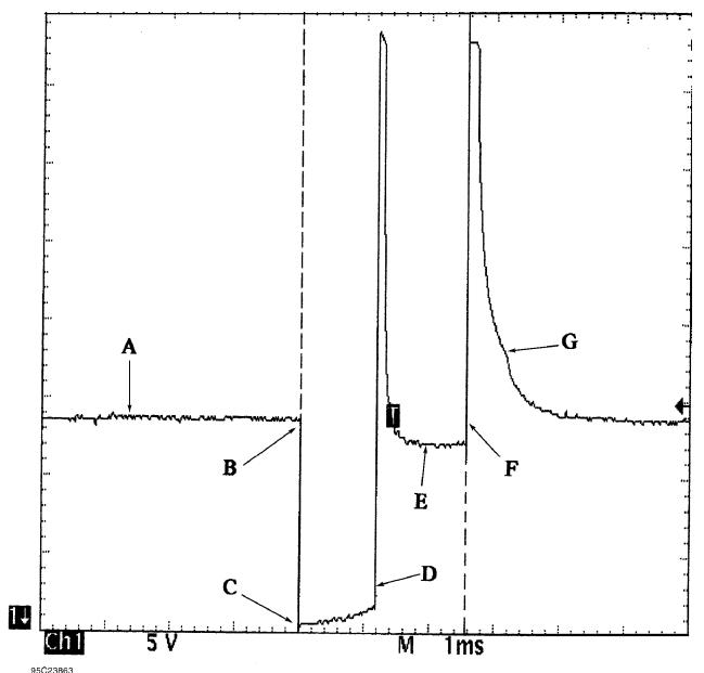
Fig. 3: Identifying Current Controlled Type Injector Pattern
