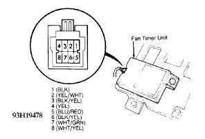
Fig. 6: Fan Timer Connector Terminal ID Courtesy of American Honda Motor Co.
