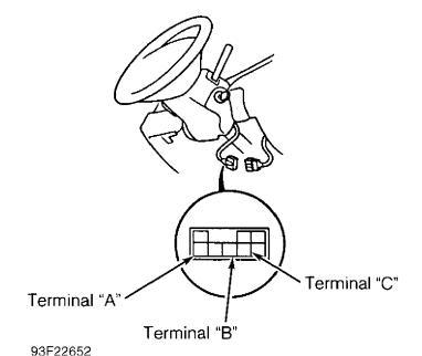
Fig. 24: Identifying Key Interlock Solenoid Connector & Terminals Courtesy of American Honda Motor Co., Inc.
