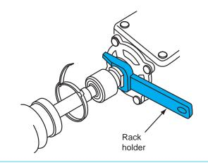
**Figure 13-16** Installing the special tool to hold the shaft screw while tightening the inner tie-rod end.
