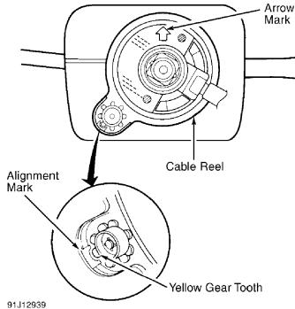
Fig. 13: Centering Cable Reel Courtesy of American Honda Motor Co., Inc. AIR BAG RESTRAINT SYSTEM Article Text (p. 15)1993 Honda PreludeFor Cadi Centre Nsk CA 95051<sup>Copyrig</sup>
