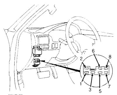
9017150 Fig. 10: Main Relay Harness Connector Term. ID (Accord Shown; Other Models Are Similar) Courtesy of American Honda Motor Co., Inc.
