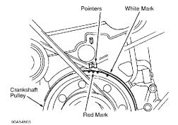
Fig. 5: Locating Ignition Timing Marks (Civic & Civic Del Sol) Courtesy of American Honda Motor Co., Inc. C-SPECIFICATIONS Article Text (p. 6)1993 Honda PreludeFor Cadi Centre Nsk CA 95051<sup>Copyright ©</sup> 1998 Mitche
