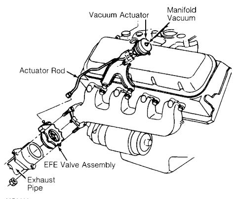
93B04145 Fig. 15: Typical Vacuum-Actuated EFE System Courtesy of General Motors Corp.
