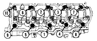
• FRONT OF VEHICLE Fig. 1: Typical Cylinder Head Tightening or Loosening Sequence This Graphic For General Information Only
