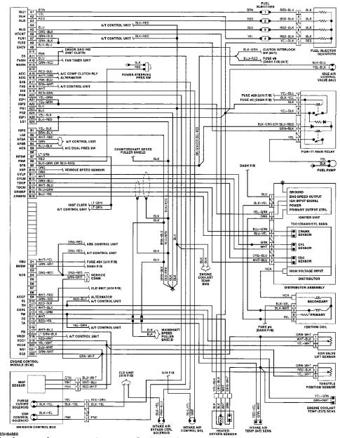
Fig. 1: Wiring Diagram (Accord 2.2L)
