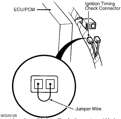
Fig. 7: Locating Ign. Timing Check Connector (Civic & Civic Del Sol) Courtesy of American Honda Motor Co., Inc.
