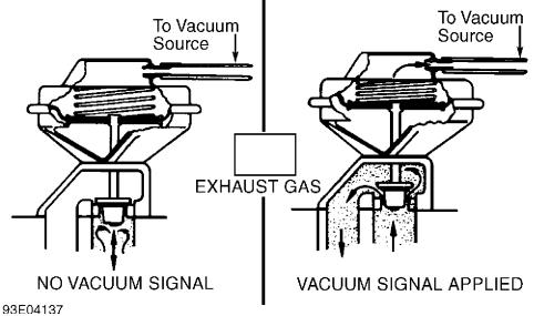
Fig. 7: Typical Single Diaphragm EGR Valve Courtesy of General Motors Corp.
