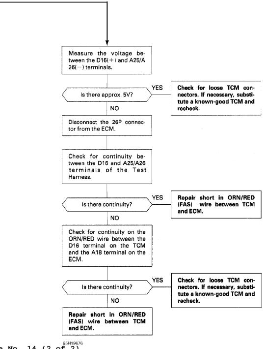
Fig. 50: Fault Code No. 14 (2 of 2)
