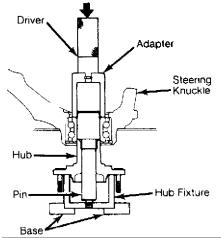
Fig. 5: Pressing Knuckle/Bearing Assembly Onto Hub Courtesy of American Honda Motor Co., Inc.
