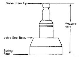
Fig. 11: Measuring Valve Stem Installed Height - Typical This Graphic For General Information Only
