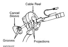
Fig. 12: Aligning Cable Reel & Cancel Sleeve (Typical) Courtesy of American Honda Motor Co., Inc.
