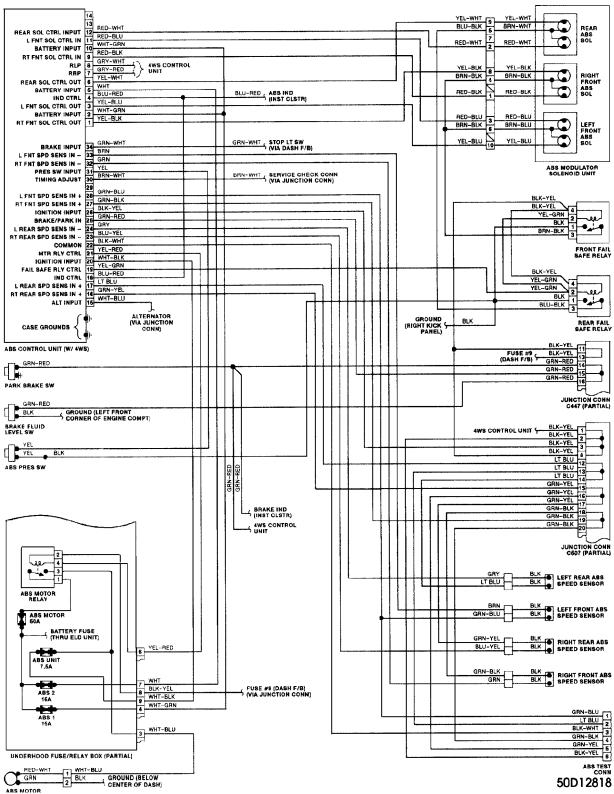
Fig. 35: Anti-Lock Brake System Wiring Diagram (Prelude 4WS) ANTI-LOCK BRAKE SYSTEM Article Text (p. 40)1993 Honda PreludeFor Cadi Centre Nsk CA 95051Copyright ( END OF ARTICLE
