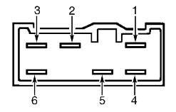
93B19431 Fig. 5: Fan Switch Connector Terminal ID Courtesy of American Honda Motor Co., Inc.
