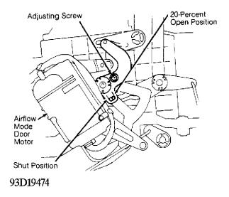
Fig. 2: Adjusting Defrost Bleed Courtesy of American Honda Motor Co. A/C-HEATER SYSTEM - MANUAL Article Text (p. 4)1993 Honda PreludeFor Cadi Centre Nsk CA 95051<sup>Copyr</sup>
