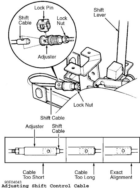
Fig. 1: Adjusting Shift Control Cable Courtesy of American Honda Motor Co., Inc.
