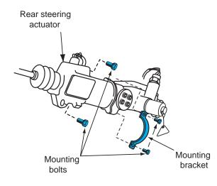
**Figure 13-8** Removing the four mounting bolts, bracket, and rear steering actuator.
