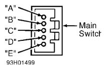
Fig. 8: Main Switch Terminal ID Courtesy of American Honda Motor Co., Inc.
