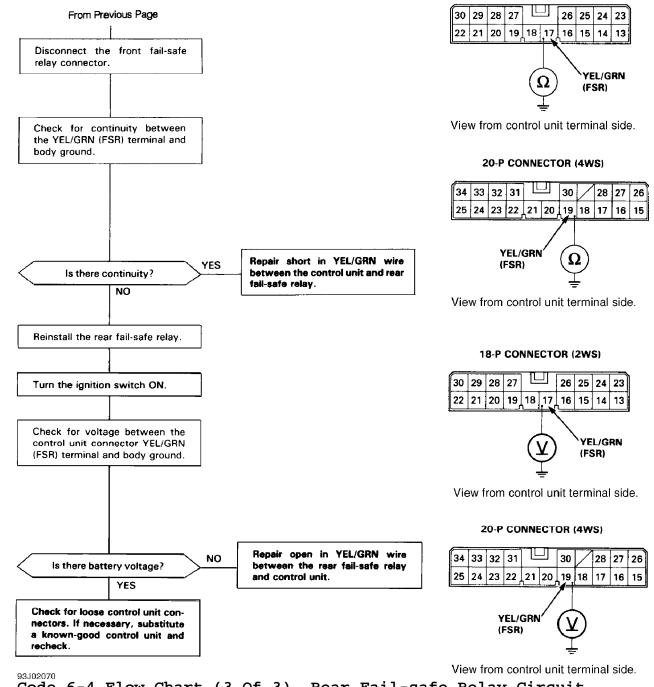
Fig. 28: Code 6-4 Flow Chart (3 Of 3), Rear Fail-safe Relay Circuit ANTI-LOCK BRANE SYSTEM Anticle Poxt (pc3) 1933 donda Prelude For Cadi Centre Nsk CA 95051 Copyright (
