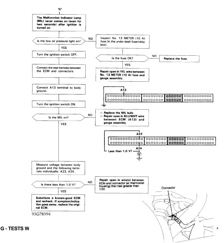
Fig. 4: Flowchart, No Start Trouble Shooting (2 of 5) Courtesy of American Honda Motor Co., Inc.
