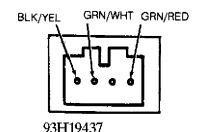
Fig. 9: Recirculation Control Motor Connector Terminal ID Courtesy of American Honda Motor Co., Inc.
