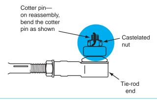
**Figure 13-23** Proper installation of cotter pin in the tie-rod end.
