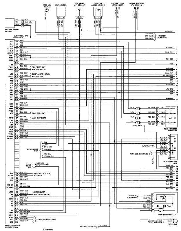
Fig. 6: Wiring Diagram (Prelude 2.2L & 2.3L - 1 Of 2) L-WIRING DIAGRAMS Article Text (p. 6)1993 Honda PreludeFor Cadi Centre Nsk CA 95051Copyright © 1998 Mit
