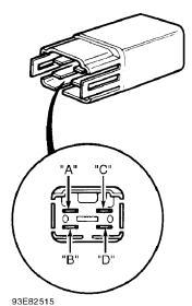
Fig. 5: Power Window Relay Terminal ID Courtesy of American Honda Motor Co., Inc.
