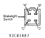
Fig. 4: Identifying Brakelight Switch Connector Courtesy of American Honda Motor Co., Inc.
