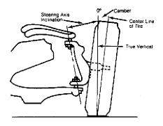
Fig. 6: Checking Steering Axis Inclination
