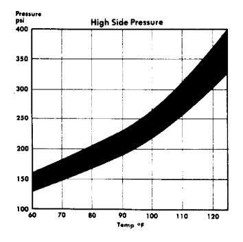
Fig. 1: Ambient Temperature/Pressure (R-12)
