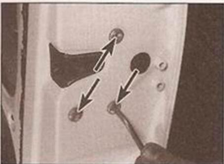
13.16a Unscrew the lock retaining bolts . . .
