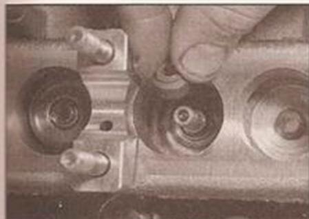
4.60a Fit a new valve stem seal over the valve
