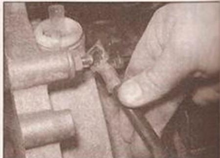
**3.8b . . . and disconnect the transmission earth strap**
