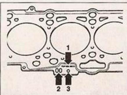
11.30 Cylinder head gasket identification markings
