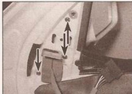
19.5b Remove the three mounting screws (arrowed) . . .
