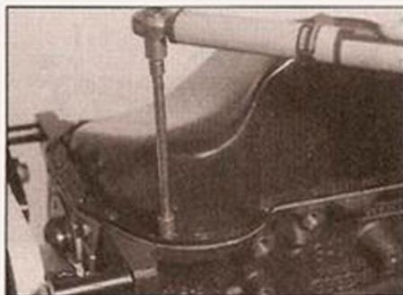
14.8 Removing the sump bolts (seen with engine removed and inverted, for clarity)
