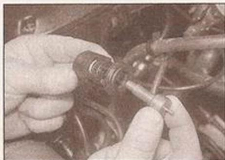
4.6b The thermostat can be separated from its spring housing
