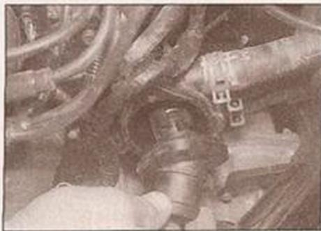
4.5b . . . and carefully remove the thermostat cover
