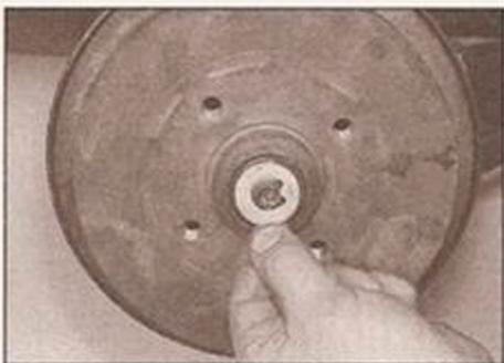
7.4a ... then unscrew the retaining nut and remove the toothed washer
