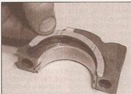
**11.16** Fitting the thrustwashers to No 3 bearing cap
