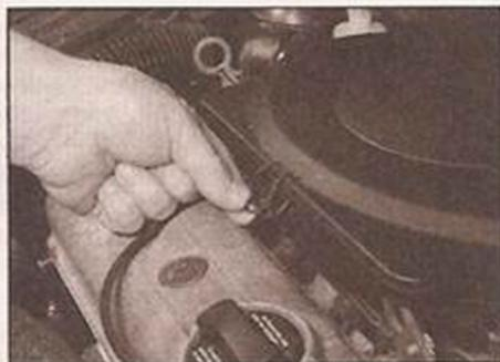
26.1a Release the air filter cover clips . . .
