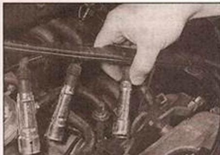
21.5 Pull the HT lead end fittings off the plugs
