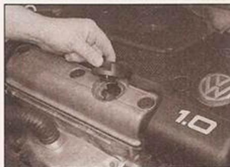
3.12a Remove the oil filler cap ...
