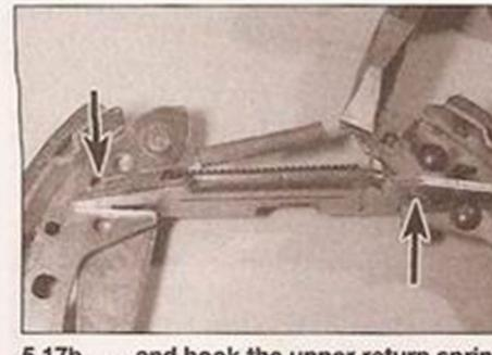
5.17b . . . and hook the upper return spring into the leading shoe and pushrod (arrowed)
