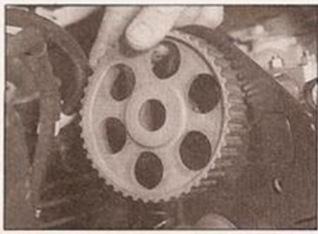
5.13 Removing the camshaft sprocket
