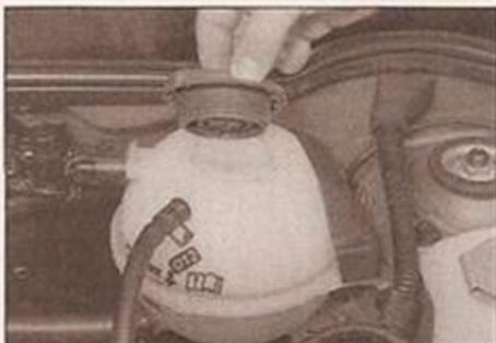
**2** If topping up is necessary, wait until the engine is cold. Slowly unscrew the expansion tank cap, to release any pressure present in the cooling system, and remove it.
