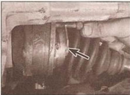
**2.7c . . . and recover the retaining plates**
