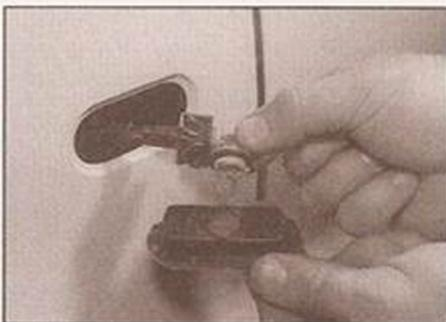
7.21 Remove the bulbholder from the rear of the light unit
