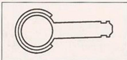
17.1 Radio/cassette removal tool 3316 - for lower-specification sets
