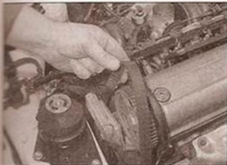
4.16 Removing the timing belt
