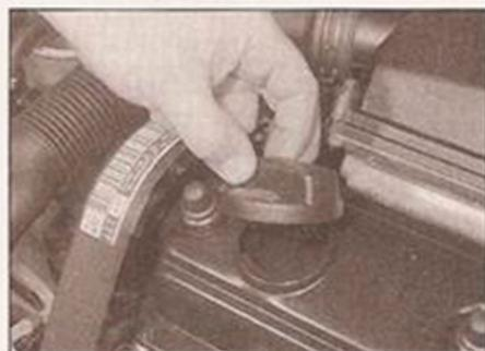
3.12a Remove the oil filler cap . . .
