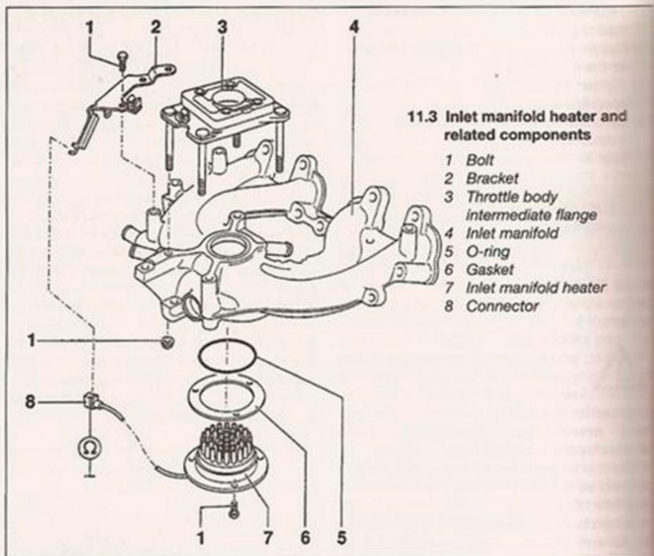
11.3 Inlet manifold heater and related components
