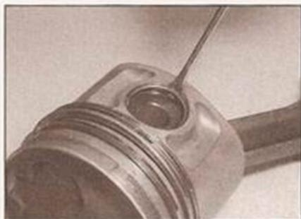
5.12a Insert a small screwdriver into the slot and prise off the gudgeon pin circlips
