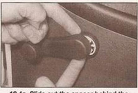
12.4a Slide out the spacer behind the regulator handle (the direction will not necessarily be as shown) . . .
