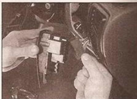
6.7b Disconnecting the lighting switch wiring plug
