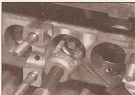
4.62b Use grease to hold the two halves of the split collet in the groove
