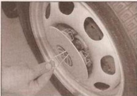
**2** Remove the wheel trim/hub cap (on some models, a wire hook is provided, which is inserted through one of the holes in the wheel trim, and used with the wheelbrace handle to pull off the trim). On lower-specification models, plastic caps may be fitted over the wheel bolts, which can be hooked off with the tool provided.
