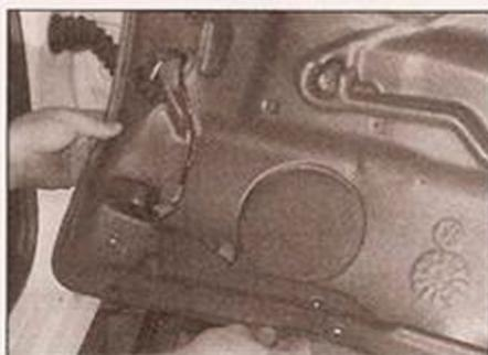
14.4b Removing the foam panel
