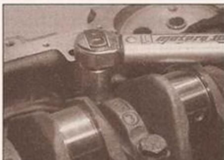
**11.19** Tighten the bearing cap bolts to the specified torque
