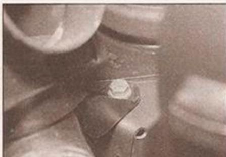
2.9b Air temperature control valve housing mounting bolt on inner wing
