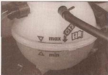
**1** The coolant level varies with engine temperature. When cold, the coolant level should be between the "MAX" and "MIN" marks. When the engine is hot, the level may rise slightly above the "MAX" mark.
