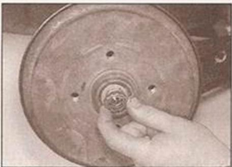
7.3 Remove the split pin and locking cap ...
