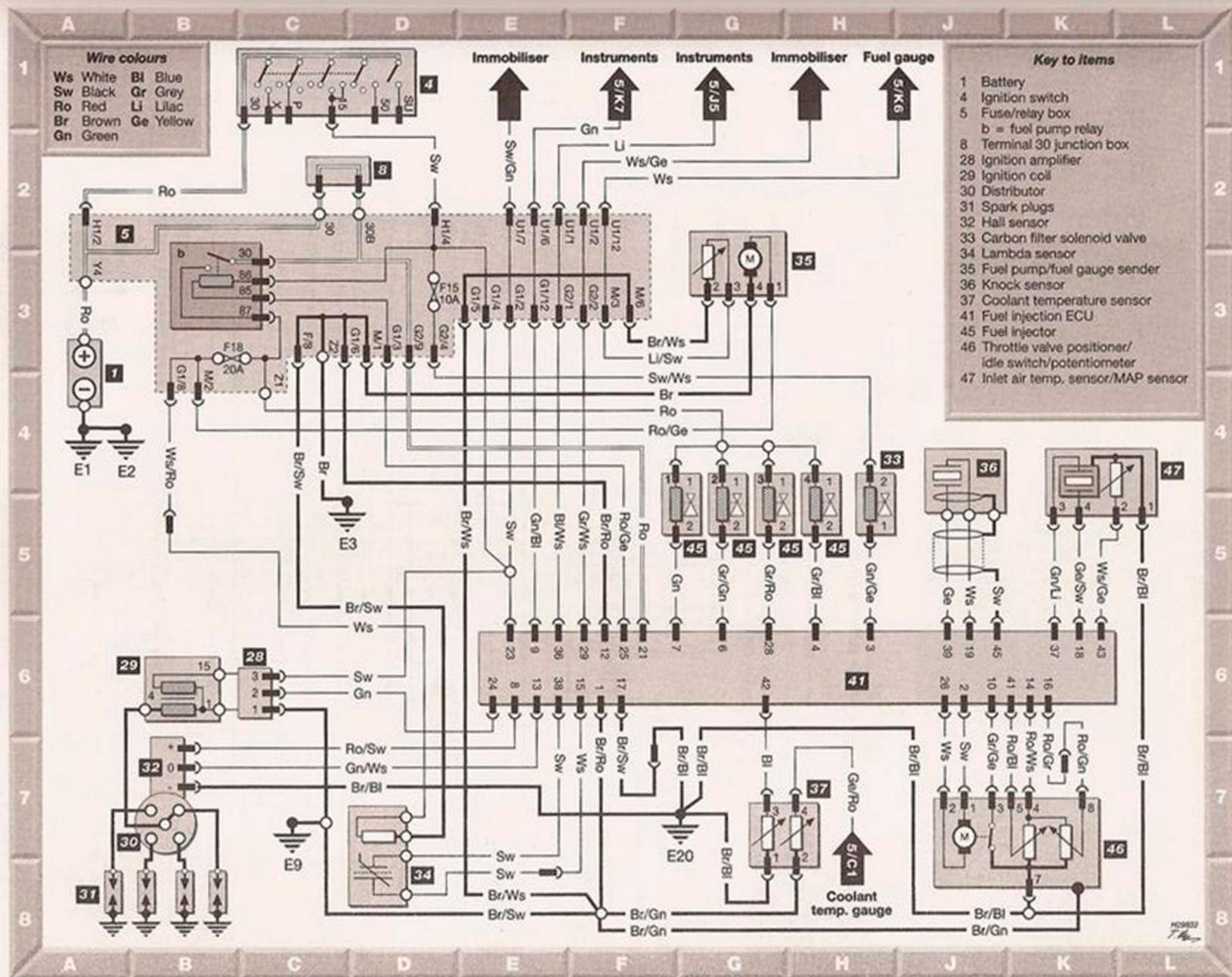
Diagram 4 : Motronic engine management - models up to 1998
