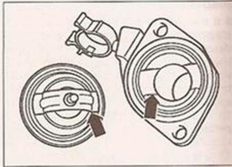
4.14 Thermostat installation details - engine codes ADX, AEA and AEV
