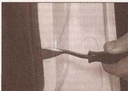
12.9a Lever between the door trim panel and the door to release the trim panel studs ...
