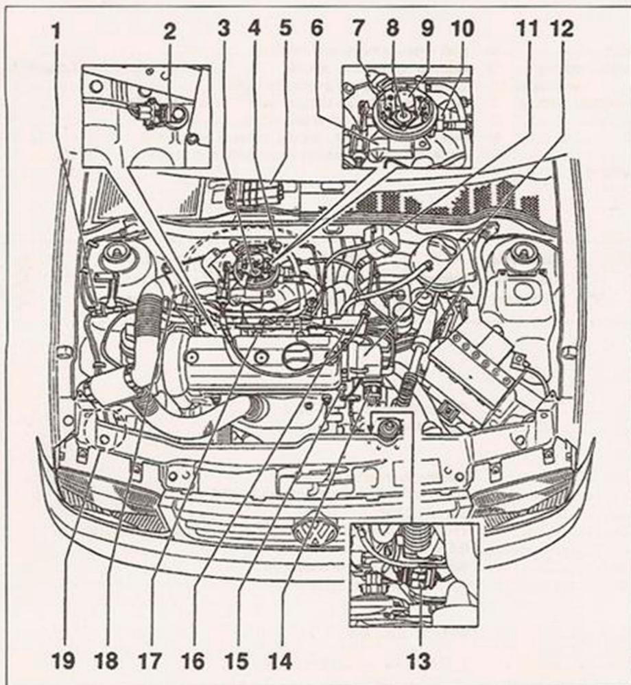
1.1 Bosch Mono-Motronic engine management system component locations
