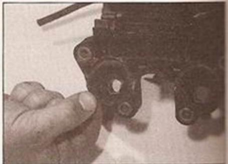
10.9 When refitting the inlet manifold, use new O-ring seals
