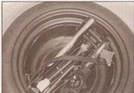
**1** The spare wheel and tools are stored in the luggage compartment, under the floor covering. A warning triangle may be provided on the right-hand side of the luggage compartment, behind a trim panel. Release the retaining strap, and lift out the jack and wheel changing tools from the centre of the wheel. Unscrew the retaining nut and lift the wheel out of the vehicle.
