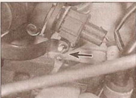
11.14 Unbolt the electrical supply cable from No 4 cylinder glow plug
