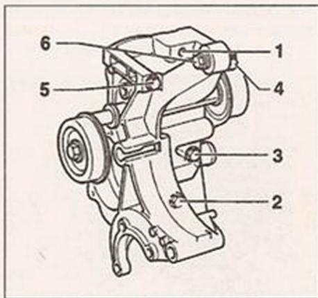
7.19 Coolant pump mounting bracket bolt tightening sequence
