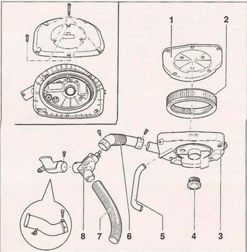
2.8c Air cleaner housing and inlet system components
