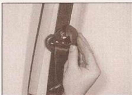
25.1 Unclip the cover from the seat belt upper mounting ...
