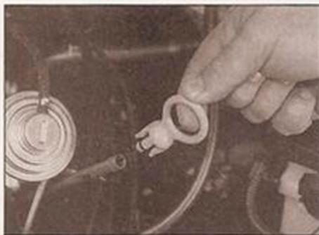
**1** The dipstick top is often brightly coloured for easy identification (see *Underbonnet check points* on pages 0•10 for exact location). Withdraw the dipstick.
