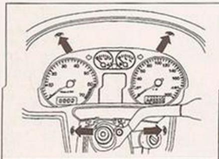
10.8 Instrument panel surround screws (arrowed) - 1998-on models
