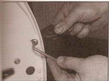
**13.4a** Remove the handle securing screw using a Torx key or socket ...
