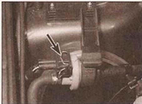
2.3 Charcoal canister purge valve wiring connector (arrowed)
