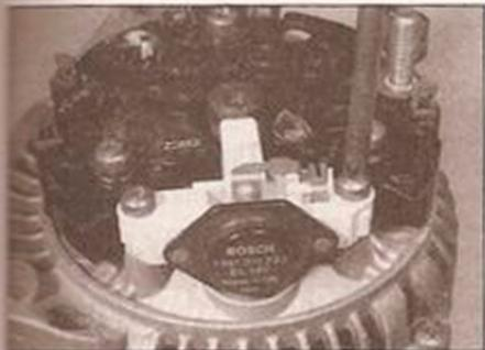
6.4a Remove the brush holder/voltage regulator module screws . . .
