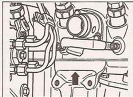
Engine number location (arrowed) - diesel models
