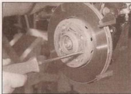
6.8a Remove the disc securing screw ...
