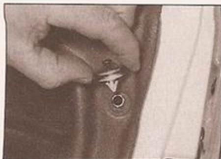
13.12 Prise out the door inner trim panel retaining studs
