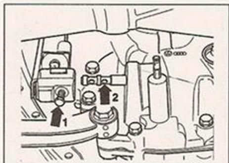
**3.27 Selector finger securing bolt (1) fits into forward recess in inner finger (2) when assembled - rod-type gear linkage**
