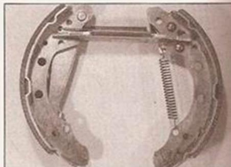
5.10 Prior to dismantling, note the correct fitted location of the shoe components
