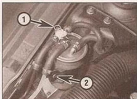
5.3 Fuel filter R-clip (1) and retaining bracket screw (2)
