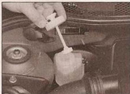
3 Unscrew the reservoir cap and carefully lift it out of position, taking care not to damage the level switch float. Place the cap and float on a piece of clean rag. Inspect the reservoir; if the fluid is dirty, the hydraulic system should be drained and refilled (see Chapter 1).
