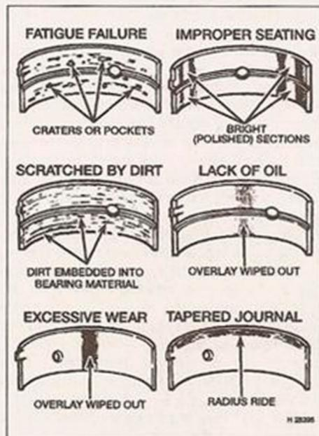
9.1 Typical bearing failures
