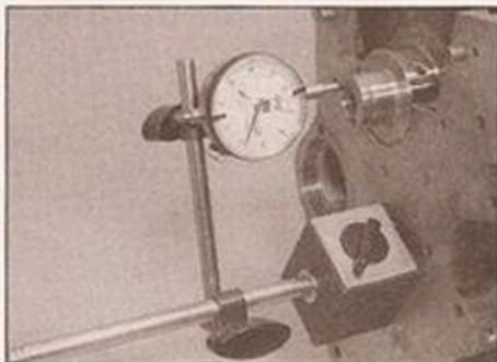
6.4 Measuring crankshaft endfloat using a DTI gauge
