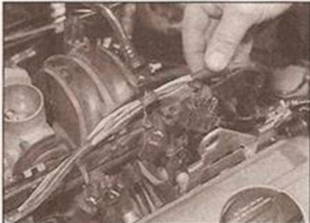
5.10b ... then unclip the harness retaining clips, and move the wiring harness to one side
