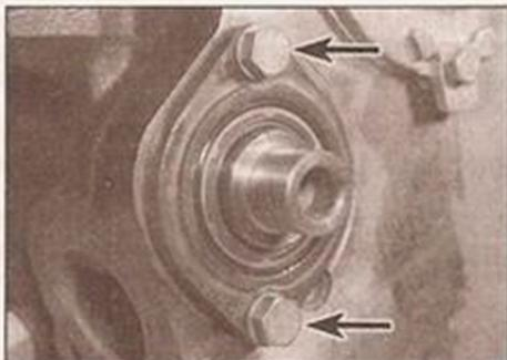
7.3a Slacken the retaining bolts (arrowed) . . .
