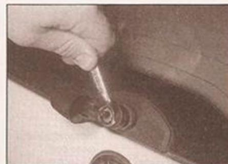
15.3b ... then remove the wiper arm nut ...
