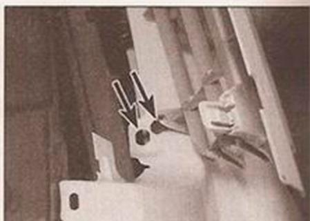
29.2c ... then lift the grille pegs out of the holes (arrowed) ...
