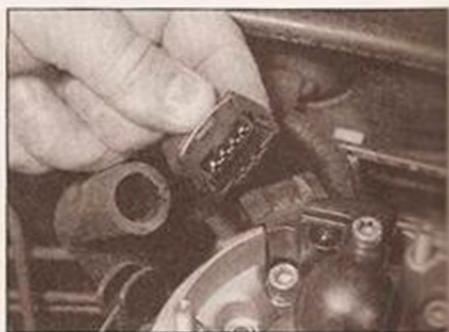
5.4 Disconnecting the fuel injector wiring plug
