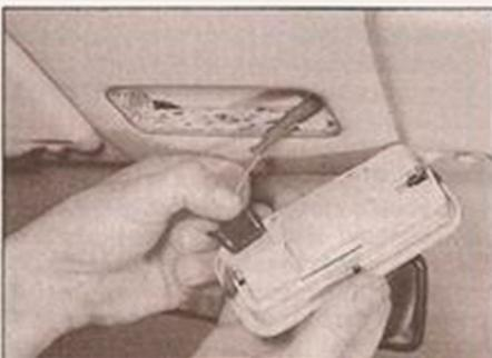
8.2b ... and disconnect the wiring plug, if required
