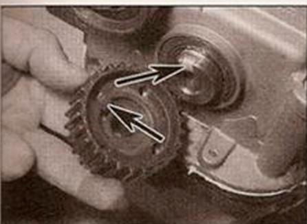
5.28 Crankshaft sprocket alignment tooth and keyway (arrowed)
