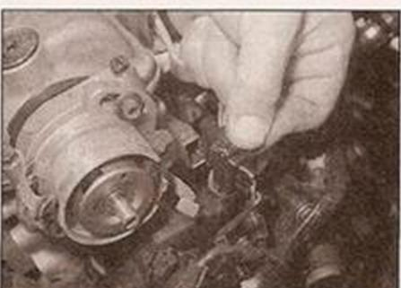
10.8e . . . distributor Hall sensor wiring plug . . .
