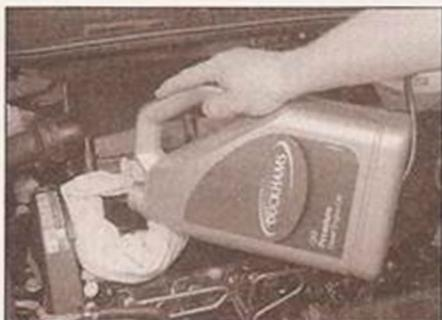
3.12b . . . and fill the engine with the recommended type and quantity of oil
