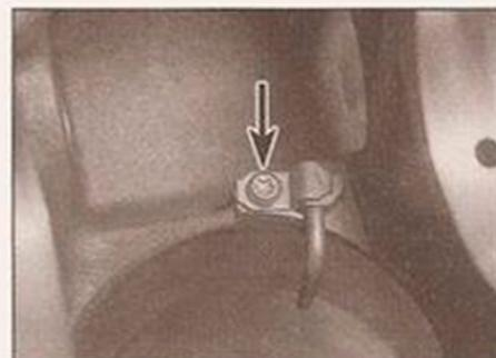
5.5a Remove the piston cooling jet retaining screw (arrowed) . . .
