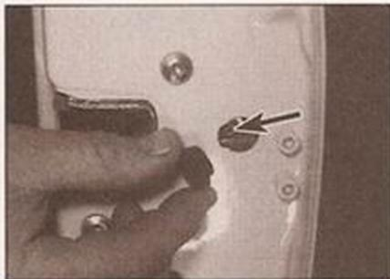
13.30 Door lock adjustment screw (arrowed)
