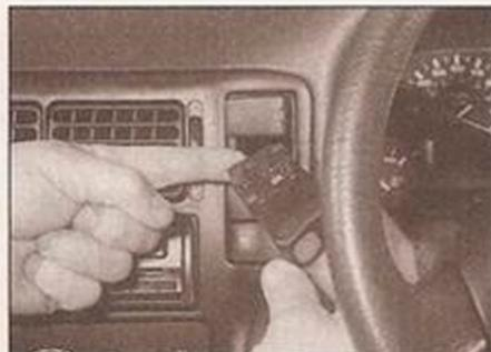
6.3 ... and disconnect the wiring plug
