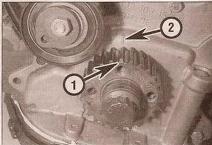
2.25 Crankshaft sprocket chamfered tooth (1) and timing mark (2)
