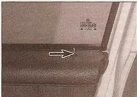
12.9b . . . lift the panel over the door lock operating knob (arrowed) . . .
