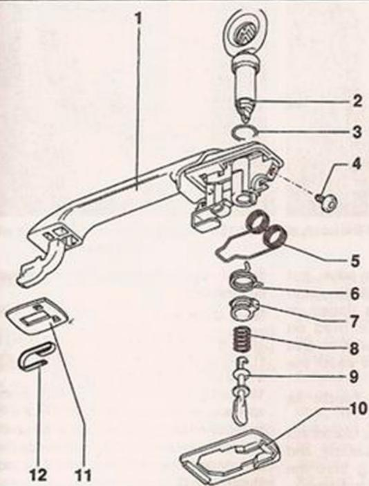
**13.1a Front door handle and lock components - models up to July 1997**
