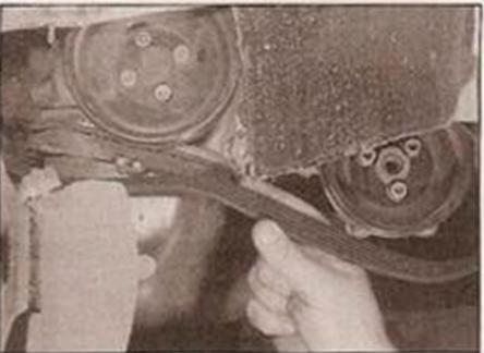
6.11 Removing the auxiliary drivebelt
