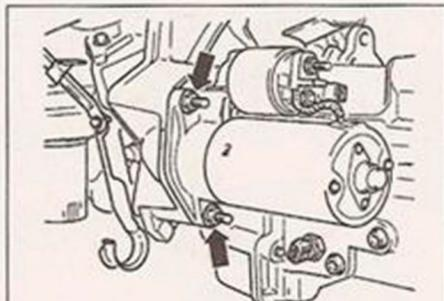
8.8 Starter motor through-bolts (arrowed) - diesel engine models
