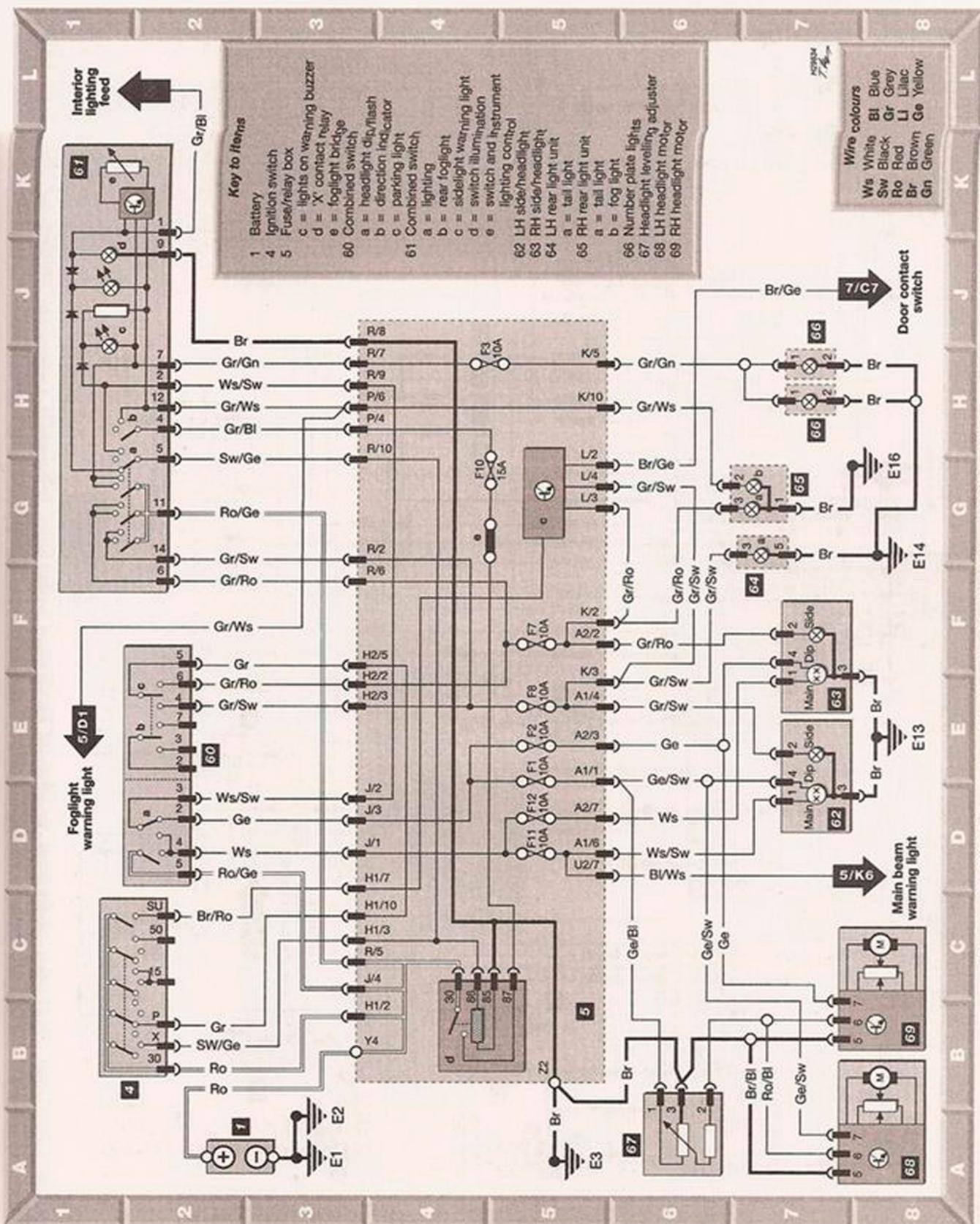
Diagram 6 : Side, tail, number plate, head and foglights, headlight levelling - models up to 1998
