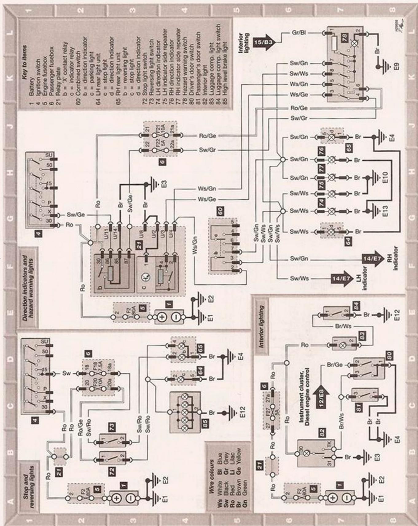
Diagram 16 : Stop, reversing, direction indicators/hazard warning lights and interior lighting - models from 1998
