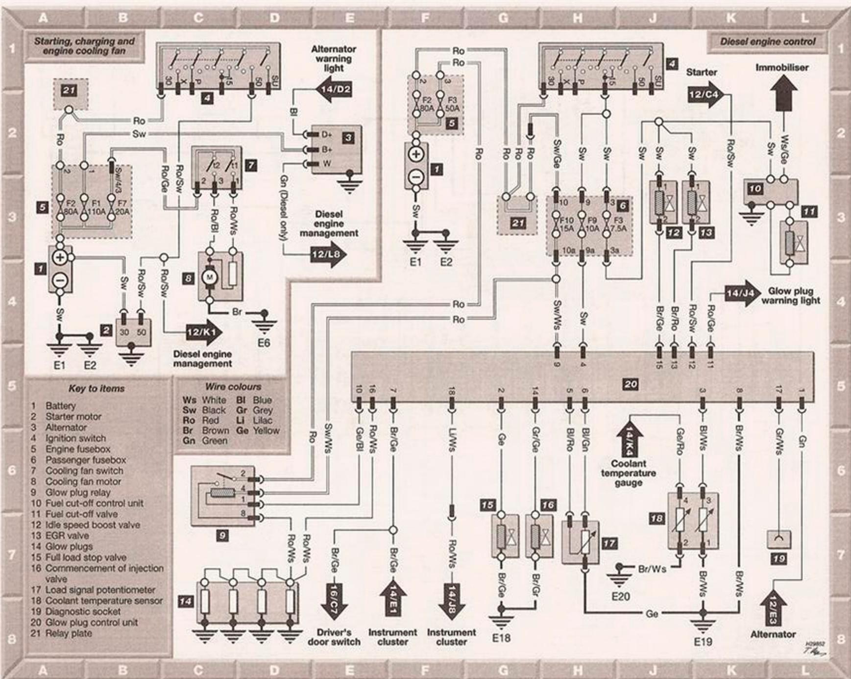
Diagram 12 : Starting and charging systems, engine cooling fan and Diesel engine control - models from 1998
