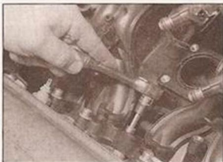
10.7a Unscrew the inlet manifold bolts . . .
