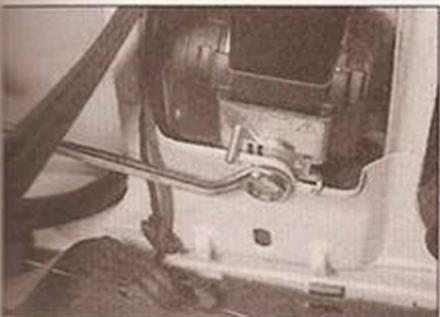
25.14b . . . and the inertia reel mounting bolt
