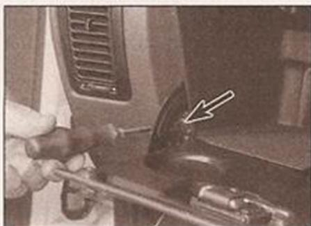
26.10a Remove the screw behind each hinge . . .
