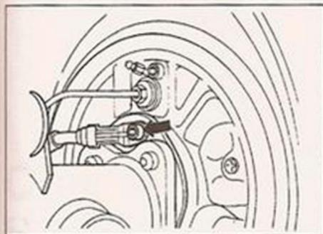
20.12 ABS rear wheel sensor retaining bolt (arrowed)
