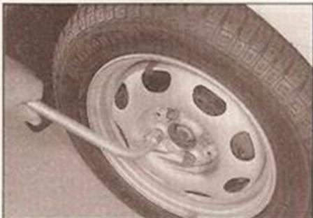
**3** Slacken each wheel bolt by a half turn, using the wheelbrace. If the bolts are too tight, DON'T stand on the wheelbrace to undo them - call for assistance from one of the motoring organisations.
