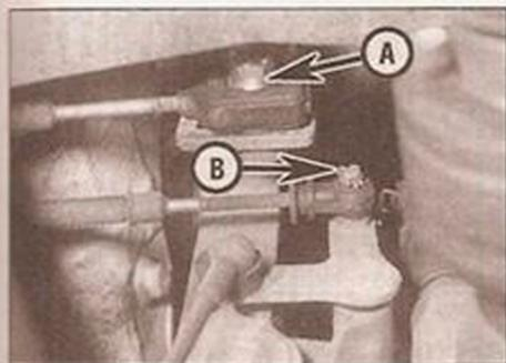
3.13a Gear selector cable through-bolt (A) and gate selector cable spring clip (B)
