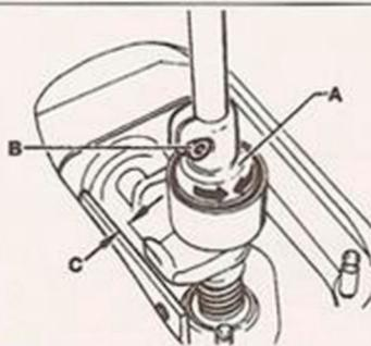
**2.4 Gearchange lever adjustment collar - models with rod-type linkage**
