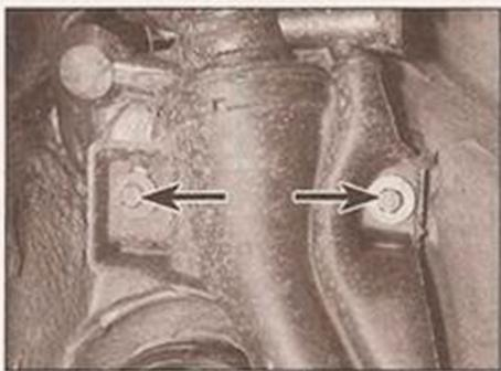
5.7 Fuel filler neck securing bolts (arrowed) - seen from inside the wheel arch
