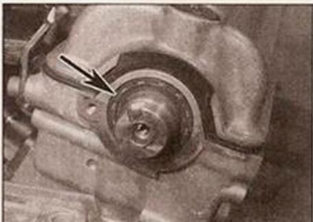
**8.3c Camshaft oil seal (arrowed)**
