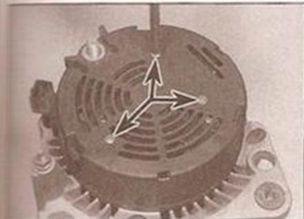
6.3a Where applicable, remove the retaining screws (arrowed) . . .
