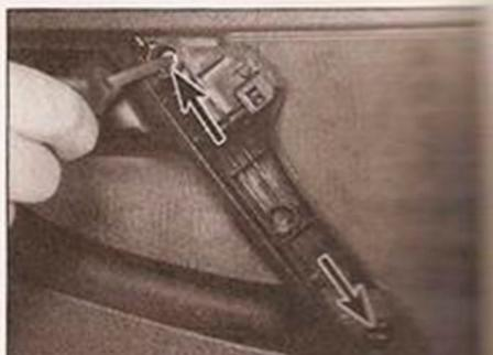
12.8 Door handle surround securing screws (arrowed)
