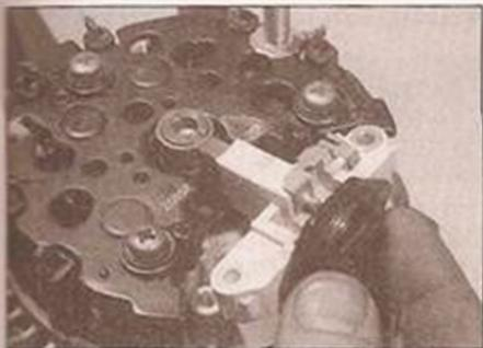
6.4b . . . then lift the module away from the alternator
