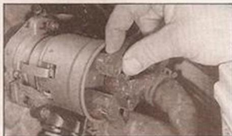
**B** Check that the HT leads are securely connected to the distributor cap (petrol engine models).
