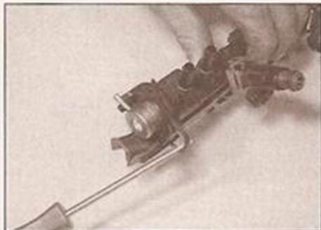
5.23b To remove the pressure regulator, prise out the retaining clip and withdraw it from the fuel rail
