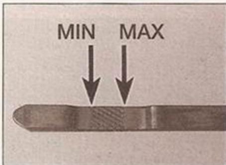
**3** Note the oil level on the end of the dipstick, which should be within the hatched area marked. If the oil level is at the bottom of, or below, the hatched area, topping-up is required.
