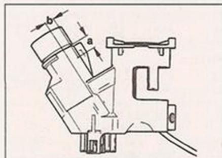
4.10b Drilling point for removing ignition lock cylinder - models with immobiliser reader coil integral with ignition switch
