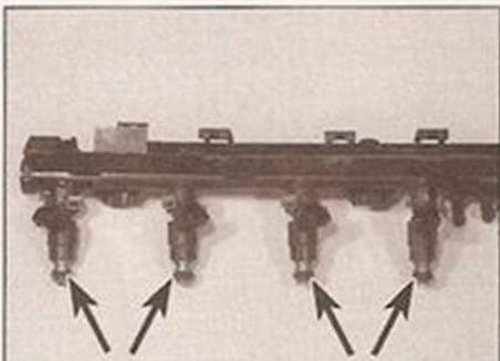
5.14b ... and recover the injector lower O-ring seals (arrowed)
