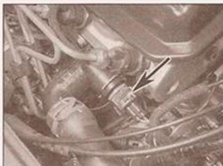
6.15a Coolant temperature sender wiring plug (arrowed)
