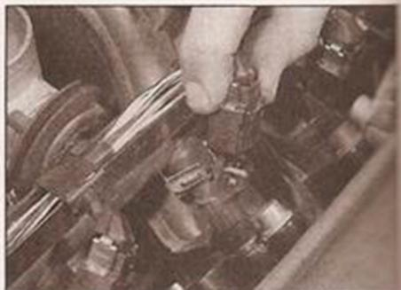
5.10a Disconnect the injector wiring plugs ...
