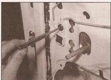
13.18a Using a pin punch, press through the spreader pin . . .
