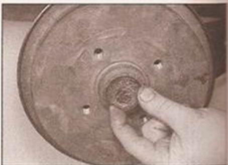
7.4b Withdraw the outer bearing ...
