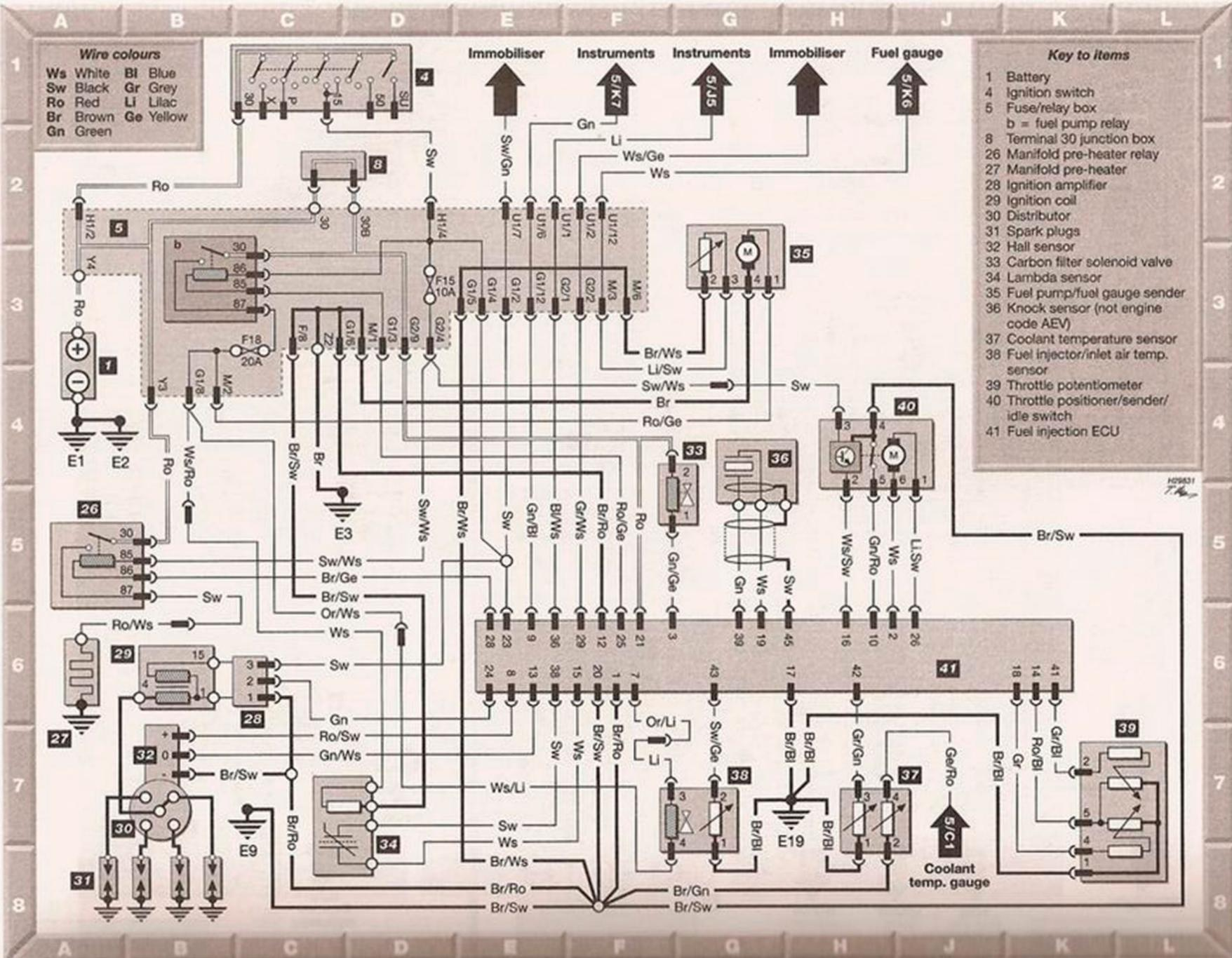
Diagram 3: Mono-motronic engine management - models up to 1998
