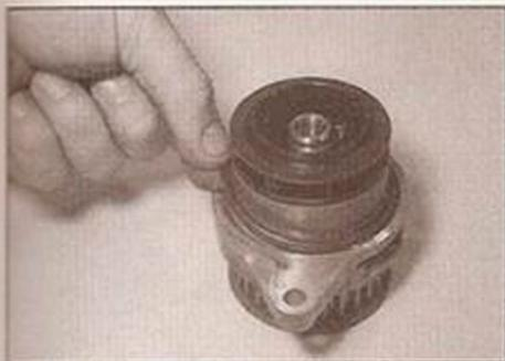
7.13 Fit a new O-ring to the coolant pump
