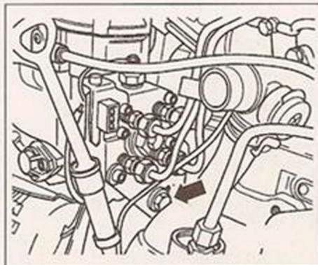
6.20b ... and rear support bolt (arrowed) - engine codes AKU, AHG and AGD
