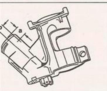
4.7a Drilling point for removing ignition lock cylinder - models with immobiliser reader coil separate from ignition switch
