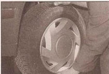
17.4 Check for wear in the hub bearings by grasping the wheel and trying to rock it
