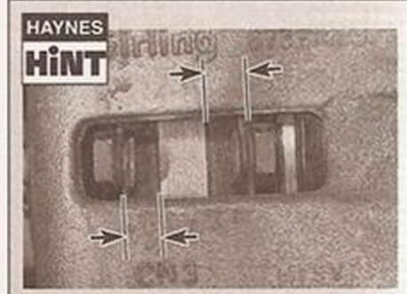
For a quick check, the thickness of the friction material on each brake pad can be measured through the aperture in the caliper body
