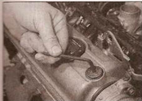
**7.3 Loosen and remove the socket-headed retaining bolts ...**
