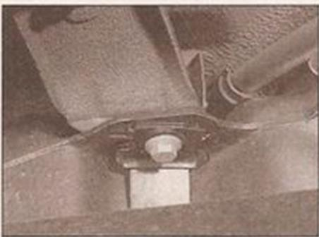
5.9 Fuel tank strap securing bolt
