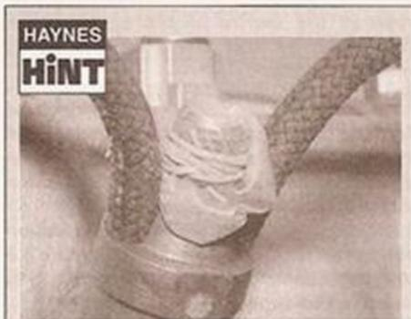
**Haynes Hint 1:** Cut the fingertips from an old pair of rubber gloves and secure them over the fuel ports with elastic bands
