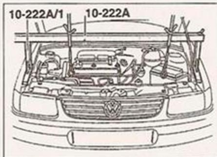
2.19 Engine/transmission support bar used by VW mechanics
