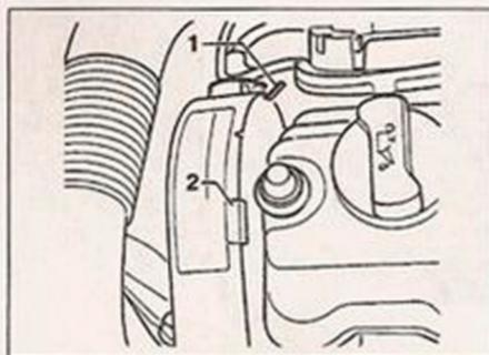
26.7 Timing belt upper cover securing clips (1) and cover (2)
