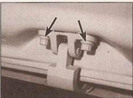
15.6 Tailgate hinge securing bolts (arrowed)
