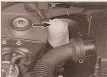
1 The brake fluid reservoir is located on the right-hand side of the engine compartment, next to the suspension strut top mounting.
