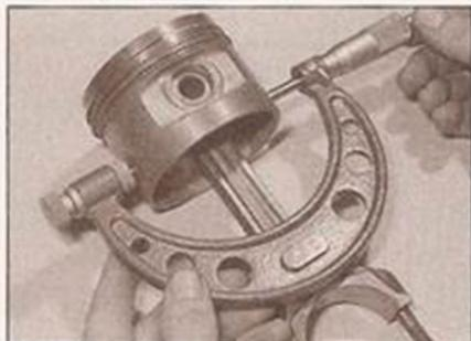
5.20 Using a micrometer, measure the diameter of all four pistons
