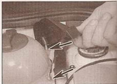
6.24 Unclip the plastic cover next to the expansion tank, for access to the mounting nuts (arrowed)
