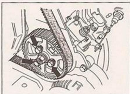
6.6 Loosen and remove ONLY the three pulley-to-hub bolts (arrowed)
