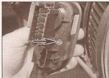
8.15 Bulbholder (arrowed) in the back of the lighting switch
