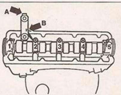
4.68 Petrol engine camshaft bearing cap orientation
