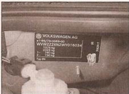
VIN plate on engine compartment bulkhead
