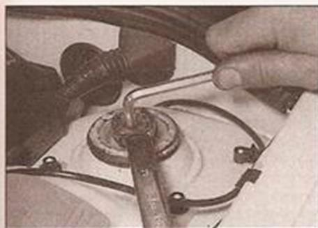
2.3a Holding the piston rod stationary with an Allen key . . .
