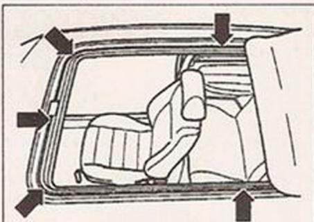
20.1 Folding fabric sunroof guide rail (arrowed)
