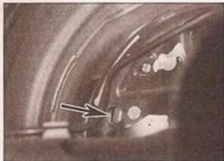
16.2 Rear brake backplate inspection hole (arrowed) for assessing brake lining wear
