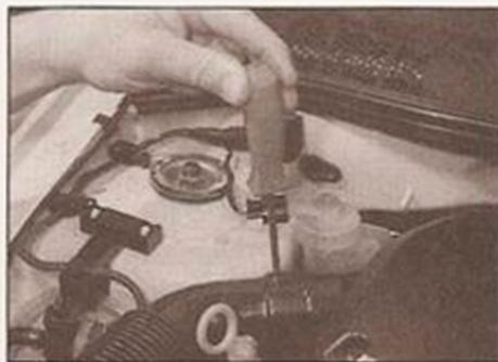
2.4 Slackening the air ducting retaining screw
