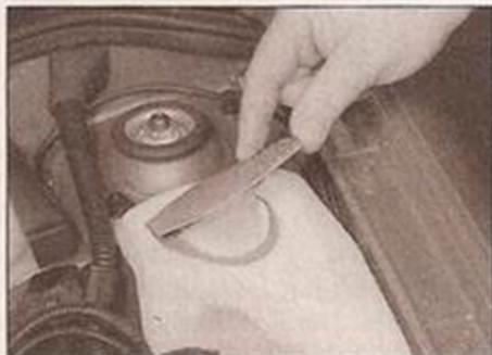
2 The screen washer level can be seen through the reservoir body. If topping-up is necessary, open the cap.
