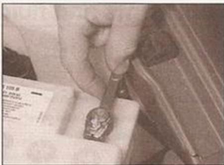
**2** Check the tightness of battery clamps to ensure good electrical connections. You should not be able to move them. Also check each cable for cracks and frayed conductors.
