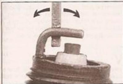
Adjusting spark plug gap
