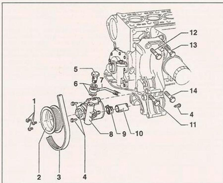
21.4 Power steering pump and associated components - typical
