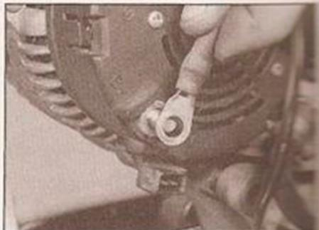
5.4b . . . remove the nut and washers, then disconnect the power cable
