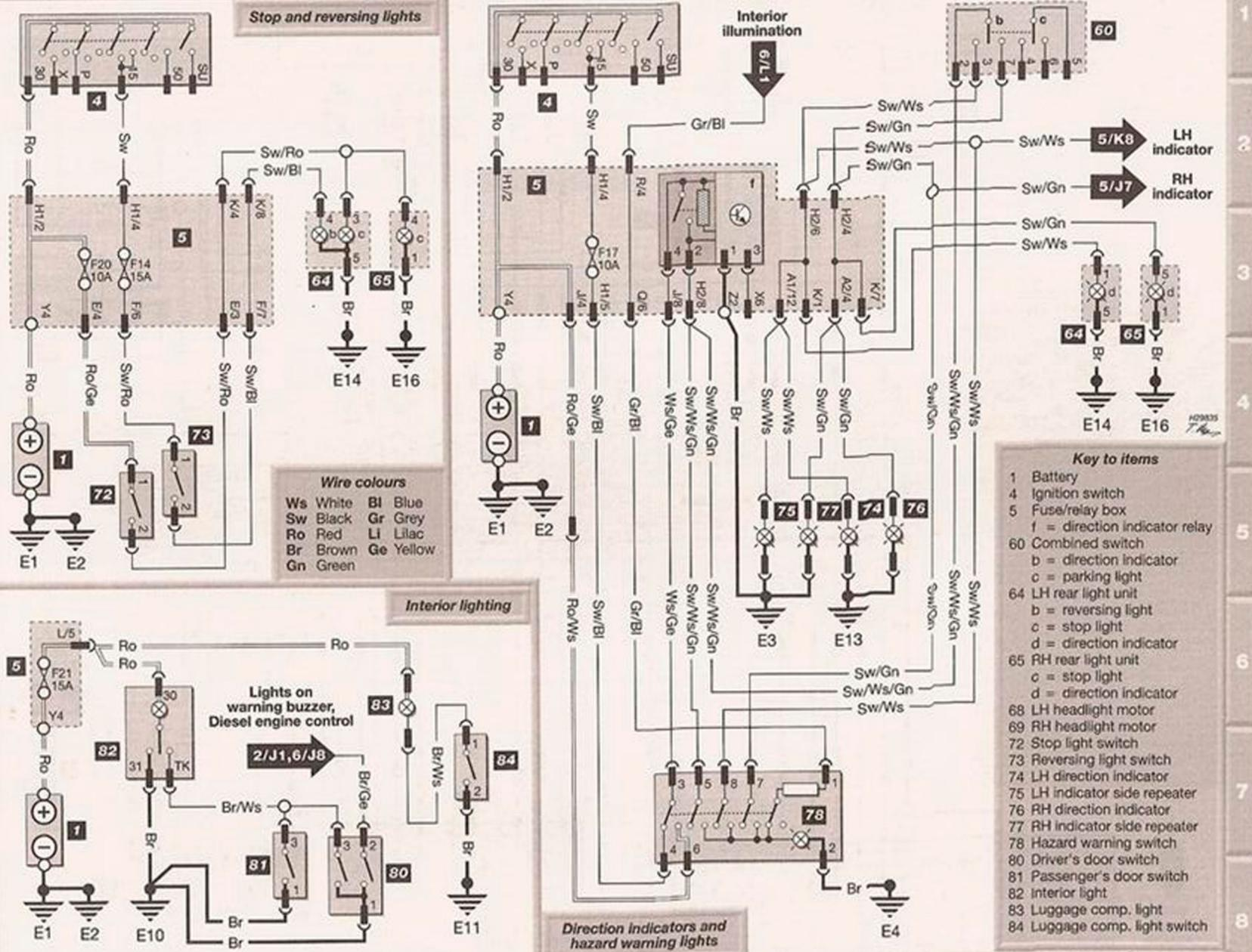
Diagram 7 : Stop, reversing, direction indicators/hazard warning lights and interior lighting - models up to 1998
