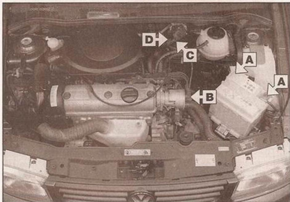
Check that electrical connections are secure (with the ignition switched off). On petrol engine models, check the four spark plug leads and the ignition coil connections at the rear of the engine compartment. Spray the connector plugs with a water-dispersant spray like WD40 if you suspect a problem due to damp.
