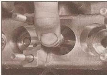
4.60b Use a long-reach socket to press on the oil seal
