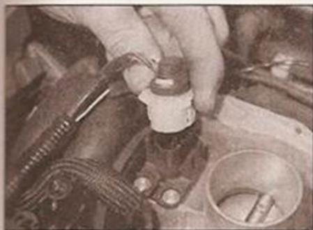
5.4a Disconnect the throttle potentiometer wiring plug . . .
