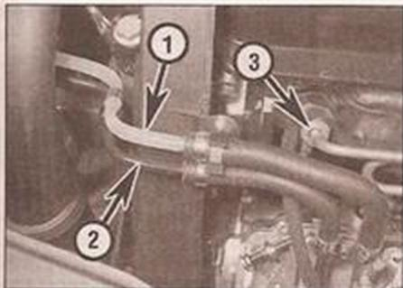
13.7 Check for leaks around the fuel supply (1) and return (2) pipes, and at the fuel injector unions (3) - one only visible
