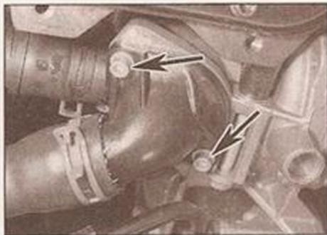
4.9 Thermostat cover and retaining bolts (arrowed) seen from below - diesel engine models
