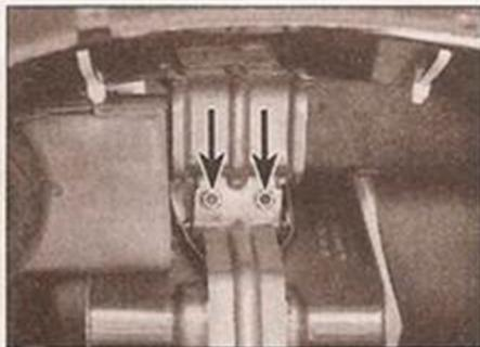
28.16b ... for access to the mounting nuts (arrowed)
