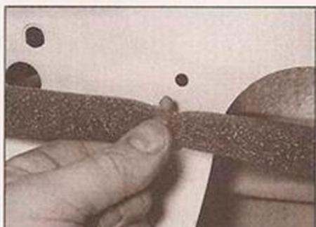
13.16b . . . detach the lock link rod from the door frame . . .
