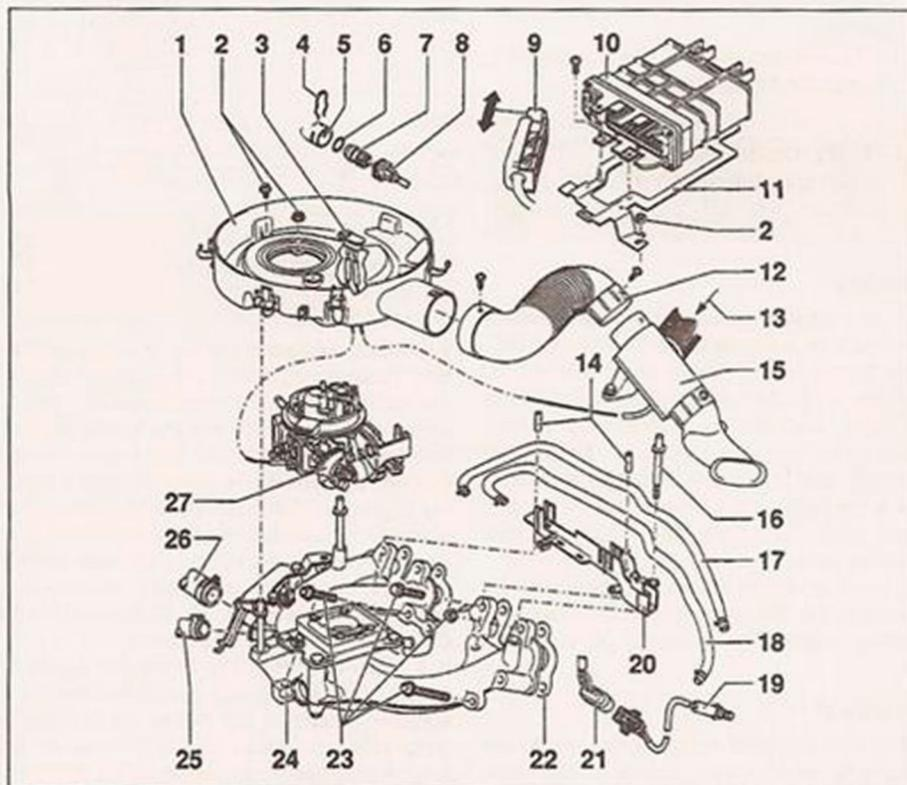
10.8 Inlet manifold and related fuel system components
