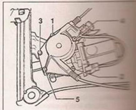
18.9 Cable drum securing screw tightening sequence
