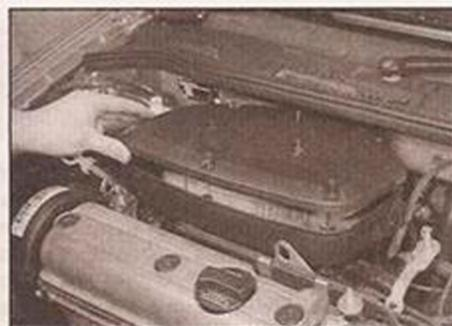
26.2b . . . then pull the housing forwards and lift off the cover
