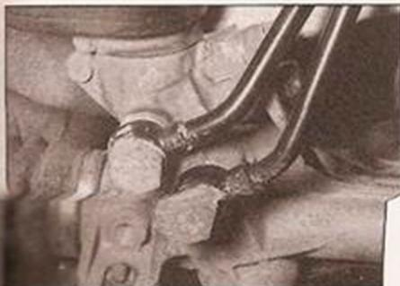
17.10a Power steering gear fluid supply and return unions
