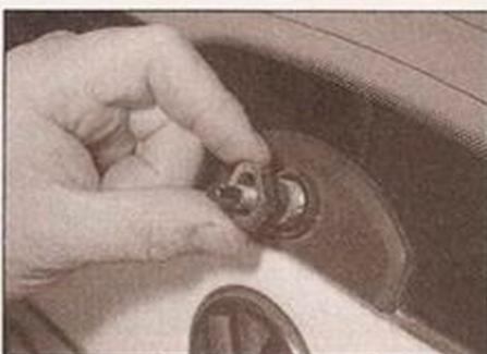
15.4a Unscrew and remove the spindle nut...
