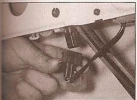
14.18 Disconnecting the electric window motor wiring plug
