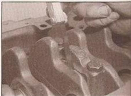
6.5 Measuring crankshaft endfloat using feeler blades
