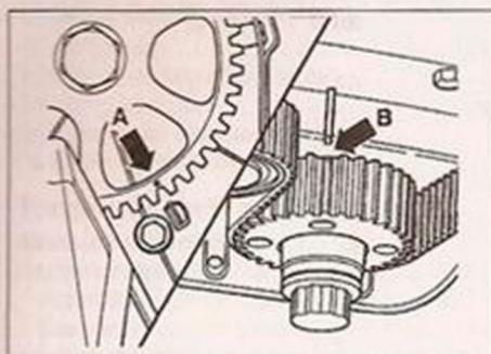
2.5 Camshaft sprocket (A) and crankshaft sprocket (B) TDC timing marks
