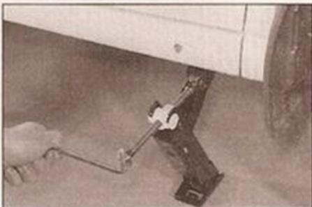
**5** Turn the jack handle clockwise until the wheel is raised clear of the ground. Unscrew the wheel bolts and remove the wheel.
