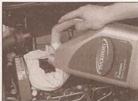
**4** Oil is added through the filler cap. Unscrew the cap and top-up the level; a funnel may help to reduce spillage. Add the oil slowly, checking the level on the dipstick often. Don't overfill (see "Car Care" left).
