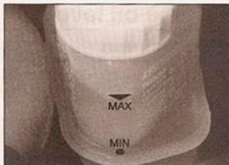
2 The MAX and MIN marks are indicated on the front of the reservoir. The fluid level must be kept between the marks at all times. If topping-up is necessary, first wipe clean the area around the filler cap to prevent dirt entering the hydraulic system.
