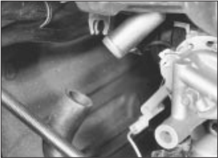
3.3b ... and crankcase emission hose - 1.3 litre
