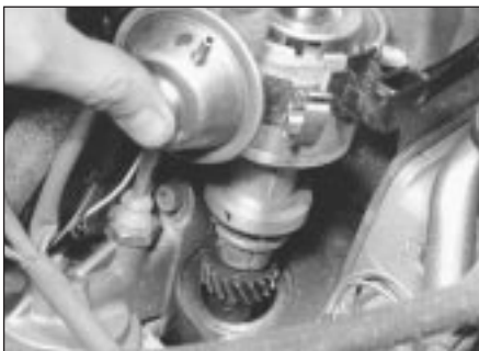
6.6a Distributor removal - 1.8 litre engine
