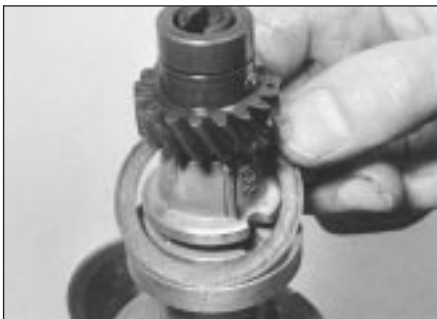
6.6b The gasket must be removed
