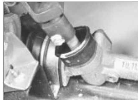
17.6 Steering gear pinion-to-lower column joint
