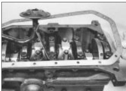
32.3 Fitting sump gasket
