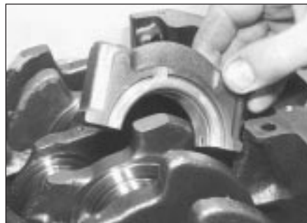
30.5 Fitting main bearing caps
