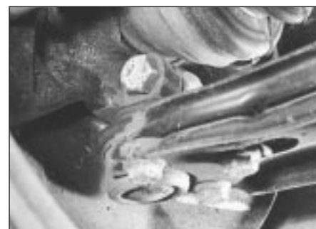
7.3 Track control arm balljoint and clamp bolt
