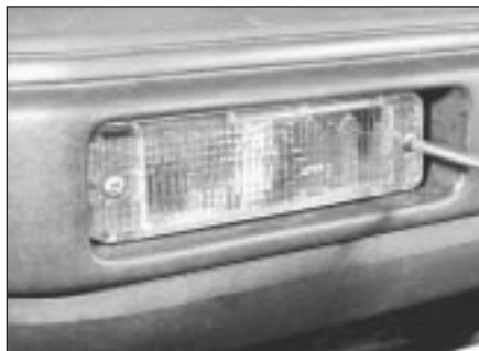
8.4 Front indicator lens removal
