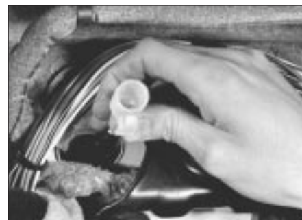
16.4 Disconnect speedometer cable
