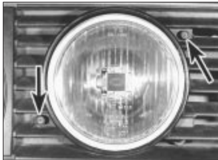
7.4 Foglight beam alignment adjuster screws (arrowed)
