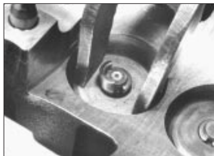
12.12c . . . and valve collets
