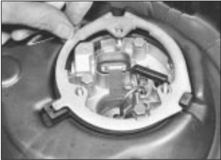
3.2 Removing air cleaner body retaining ring - 1.3 litre
