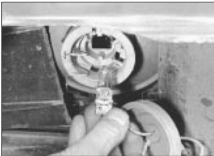
7.2 Bulb and holder removal from foglight
