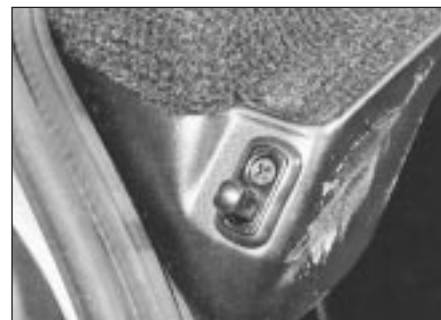
14.2 Tailgate actuated luggage compartment light switch
