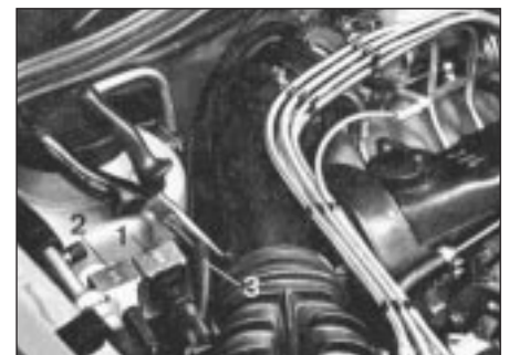
6.1 Idle speed boost valve check
