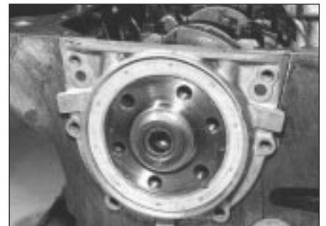
30.9 Fitting crankshaft rear oil seal and flange
