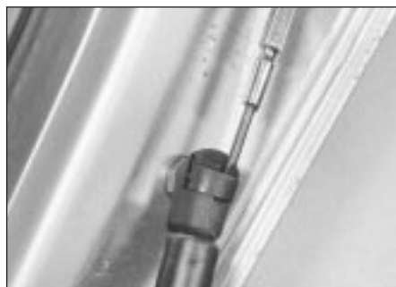
9.2a Releasing tailgate strut balljoint clip
