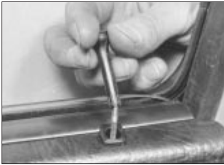
14.1 Unscrewing door locking knob
