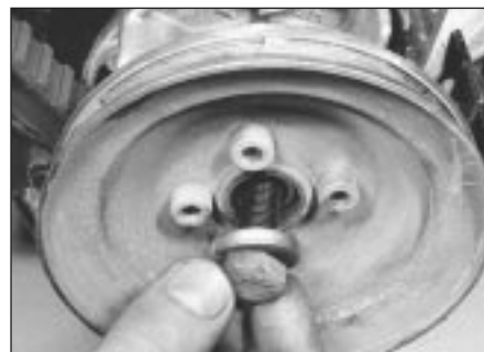
12.7 Removing crankshaft sprocket bolt and washer
