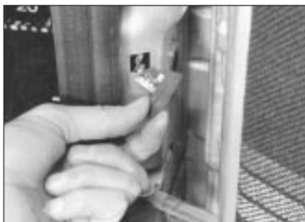
14.3 Door courtesy light switch removal
