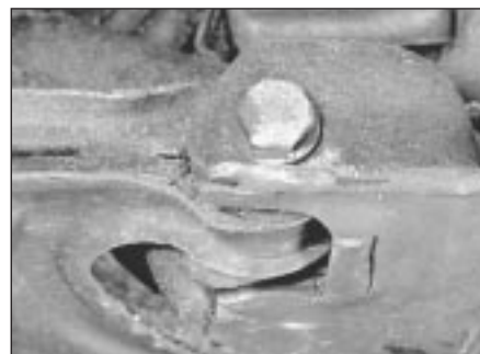
7.4 Track control arm pivot bolt
