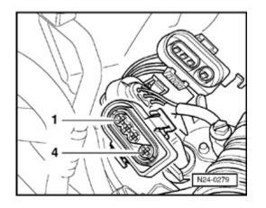
Check wiring between test box and 4-pin connector for open circuit according to wiring diagram.
