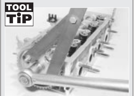
Using a home-made tool to hold the camshaft sprocket stationary whilst the retaining bolt is tightened (shown with cylinder head removed)
