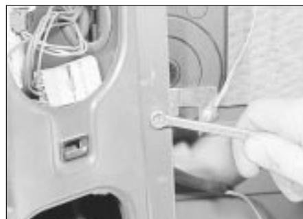
22.18b Unscrew the aerial motor securing bolt . . .
