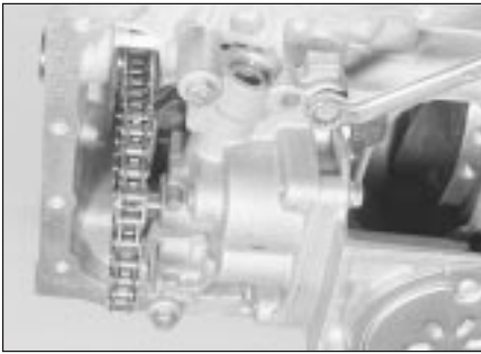
13.2 Oil pump is retained by three bolts
