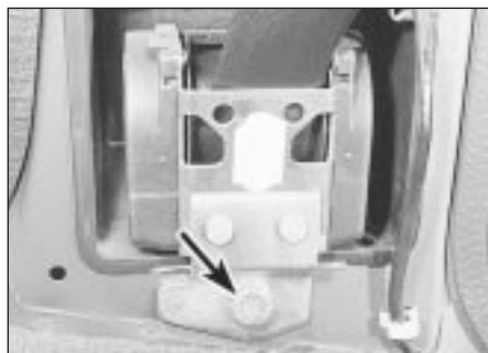
27.7 Front inertia reel securing bolt (arrowed)
