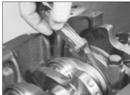
14.3 Checking crankshaft endfloat using feeler gauges
