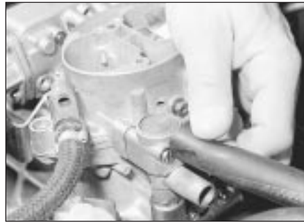
12.5 Disconnecting the float chamber breather pipe
