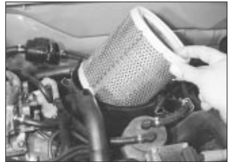
21.3 Removing the air cleaner element on TU models
