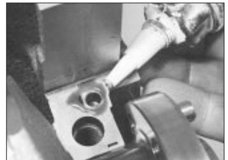
18.71 Applying sealant to the cylinder block No 1 main bearing cap mating face
