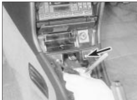
29.32a Remove the front securing screws . . .
