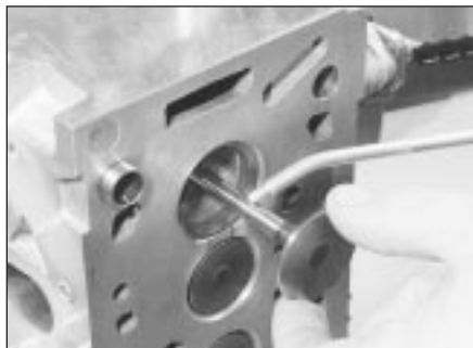
9.1 Lubricate the valve stems prior to refitting
