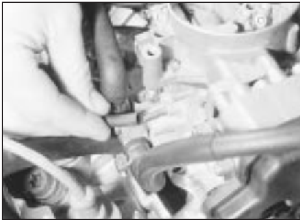
12.4 Disconnecting the distributor vacuum pipe
