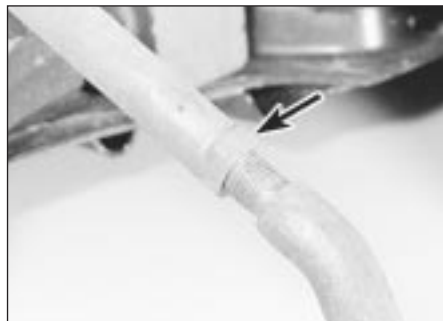
22.3 Track rod end locknut (arrowed)
