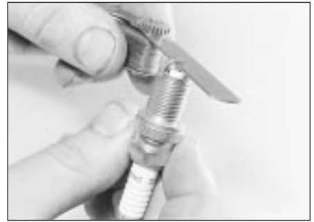
11.12 Measuring the spark plug gap with a feeler blade
