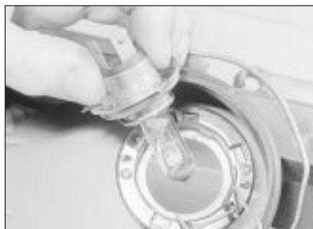
5.4b . . . then withdraw the headlight bulb
