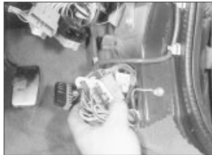
30.43 Pull the connector bracket from the footwell
