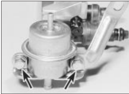
14.37 Regulator-to-fuel rail bolts (arrowed) - assembly removed for clarity
