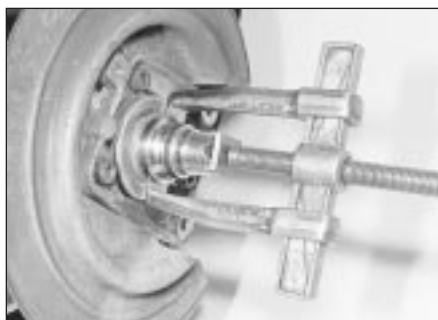
10.6b Removing the inner bearing race . . .
