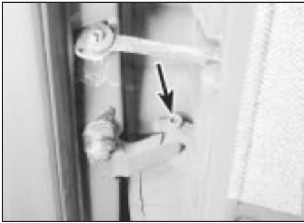
12.6 Door pivot pin (arrowed)
