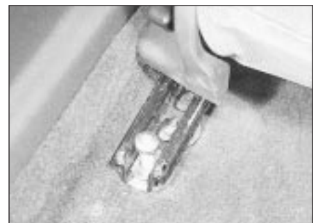
26.3 Front seat rear securing bolt partially removed
