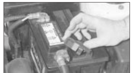
E Check that the ignition coil wiring plug is secure, and spray with water-dispersant if necessary.
