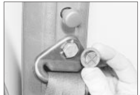
27.3 Removing the trim plate from the front seat belt upper anchor bolt
