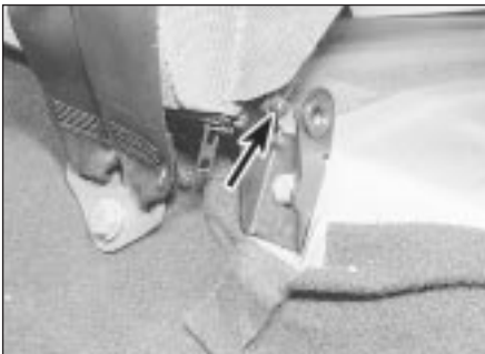
26.18b Split rear seat back inner pivot (arrowed) - Estate model
