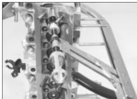
7.4a Compress the valve spring using a spring compressor . . .
