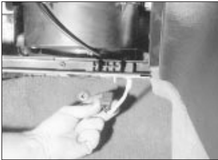
9.59 Disconnect the blower motor wiring plug
