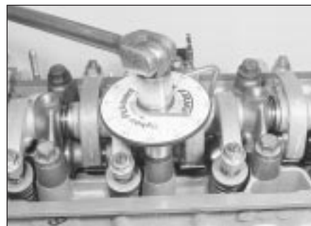
11.38 . . . then through the angle specified for stage 2
