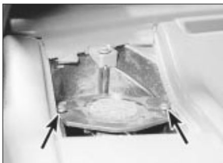
21.7 . . . for access to the loudspeaker screws (arrowed) - models up to 1992
