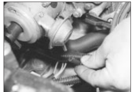
4.3b . . . and the vacuum diaphragm hose
