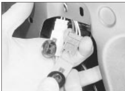
22.3 Disconnecting the door mirror wiring connectors
