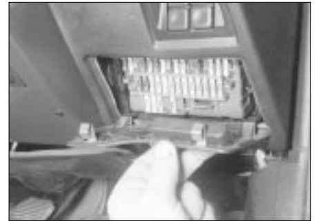
3.3c Removing the fusebox cover - later models
