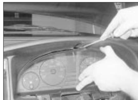
9.22 Lever the upper securing clip down . . .
