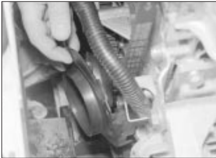
5.7 Undo the retaining bolt and remove the lower timing belt cover
