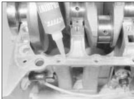
18.43 Apply a film of suitable sealant to cylinder block/crankcase mating surface . . .
