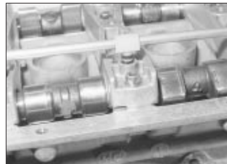
10.55 Take care not to displace the O-rings when refitting the oil supply pipe to the camshaft bearing caps
