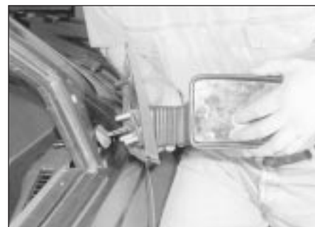
22.6b . . . and withdraw the mirror
