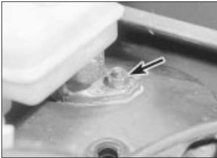
13.5 Master cylinder securing nut (arrowed)
