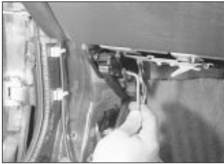
30.53 Remove the screw and withdraw the bonnet release lever
