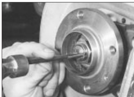
10.4b . . . then tap up the staking on the hub nut
