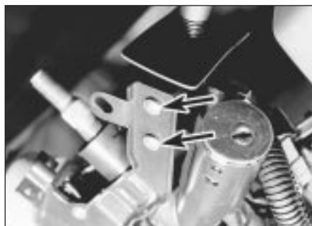
4.3 Steering column combination switch screws (arrowed) - models up to 1992
