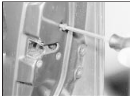
14.16 Remove the door lock securing screws
