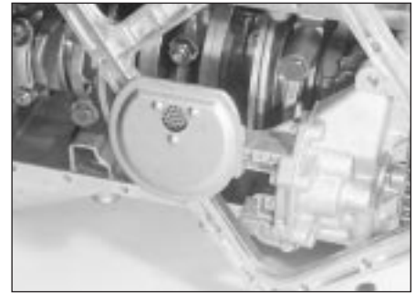
13.11b . . . then refit the plate to the base of the cylinder block/crankcase
