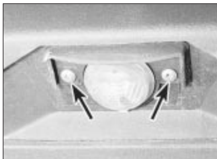
7.36 Number plate light securing screws (arrowed) - Saloon model
