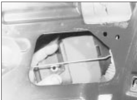
14.7c . . . and withdraw the plastic shield - later model
