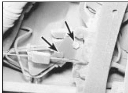
21.4 Rear brake pressure-regulating valve securing bolts (arrowed)
