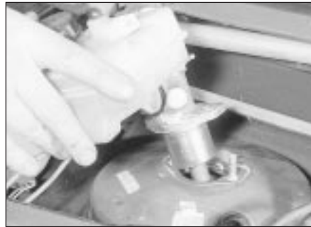
13.7 Removing the master cylinder from the vacuum servo
