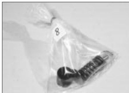
7.7 Place each valve and its associated components in a labelled polythene bag
