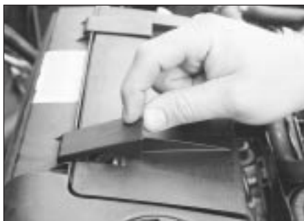
21.14b ... and release the retaining clips
