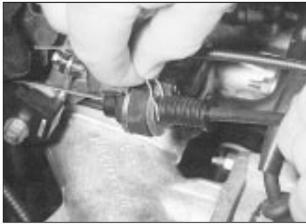
7.9 Adjusting the accelerator cable
