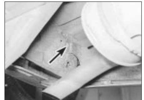
7.11 Rear underbody shield securing clip (arrowed) - Estate model
