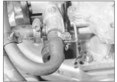
12.6a Automatic choke coolant pipe connection . . .
