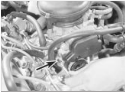
10.7 Idle mixture adjustment screw (arrowed)
