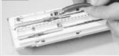
A length of rubber tubing can be used to remove and refit the bulbs
