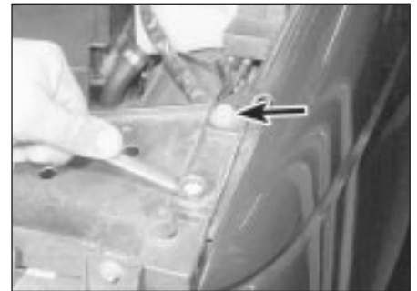
11.14 Unscrew the body front panel upper securing bolts
