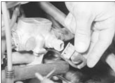
14.48 Disconnecting the injection thermistor wiring
