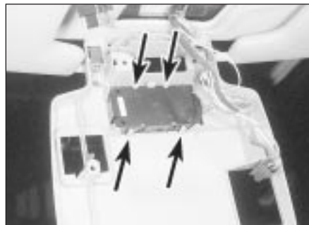
20.33 Central locking remote control receiver securing clips (arrowed)
