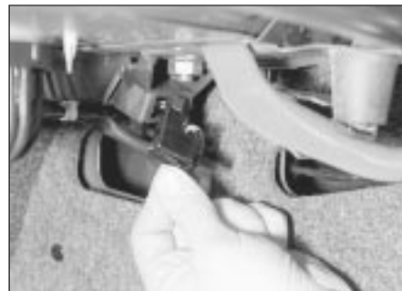
4.35 Removing the luggage compartment courtesy light switch - Saloon model
