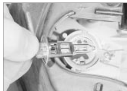
5.23b Removing a headlight-mounted driving light bulb
