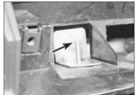
30.23 Upper facia securing bolt (arrowed)
