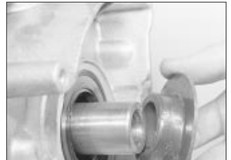
7.12 Remove the flanged spacer if necessary
