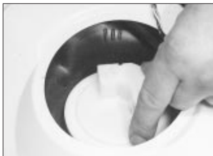
10.1 Removing the fuel gauge sender unit
