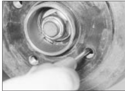
9.3b Releasing the handbrake operating lever
