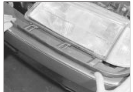
7.7 Removing the trim plate from the bottom of the headlight
