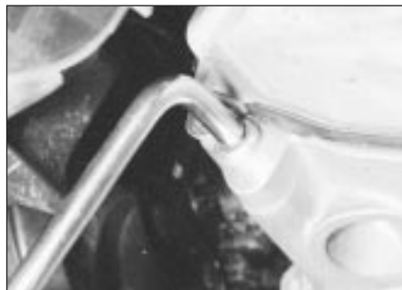
26.3 Using a square-section wrench to unscrew the transmission filler/level plug (MA transmission shown)
