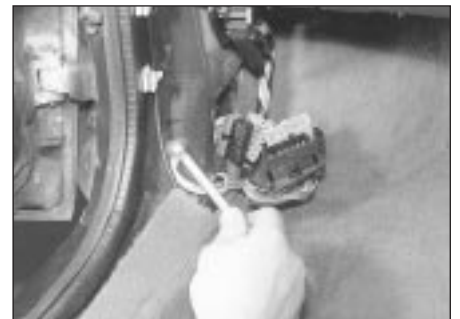
30.52 Unbolt the earth lead from the passenger's footwell
