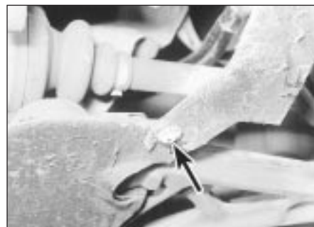
9.6 Remove the (arrowed) screws securing the underbody shields to the subframe
