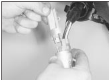
18.8b . . . slide the rear section from the lock body . . .
