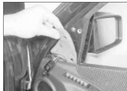
22.5a Prise off the sealing strip . . .
