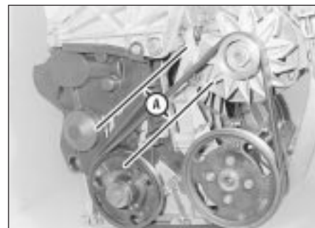
5.11 Alternator drivebelt deflection (A)
