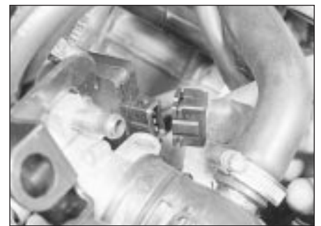
12.5 Disconnecting the multi-plug
