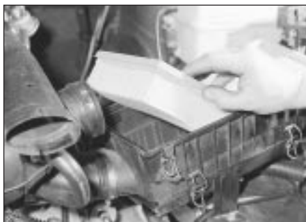
21.9 Removing the air filter element
