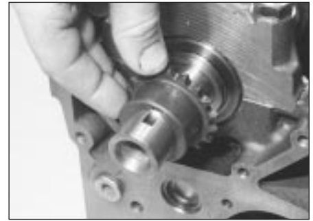
11.16b . . . then slide off the drive sprocket . . .
