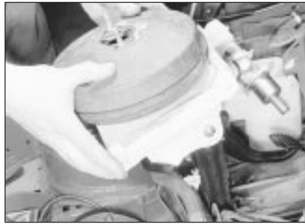
15.15 Removing the vacuum servo/pedal bracket assembly
