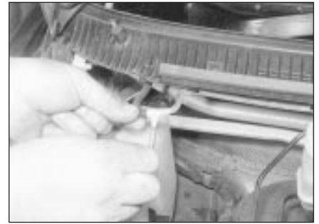
25.8 Disconnect the washer fluid hose
