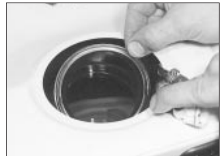
9.12b . . . and recover the rubber sealing ring
