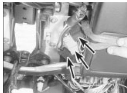
17.8 Ignition switch wiring connectors (arrowed) - models from 1993
