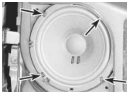
21.3 Door-mounted loudspeaker securing screws (arrowed)
