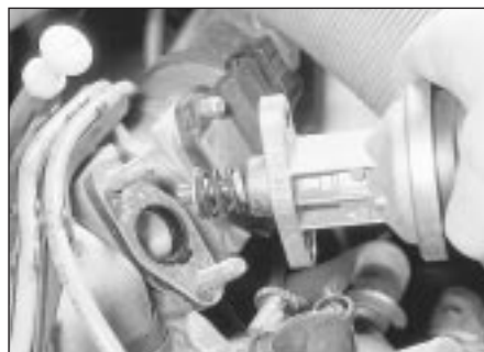
4.5 Removing the fuel pump (XU engine)
