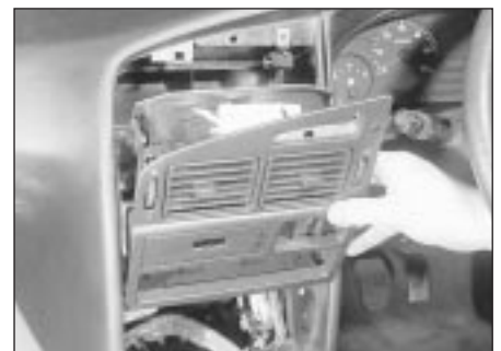
30.40 Withdrawing the ventilation nozzle housing
