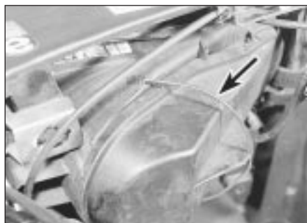
5.2 Headlight rear cover securing clip (arrowed)
