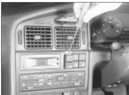
30.39a Prise the switches from the housing . . .
