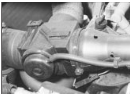
3.17 Air temperature control valve assembly (TU engine)
