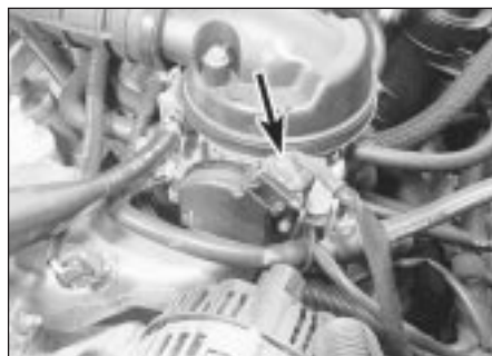
16.14 Throttle potentiometer wiring connector (arrowed)
