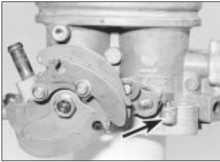
14.6a Secondary throttle adjusting screw (arrowed) ...
