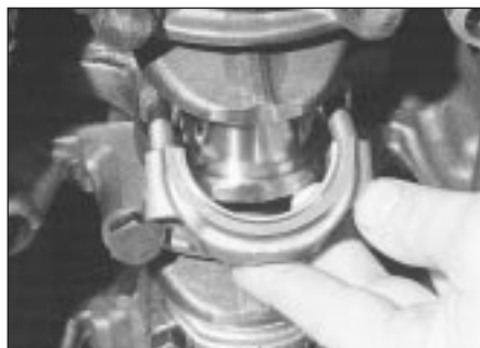
10.5 Removing a big-end bearing cap and shell
