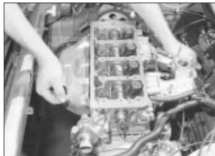
11.33 . . . then lower the cylinder head into position . . .
