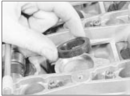
4.32 Fitting a spark plug hole oil seal
