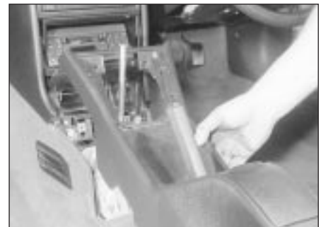
29.32b . . . and withdraw the console ("Lowline" console - models from 1993)
