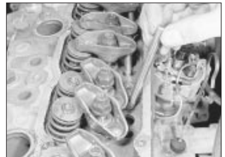
8.17 Removing the pushrods
