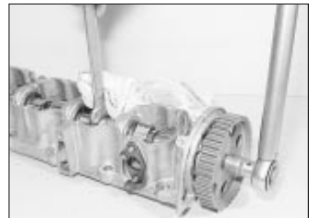
9.12b Tightening the camshaft sprocket bolt
