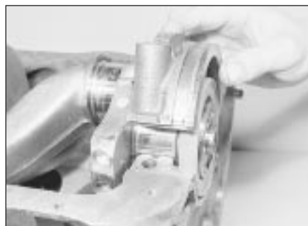
20.16 Fitting the rear main bearing cap
