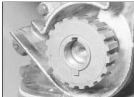
13.2a Removing the crankshaft sprocket
