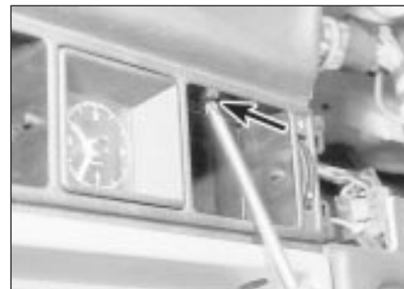
10.3 Removing a centre vent housing screw
