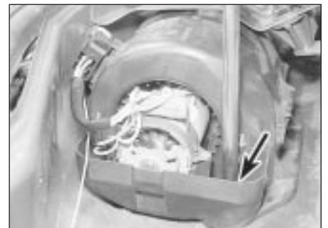
9.9 Removing a blower motor securing nut
