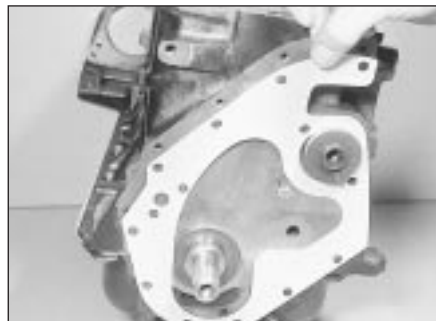
18.10 Fitting a new front plate gasket
