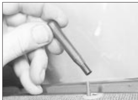
12.4 Unscrewing the lock button
