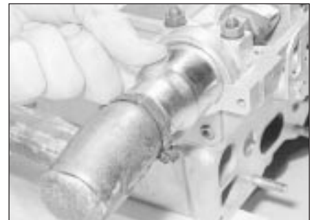
9.4b Seating a camshaft oil seal
