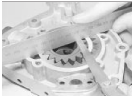
14.3 Checking oil pump gear endfloat
