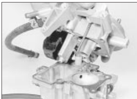
21.3 Lifting off the carburettor top cover
