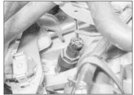
25.22 Speedometer sender (used with digital instrument panel)
