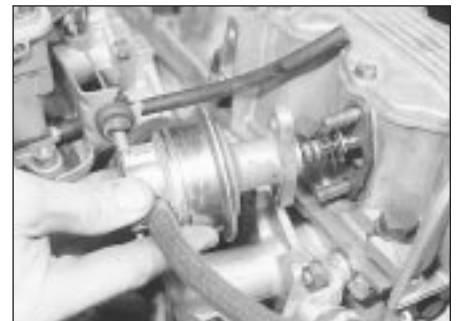
5.5 Removing the fuel pump (1.3 litre engine shown)
