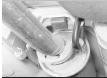
27.4b Exhaust system rubber mounting ring
