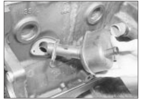
22.8 Crankcase ventilation system oil separator - 1.3 litre engine
