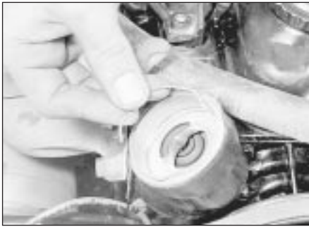
4.3a Remove the thermostat retaining snap-ring . . .
