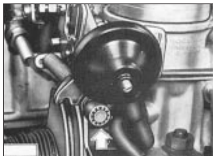
13.2 Fast idle adjustment screw (arrowed)
