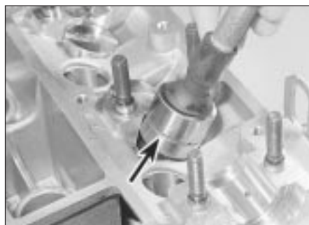
12.4 Removing a tappet. Note the oil ring (arrowed)
