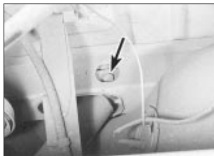
12.14 Rear shock absorber top mounting bolt (arrowed) - Estate
