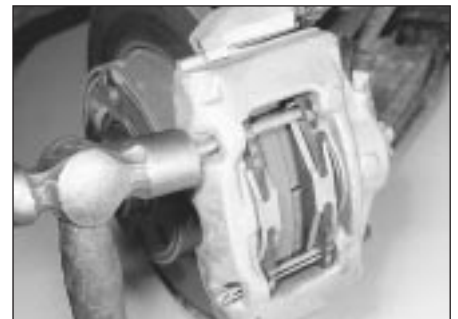
4.10a Inserting disc pad pin
