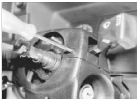
20.3a Removing an upper shroud securing screw
