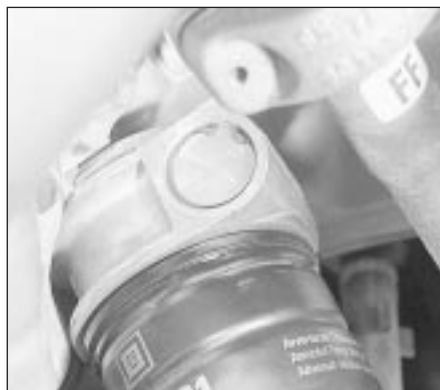
16.2 Circlip securing oil cooler thermostatic valve
