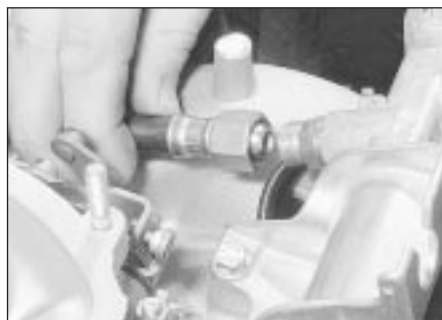
12.60 Disconnecting the fuel supply line from the fuel rail
