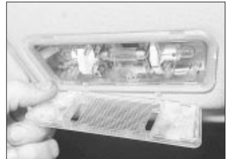
11.25c Removing the cover from the main interior lamp
