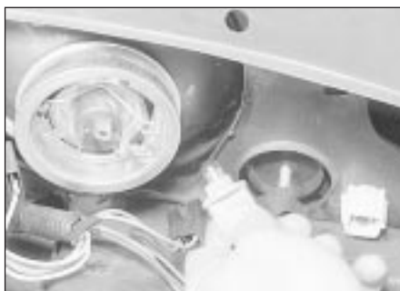
11.7 Removing a sidelamp bulb and holder
