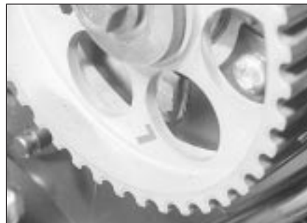
10.4 Exhaust camshaft sprocket is marked 'L'
