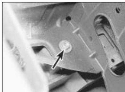
8.3 Front trim panel securing nut (arrowed)
