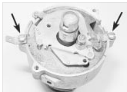
7.7 Undo the baseplate retaining screws (arrowed)
