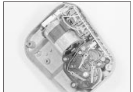
21.13c . . . and remove the motor cover to gain access to the motor wiring
