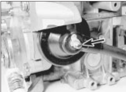
14.8a Choke valve gap adjustment screw (arrowed)
