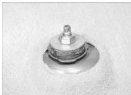
12.2 Rear shock absorber upper mounting - Hatchback
