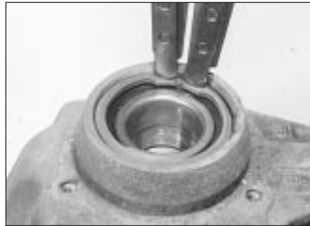
3.5b Removing a hub bearing circlip
