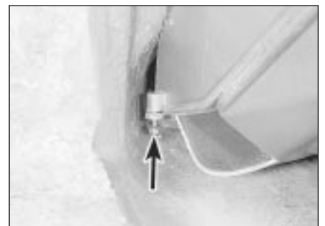
9.15b Air distribution housing lower screw (arrowed)
