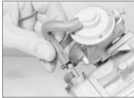
19.4 Disconnecting the vacuum hose
