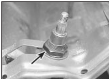
20.4 Wiper spindle clamp nut (arrowed)
