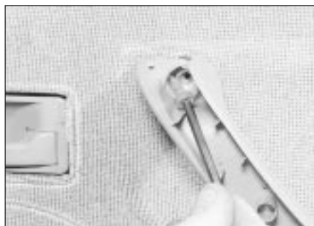
12.6b Removing an armrest screw
