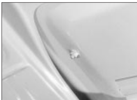
26.9 Boot lid handle retaining nut
