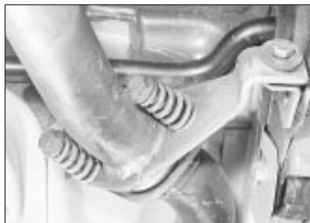
14.5 Manifold-to-exhaust system joint and bracket
