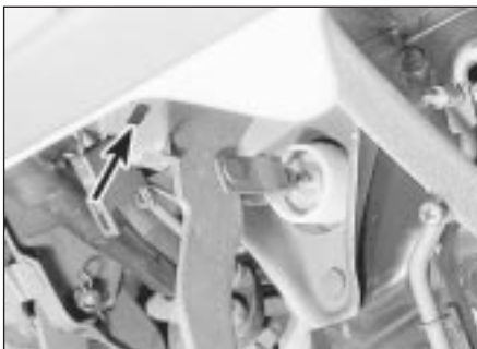
17.1 Stop-lamp switch 'keyhole' mounting (arrowed)
