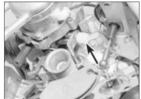
15.4 Fast idle adjustment screw under tamperproof cap (arrowed)
