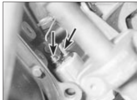
13.2 Oil pressure sender wires (arrowed)
