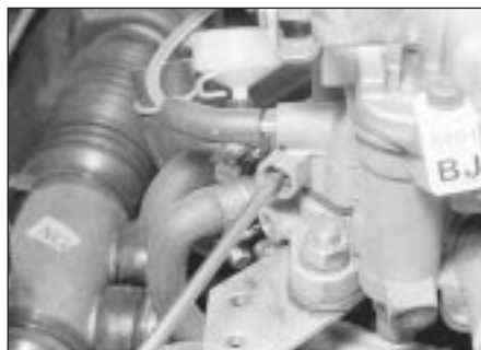
11.4c Adjusting the idle speed - Varajet carburettor
