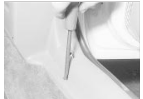
12.46a Remove the kick plate screws . . .
