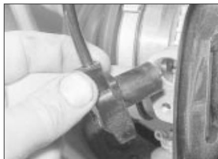
22.2c Removing a front wheel speed sensor
