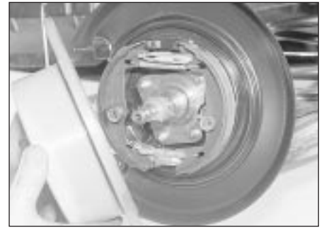
8.5 Removing the rear disc
