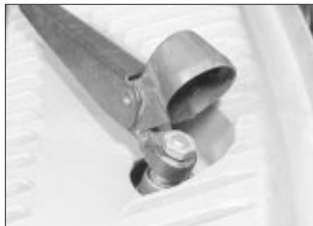
19.3 Wiper arm retaining nut
