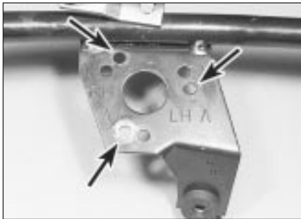
20.9 Choice of wiper motor mounting holes - RHD arrowed
