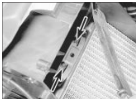
9.17b Heater matrix upper securing screws (arrowed)
