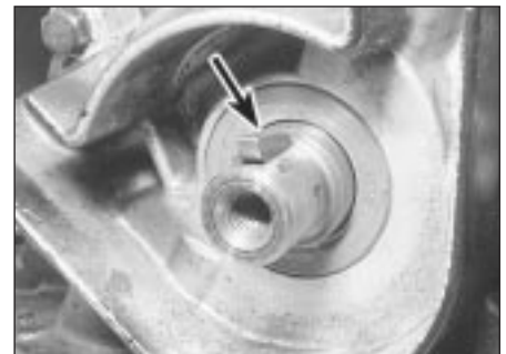
13.2b Woodruff key (arrowed) in crankshaft nose
