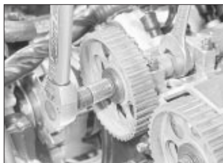
10.14 Tightening a camshaft sprocket bolt
