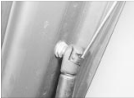
22.2 Releasing a tailgate strut spring clip
