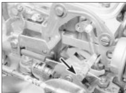
10.5 Choke cable inner clamp screw (arrowed)
