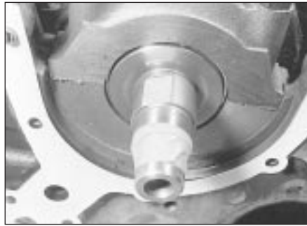
13.6 Tape the crankshaft nose
