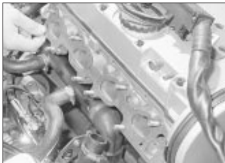
13.33 Fitting a new inlet manifold gasket
