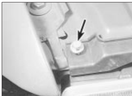
12.3a Headlamp lens outboard securing screw (arrowed)
