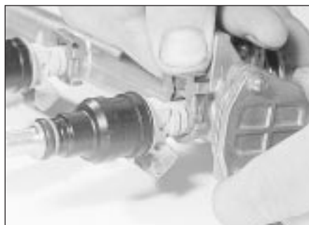
12.69a Remove the retaining clip
