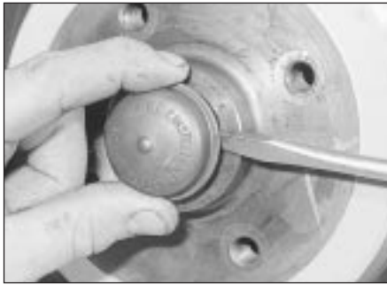
8.3 Levering off the grease cap
