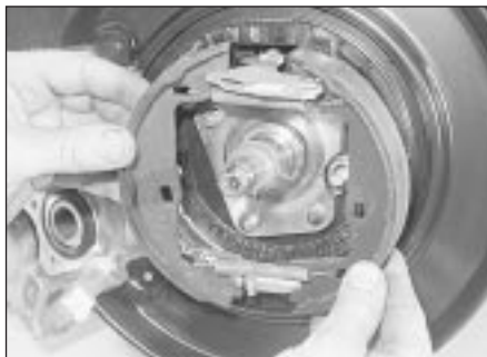
20.4 Removing the handbrake shoe assembly
