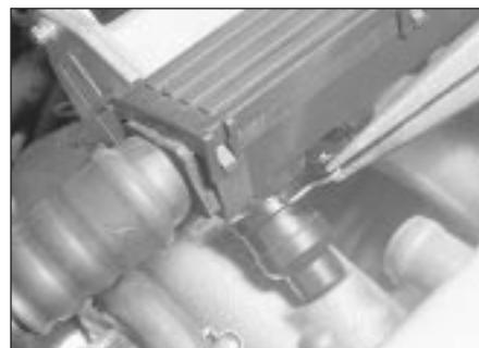
12.66a Removing the spring clip from an injector multi-plug
