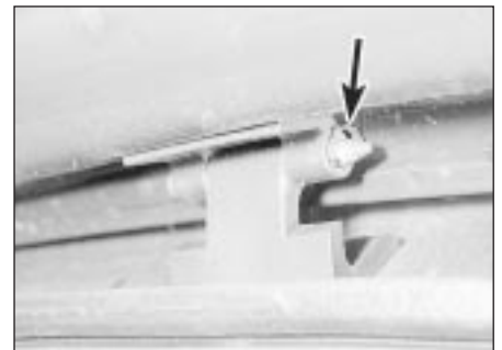
20.4 Tailgate hinge showing circlip (arrowed)
