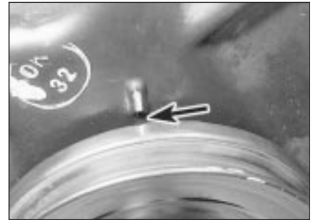
7.7 Ignition timing marks (arrowed) in alignment
