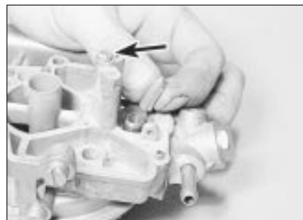
19.14 Removing the float needle valve. Main jet is arrowed
