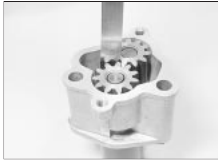
13.8 Check the pump gear teeth backlash
