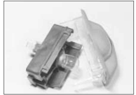
11.23 Number plate lamp bulb holder and lens separated
