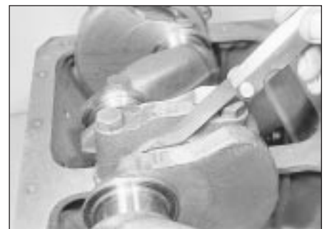
20.18 Checking the crankshaft endfloat
