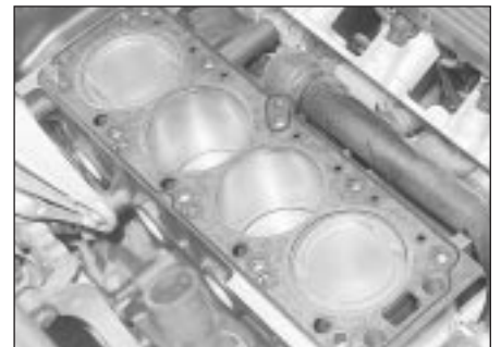
11.22 New head gasket in position
