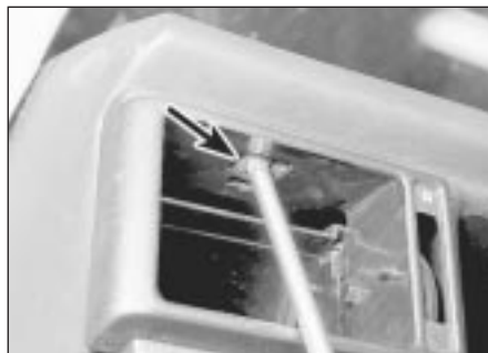
10.2 Removing a swivelling vent housing securing screw
