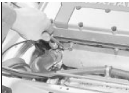
14.3 Removing an exhaust manifold heat shield bolt
