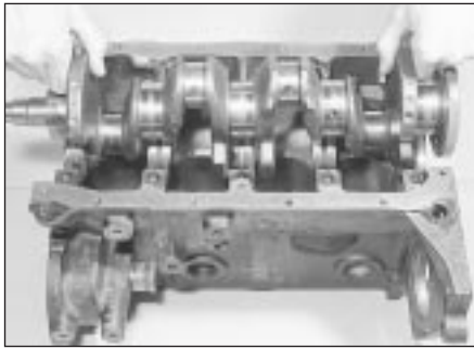
20.15 Fitting the crankshaft
