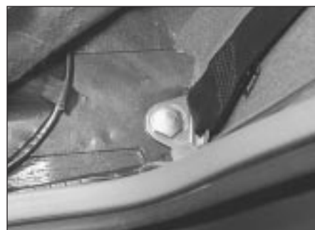
37.7c Rear seat belt floorpan mounting
