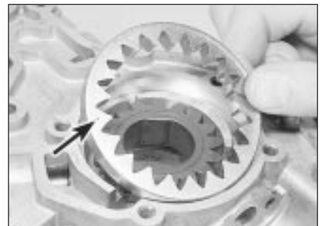
14.4 Gear outer face identification mark (arrowed)
