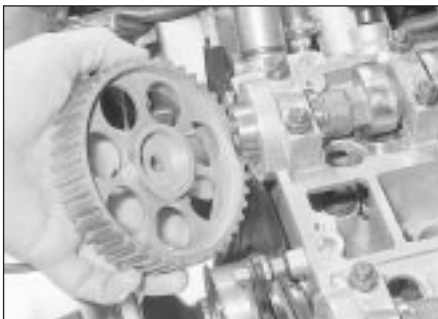
10.3b Removing a camshaft sprocket
