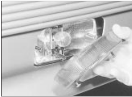
11.19 Removing a rear foglamp lens
