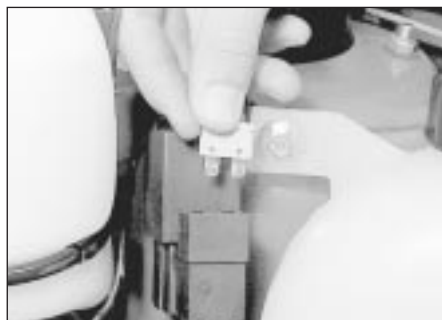
3.7b Removing the headlamp washer fuse
