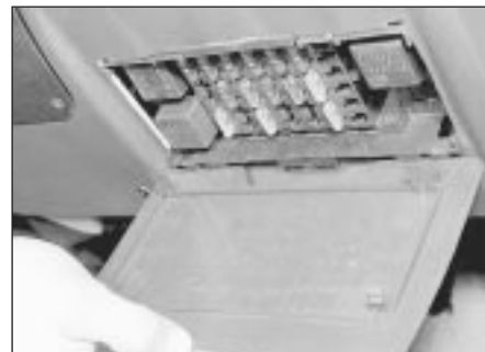
3.1 Removing the cover from the fuse/relay box
