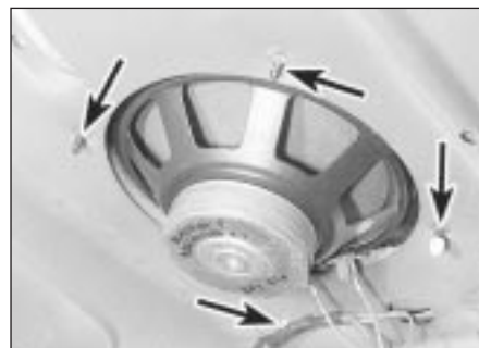
26.2b . . . the speakers are retained by four screws
