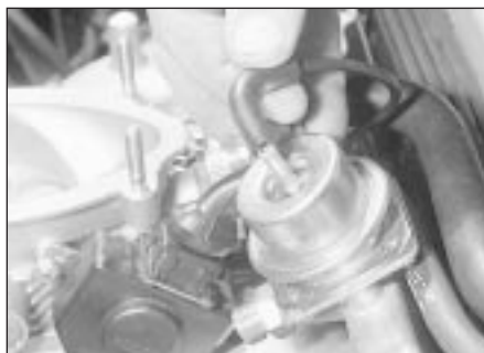
12.74 Disconnecting the vacuum hose
