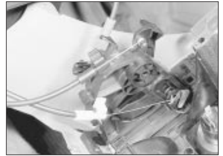
9.5 Removing the heater control panel
