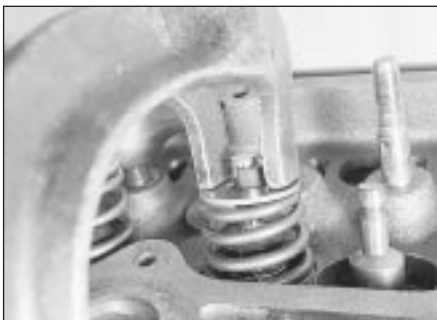
9.20 Compress the spring and fit the collets
