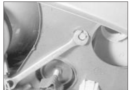
12.2a Undoing a direction indicator lens screw
