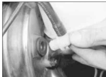
15.3 Brake servo vacuum connection at servo
