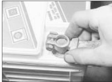
4.2 Disconnect the battery negative terminal first
