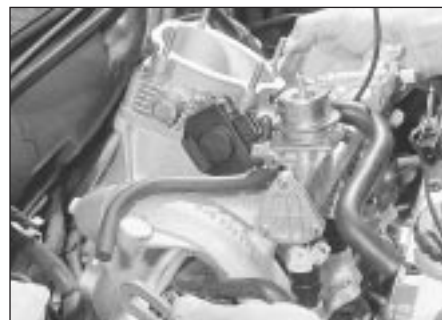
13.32 Removing the inlet manifold - 2. litre 16-valve model
