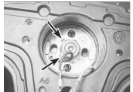
19.4 Steering wheel retaining nut and locktabs (arrowed)
