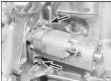
10.7 Starter motor mounting bolts (arrowed) - engine removed for clarity
