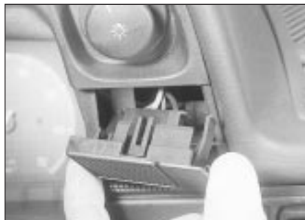
4.5 Removing a foglamp switch
