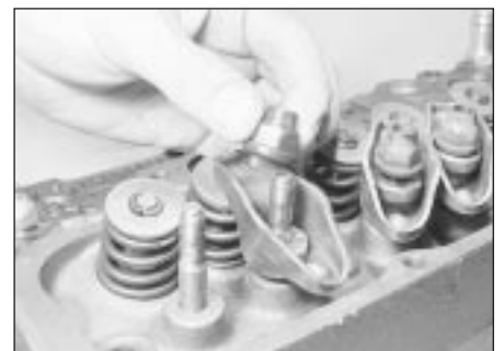
9.25 Fit the nut with the self-locking collar uppermost
