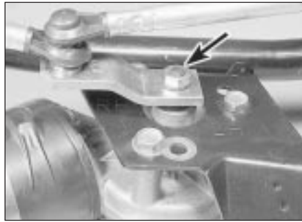
20.8a Wiper motor spindle nut (arrowed)
