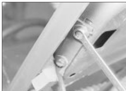
6.3 Removing a bonnet hinge bolt
