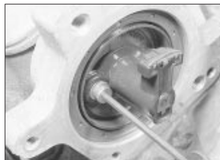
3.10a Undo the two Allen screws . . .
