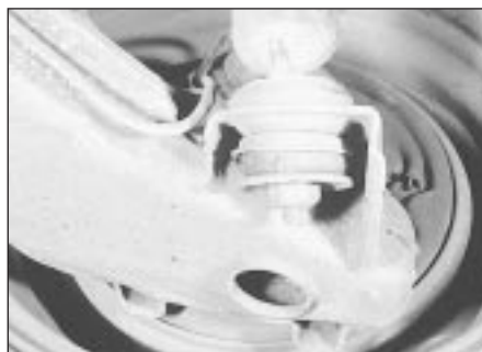
12.13 Rear shock absorber lower mounting - Estate
