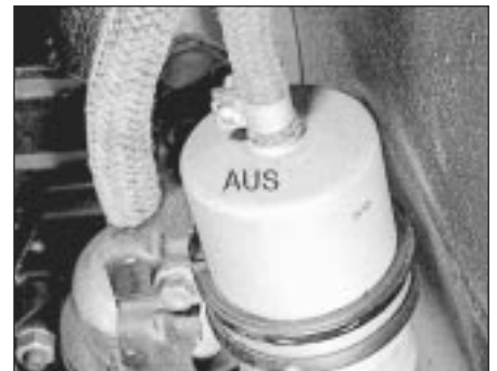
25.4 Fuel filter directional marking
