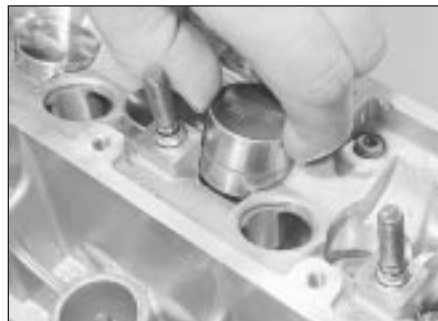
12.16b . . . and fitting it to its bore
