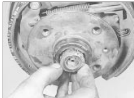
10.6a Fit the outer bearing race . . .
