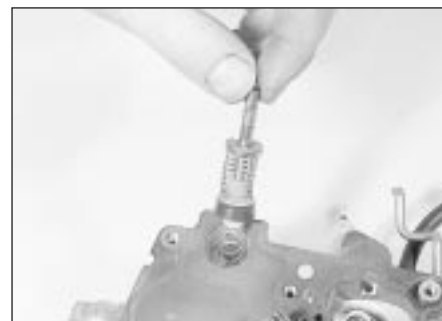
23.10 Accelerator pump plunger and spring
