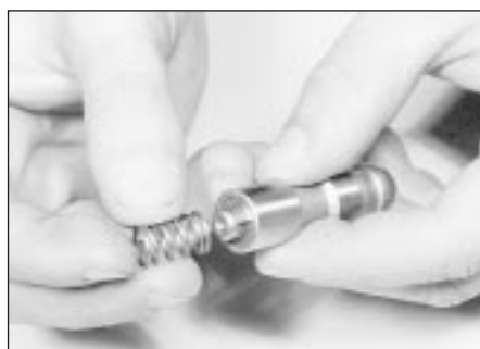
10.14a Locate the spring over the plunger cap . . .
