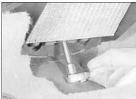
9.17a Removing the heater matrix lower screw
