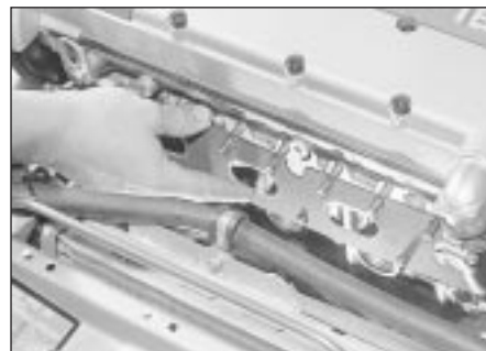
14.8 Fitting a new exhaust manifold gasket
