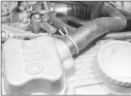
22.7a Crankcase ventilation hose attached to camshaft cover (1.8 litre engine shown)
