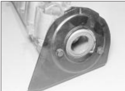
9.7 Camshaft belt cover backplate (1.3 litre engine shown)
