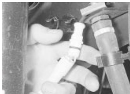
22.3b Separating a front sensor connector
