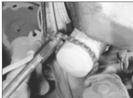
6.9 Using an oil filter removal tool to unscrew the oil filter
