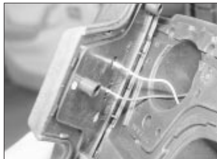
19.2 Removing the steering wheel central cap
