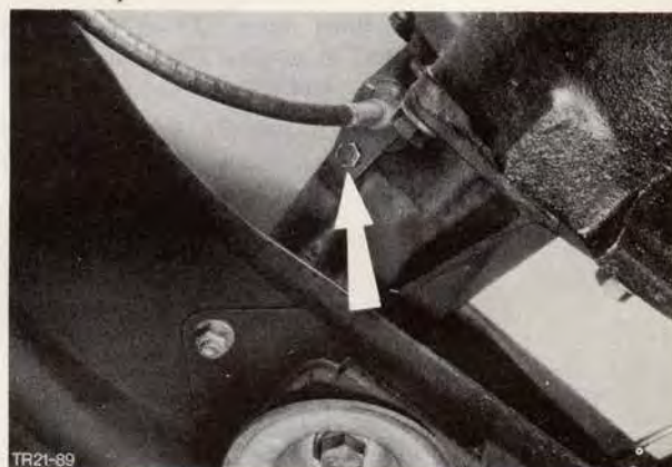
Fig. 23. Remove speedometer drive cable
