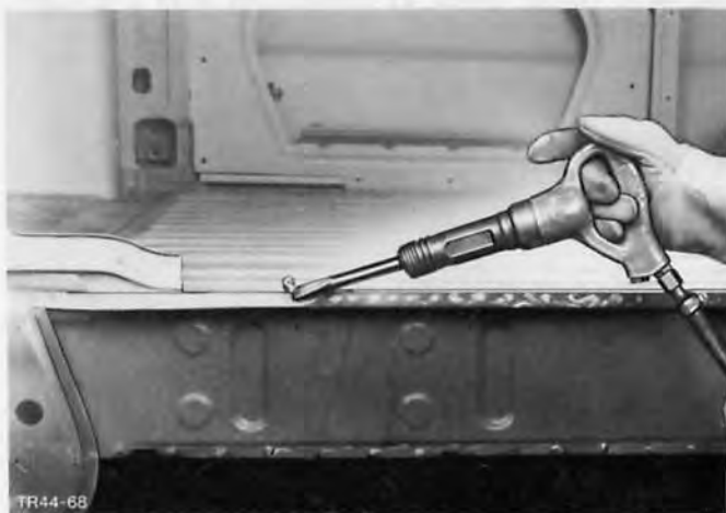
Fig.125. Remove metal remnants.
