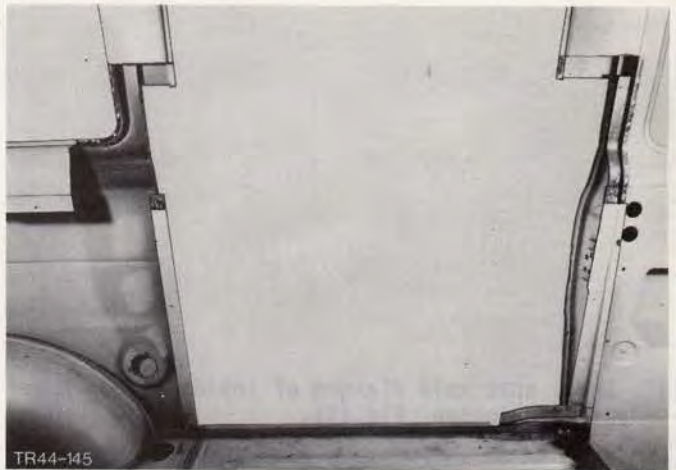
Fig.148. Side panel and inside window panel cut out, viewed from inside.
