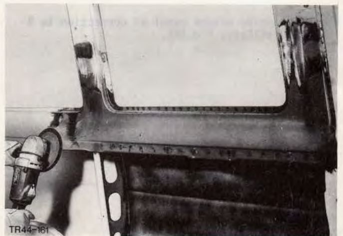
Fig.164. Dress solder-fill locations on inside window panel.
