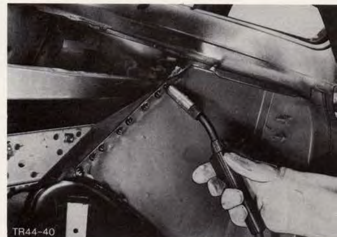
Fig.71. Weld apron panel to side panel.
