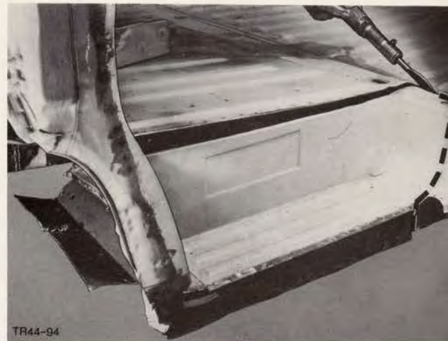
Fig.136. Cut out entrance step.
