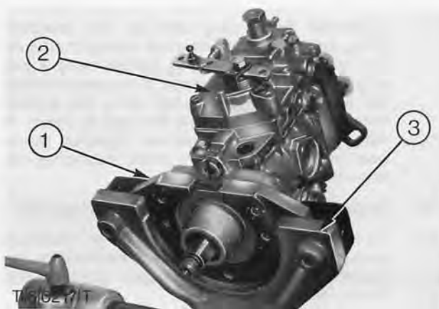
Fig. 15. Mounting the fuel pump 1. Adaptor Special Tool No. 1 685 720 062 2. Fuel injection pump 3. Mounting yoke Special Tool No. KDEP 2963
