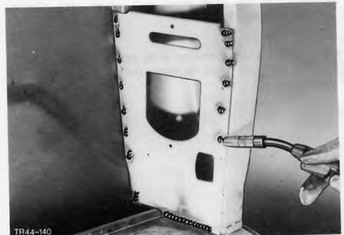
Fig.176. Plug weld box corner reinforcement.
