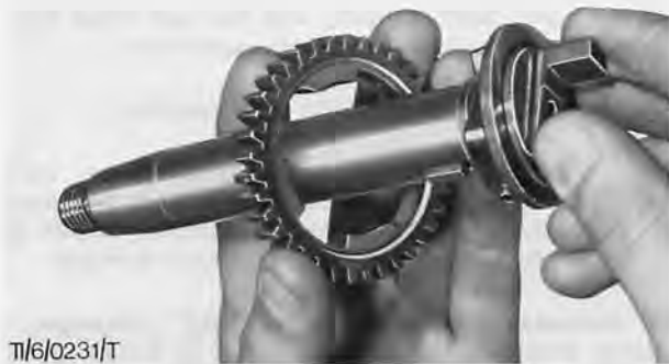
Fig. 30. Fit gear to shaft; recess to drive coupling
