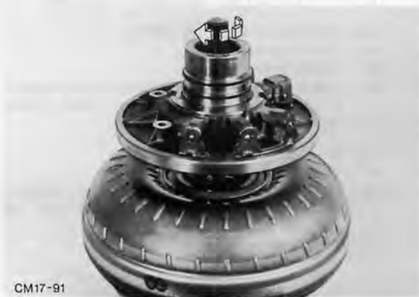
Fig. 14. Check for contact between stator and turbine
