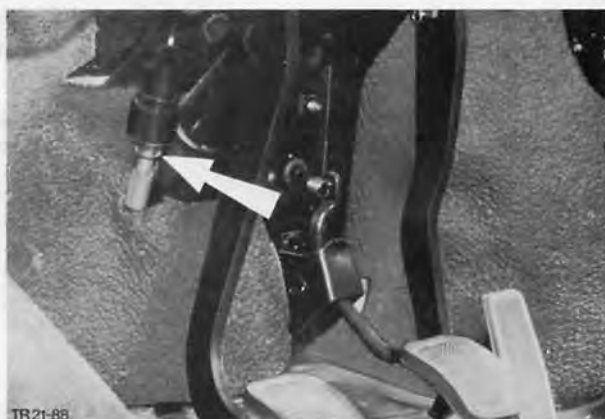
Fig. 29. Adjust clutch cable clearance
