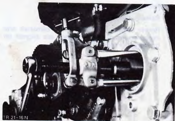
Fig. 133. Remove camshaft oil seal using Special Tool 15-048/048-01
