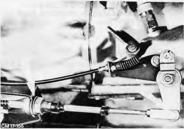
Fig. 34. Fit selector lever cable
