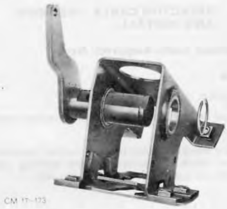
Fig. 46. Install and secure shift shaft
