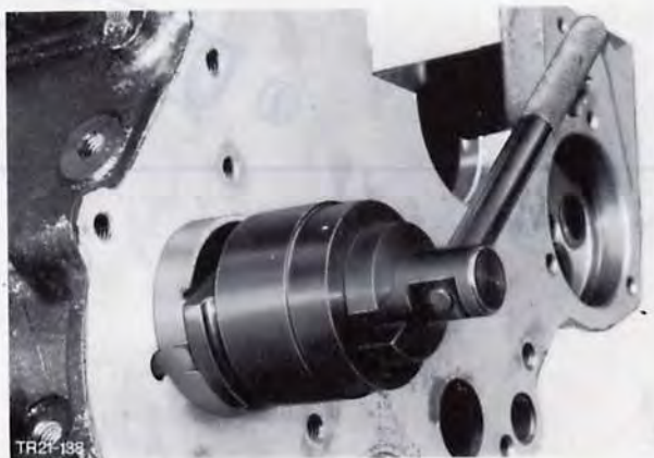
Fig. 127. Replace bearing bush No. 1
