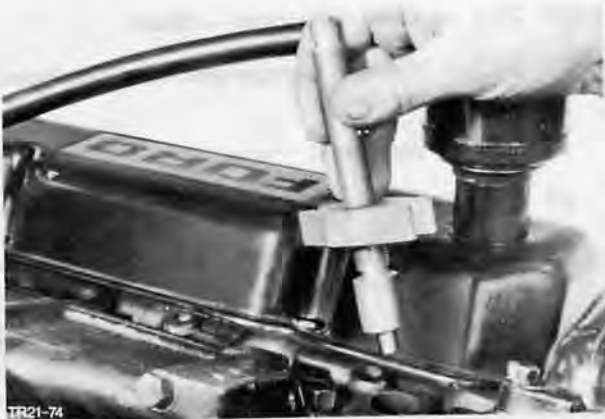
Fig. 8. Install compression tester adaptor into orifice
