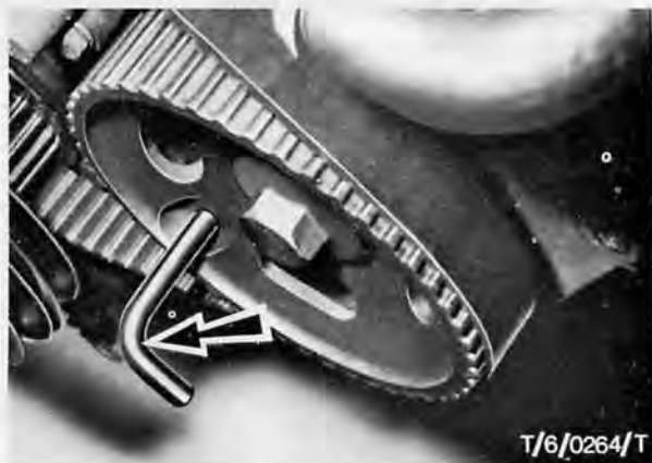
Fig. 10 Timing peg Special Tool No. 21 016
