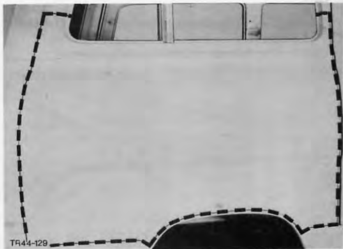
Fig.165. Mark out rear side panel cut line.
