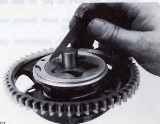
Fig. 173. Measure clearance pump housing/outer rotor
