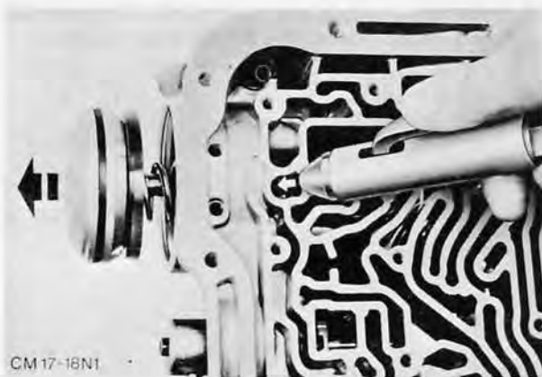
Fig. 78. Use compressed air to remove servo piston
