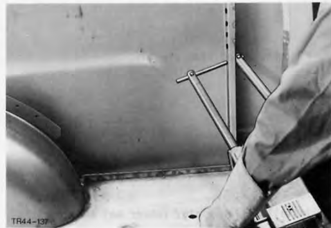
Fig.173. Spot weld side panel at connection to box corner.
