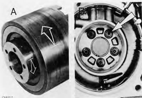
Fig. 103. A - Check operation of one-way clutch B - Clutch inner ring recuring bolts
