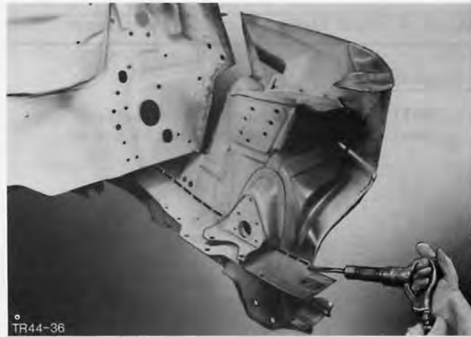
Fig.67. Cut out apron panel (steering box removed).
