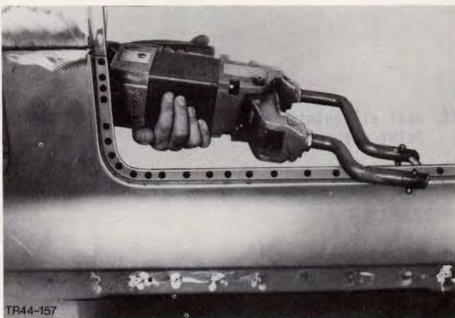
Fig.160. Spot weld inside window panel to window guide.
