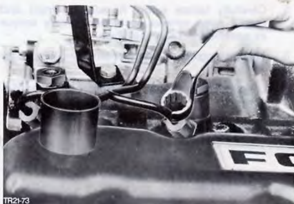
Fig. 101. Remove injector pipes using Special Tool 21-041
