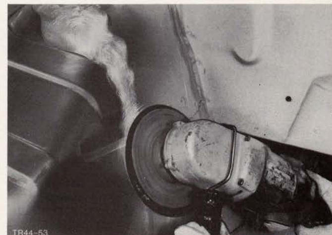
Fig.84. Dress solder-filled locations.
