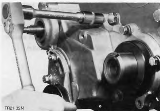
Fig. 149. Centralise timing cover using Special Tool 21-025
