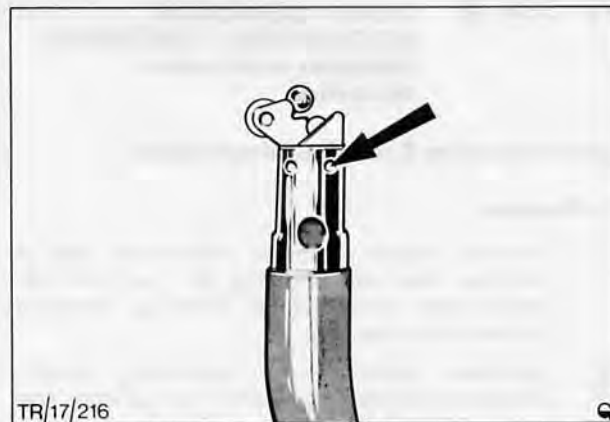
Fig. 9. Selector lever operating cable top linkage
