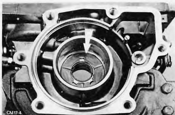
Fig. 110. Thrust washer No. 8
