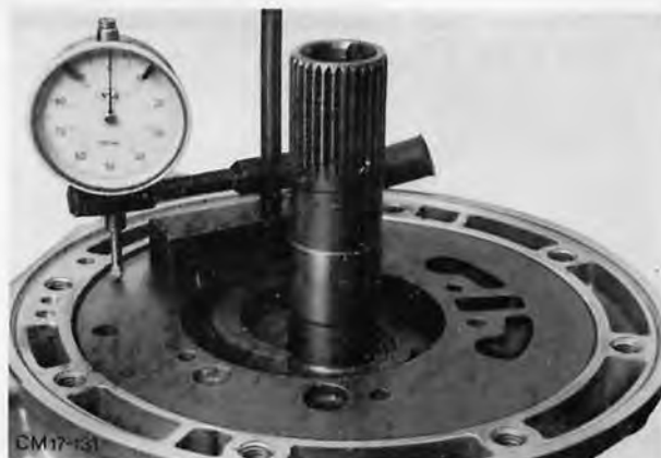
Fig. 74. Set dial gauge on pump body to '0'
