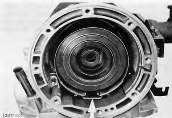
Fig. 76. Brake band with brass clip fitted
