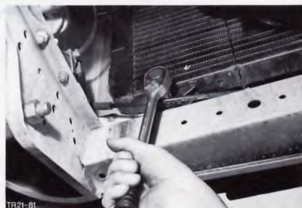
Fig. 156. Fit radiator at bottom location
