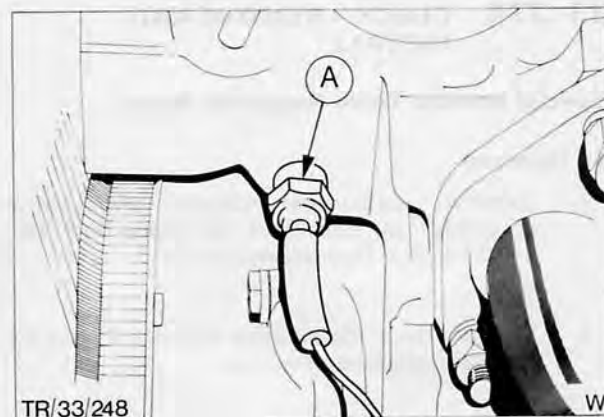
Fig. 69. Sender unit on OHV variants A - Sender unit
