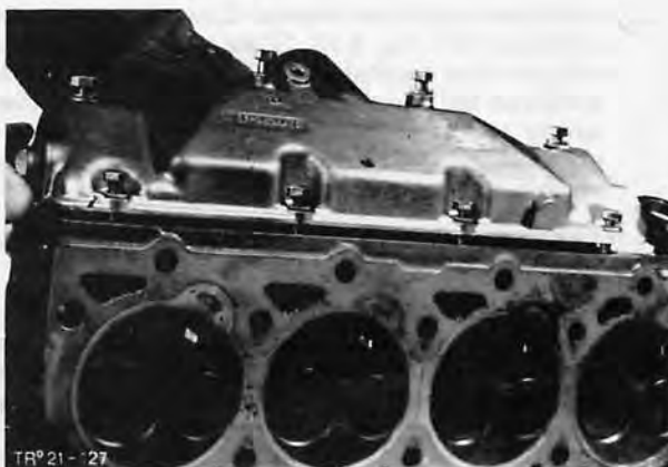
Fig. 113. Remove inlet manifold
