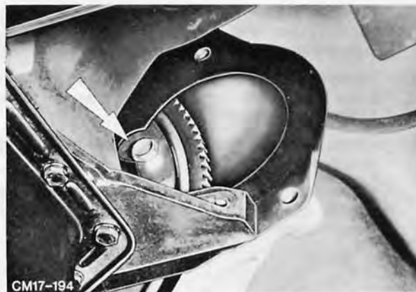
Fig. 24. Remove torque converter drive plate bolt through starter motor aperture
