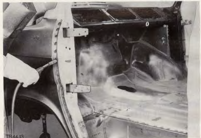
Fig.50. Plug weld fender in area of A pillar.
