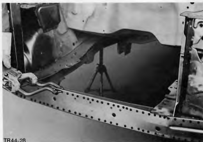
Fig.39. Spot weld new body front lower panel onto crossmember.
