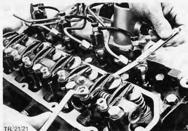
Fig. 112. Adjust valve clearances
