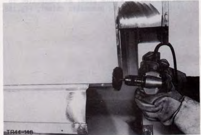
Fig.151. Dress inside window panel spot weld flange.
