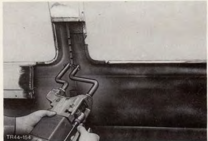
Fig.157. Spot weld front side panel to rear side panel (from inside).
