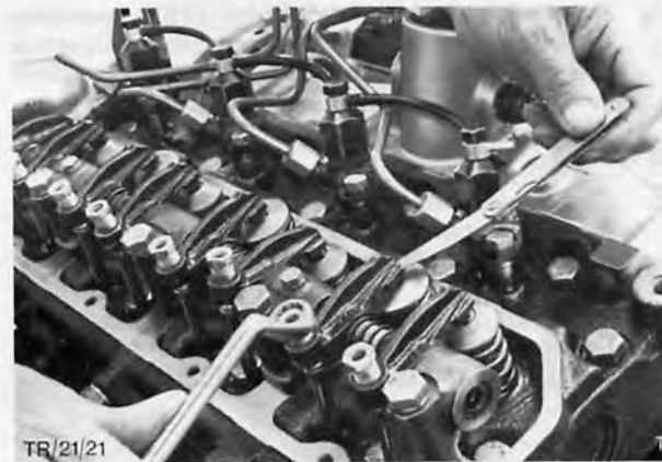
Fig. 107. Adjust valve clearances
