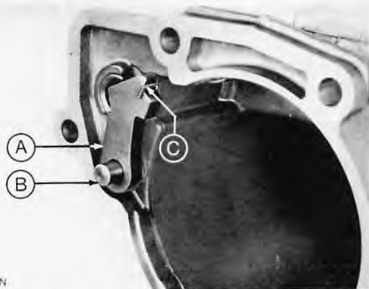
Fig. 124. Extension housing with parking pawl A - Parking pawl B - Dowel C - Return spring
