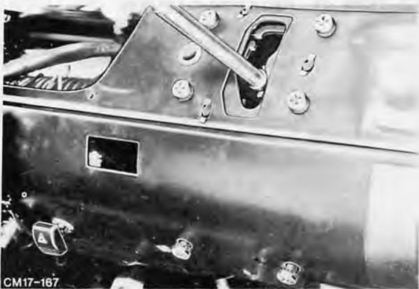
Fig. 40. Remove selector housing bolts
