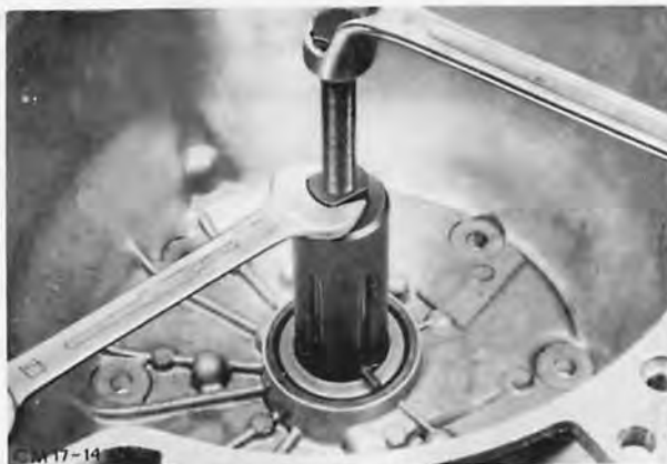
Fig. 71. Remove pump oil seal using Tool 17-011
