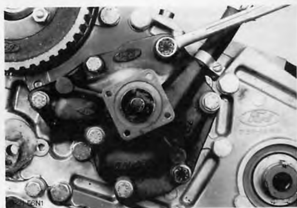
Fig. 51. Remove water pump
