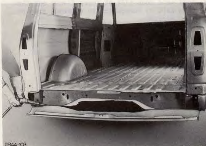
Fig.199. Cut out back panel.
