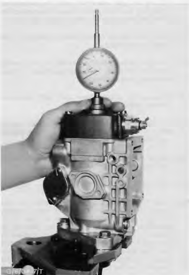
Fig. 36. Measure the dimension 'K'
