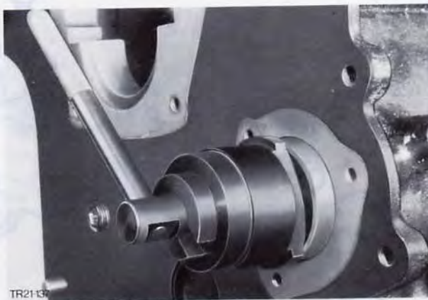
Fig. 126. Back off spindle and fit new bearing bush No. 5
