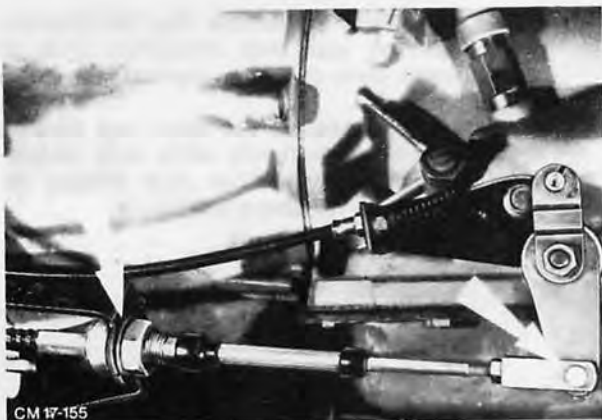
Fig. 20. Remove selector lever cable
