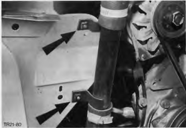
Fig. 14. Unscrew expansion tank connecting pipe
