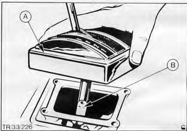
Fig. 50. Removal of selector housing A – Selector housing B – Quadrant lamp
