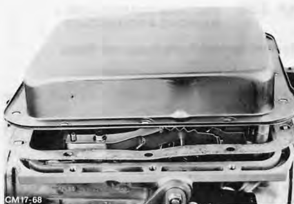
Fig. 139. Fit oil pan with a new gasket
