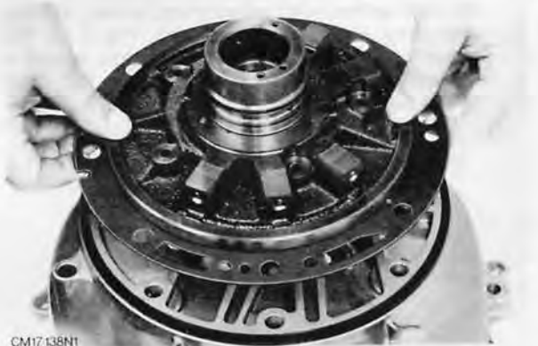
Fig. 120. Align bores in steel plate with hydraulic pump and converter casing
