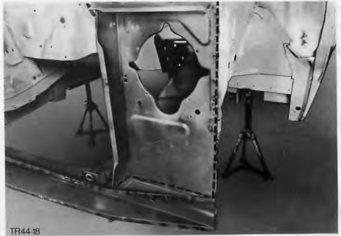
Fig.55. Cut lines for headlamp support plate.
