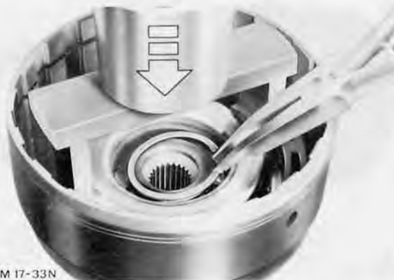
Fig. 94. Compress springs using Tool 17-007
