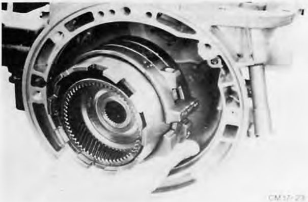
Fig. 82. Remove annulus, brake drum and rear brake band
