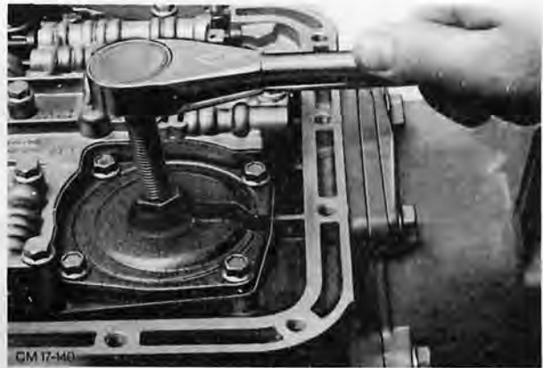
Fig. 134. Adjust adjustment screw with Tool 17-005
