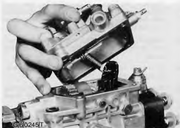
Fig. 16. Lift off the housing cover
