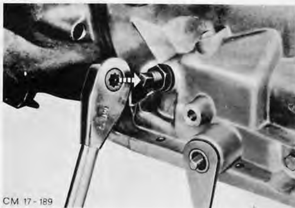
Fig. 123. Adjust front brake band using Tool 17-005
