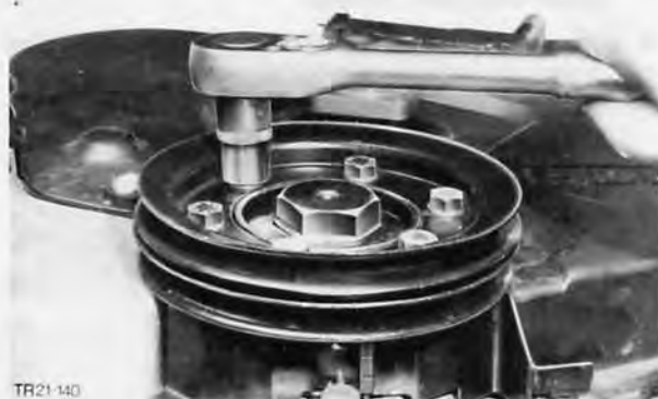
Fig. 143. Remove crankshaft pulley
