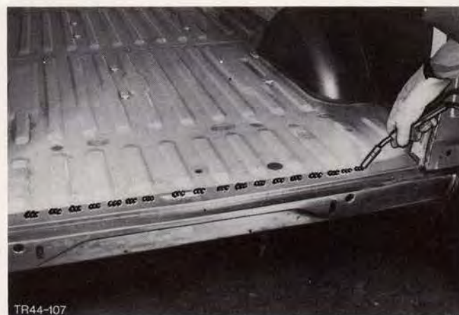
Fig.203. Plug weld new back panel.
