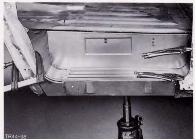
Fig.140. Press in new entrance step with jack and secure with clamps.
