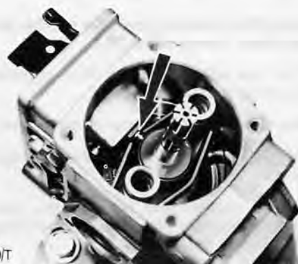
Fig. 38. Engage the control lever ball with the governor control sleeve
