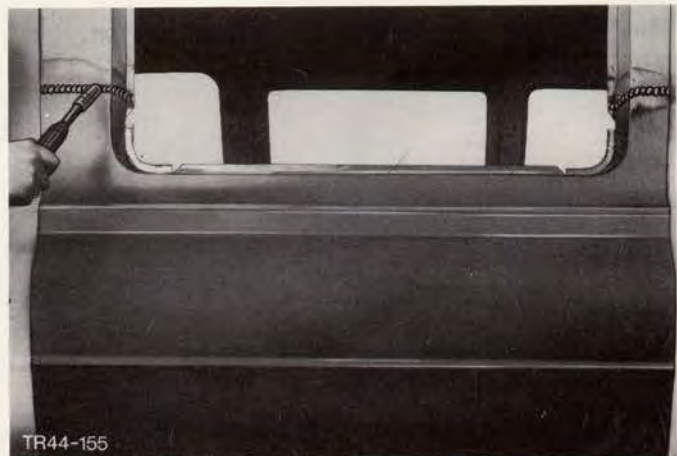
Fig.158. Weld side panel at connection to B and C pillars.
