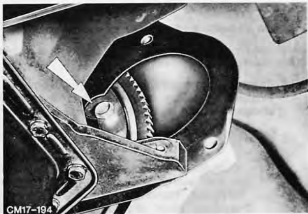
Fig. 31. Torque converter to drive plate bolt
