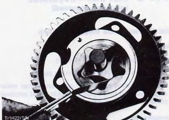
Fig. 172. Measure inner/outer rotor clearance
