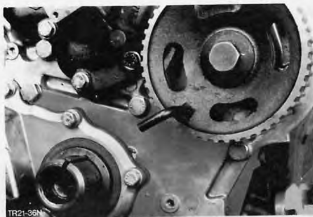
Fig. 50. Lock camshaft toothed belt gear using Special Tool 21-016
