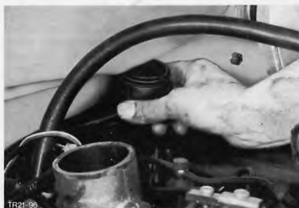
Fig. 109. Fit water outlet connector
