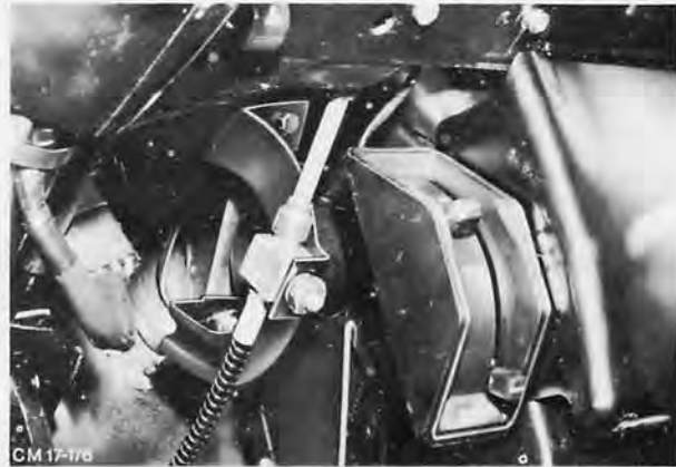
Fig. 52. Disconnect selector cable from heater assembly bracket
