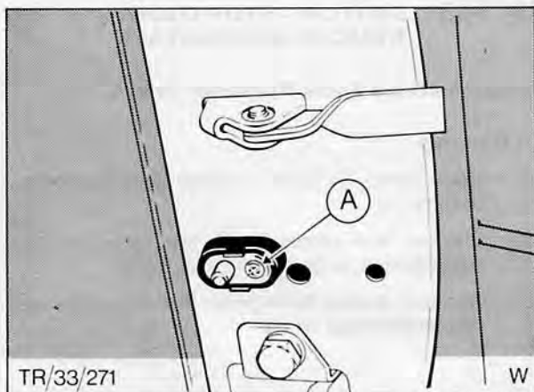
Fig. 81. Courtesy light switch A – Securing screw
