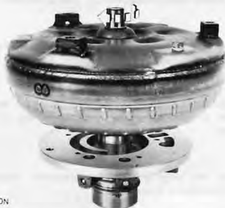
Fig. 13. Check the contact between turbine wheel stator and pump case
