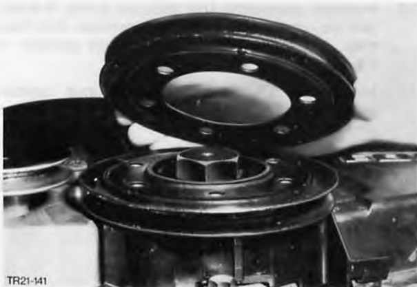
Fig. 138. Fit crankshaft pulley
