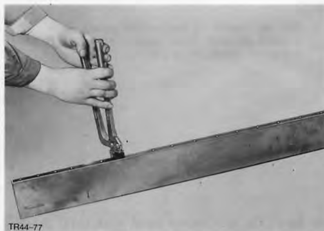
Fig.134. Punch new rocker panel extension at upper spot weld flange.
