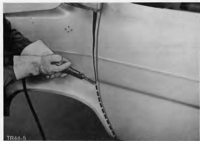
Fig.41. Fender cut line in area of A pillar.
