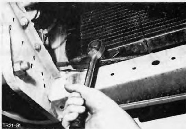
Fig. 36. Fit radiator at bottom location
