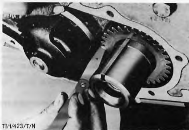
Fig. 78. Check oil pump gear backlash
