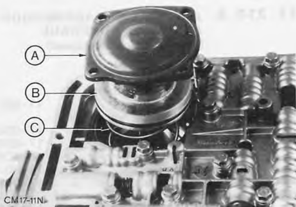
Fig. 69. Rear servo A – Servo cover B – Servo piston C – Spring
