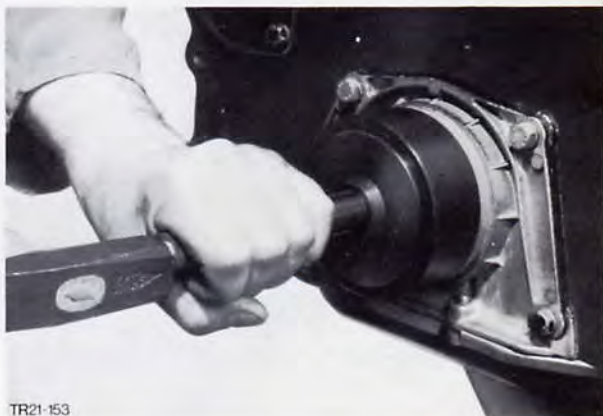
Fig. 158. Drive in oil seal with Special Tool 21-011-A
