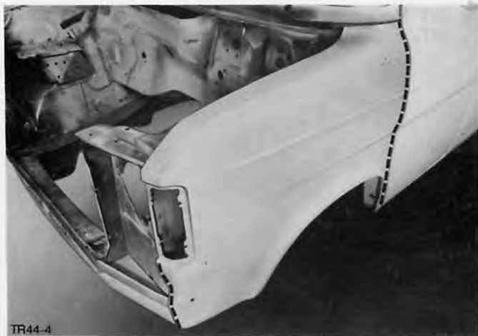
Fig.40. Cut line of fender to be replaced.
