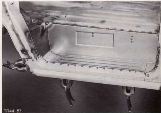
Fig.195. Door sill punched and secured with clamps.
