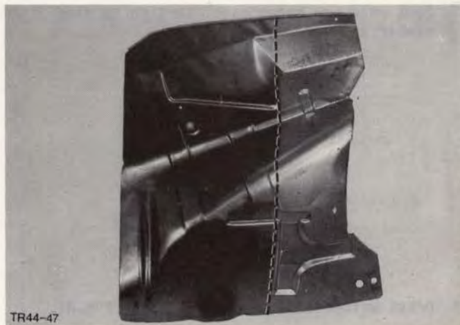
Fig.78. Mark new apron panel.
