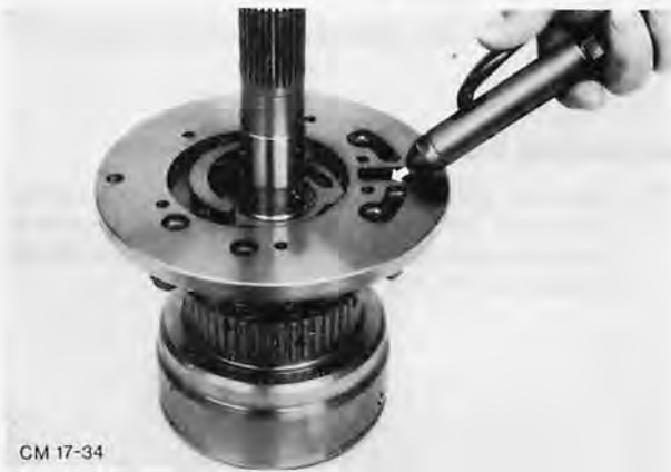
Fig. 95. Remove clutch piston using compressed air
