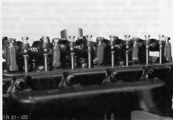
Fig. 106. Insert push rods in rocker arm sockets
