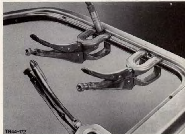
Fig.113. Plug weld window opening flange.
