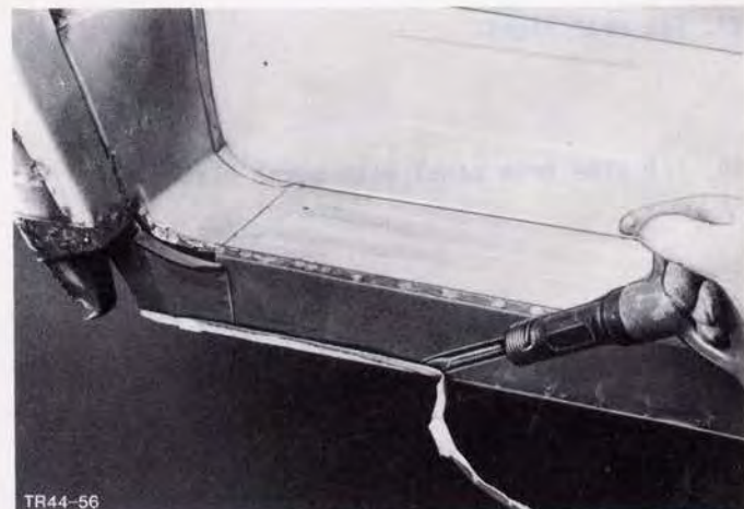
Fig.194. Remove metal remnants.
