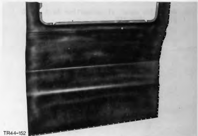
Fig.155. Punch side panel at front and bottom.
