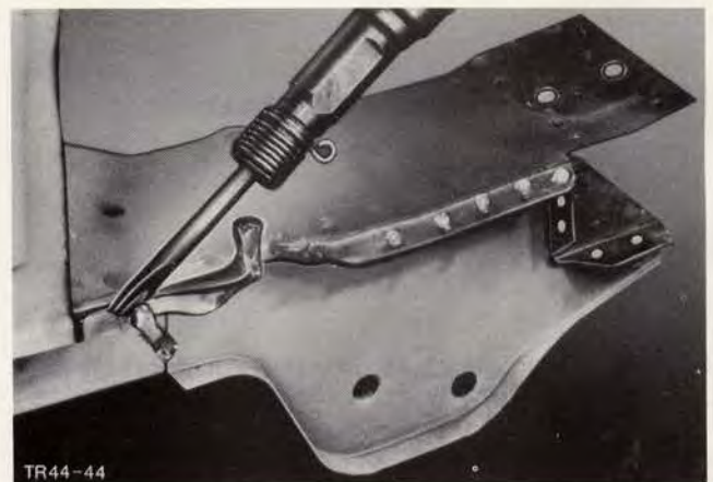
Fig.75. Remove metal remnants.
