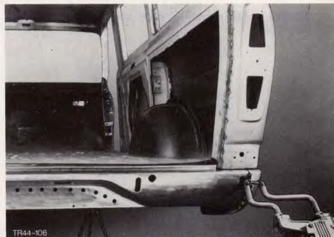
Fig.202. Spot weld new back panel.
