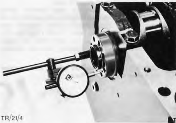
Fig. 69. Check crankshaft end float
