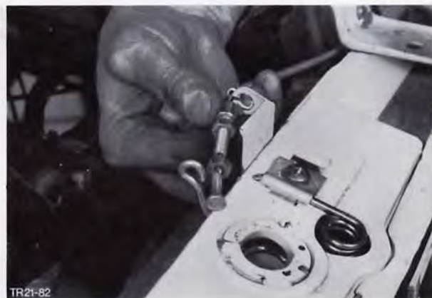
Fig. 155. Fit hood cable
