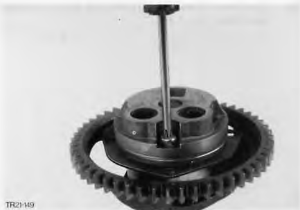
Fig. 171. Fit pump housing cover
