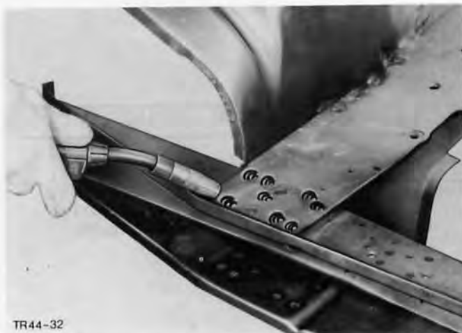
Fig.63. Plug weld crossmember at side members.
