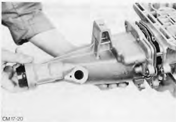
Fig. 79. Remove extension housing
