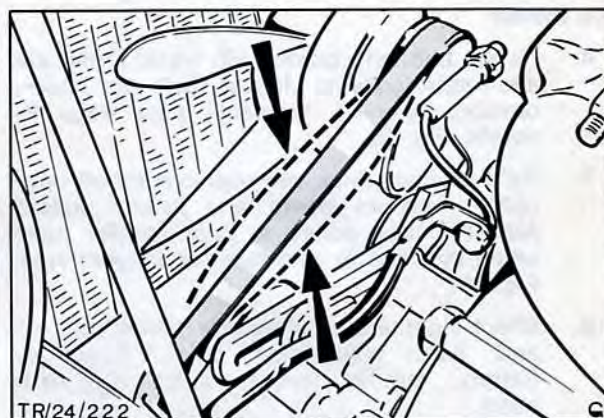
Fig. 34. Fan belt adjustment (Kent engine variant illustrated)
