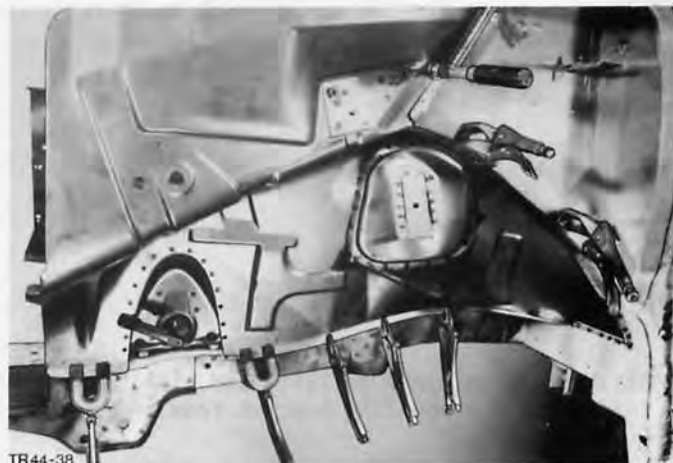
Fig.69. Apron panel punched in area of steering box mounting bracket and fixed with clamps.
