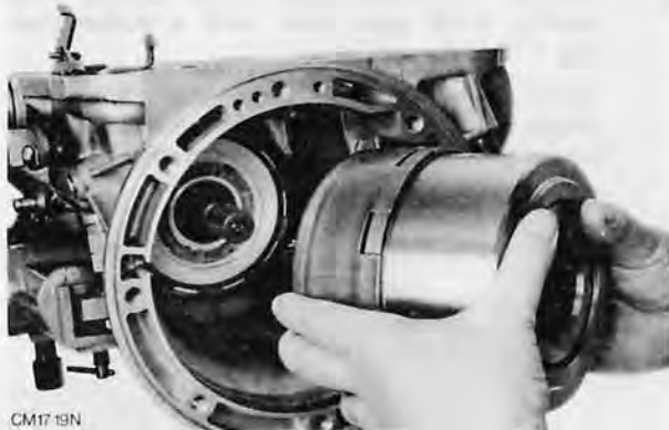
Fig. 116. Insert completed front assembly into transmission housing
