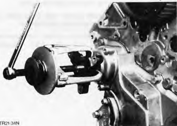
Fig. 147. Remove vacuum pump hub
