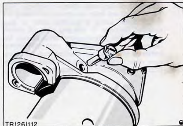
Fig. 68. Removing the eccentric pivot pin
