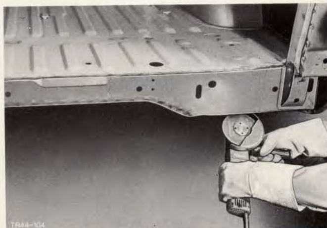
Fig.200. Dress spot weld flanges.
