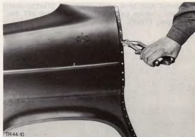
Fig.46. Punch spot weld flange for A pillar on new fender.
