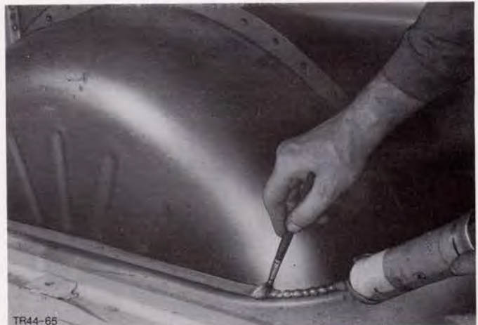
Fig.182. Seal wheel house with metal joint sealer.
