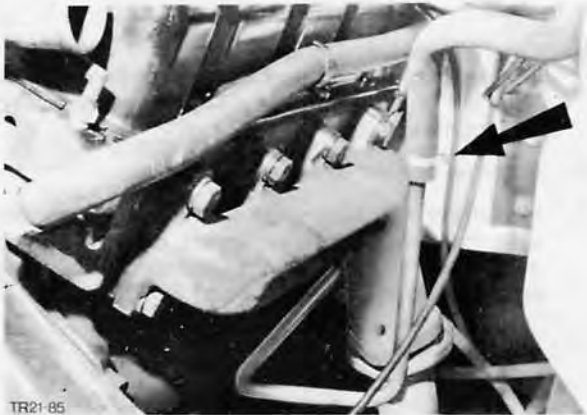
Fig. 31. Slide brake servo vacuum hose on to line and secure
