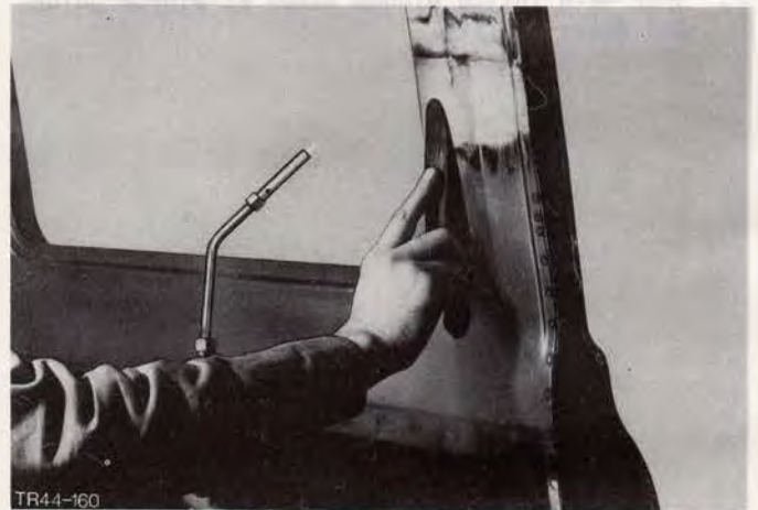
Fig.163. Solder-fill inside window panel joint seam.
