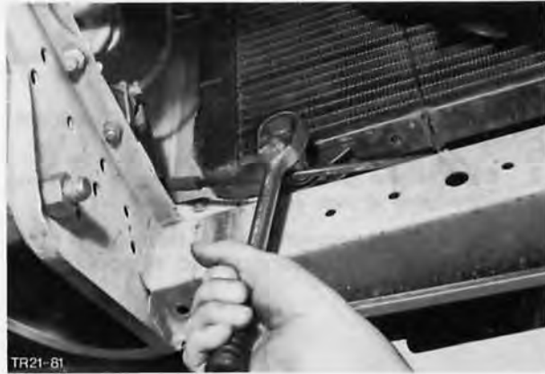
Fig. 15. Remove radiator bottom mounting from crossmember
