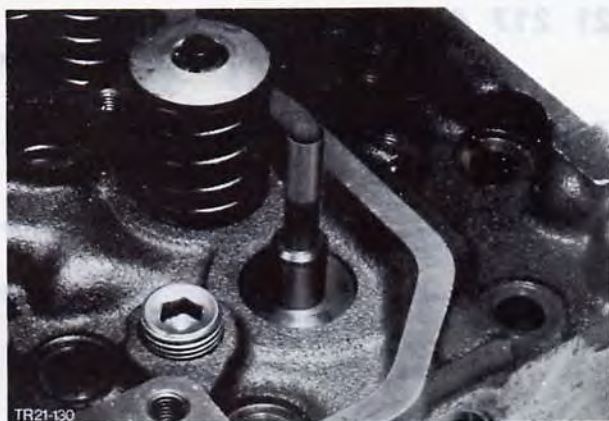
Fig. 116. Cover valve splines with adhesive foil
