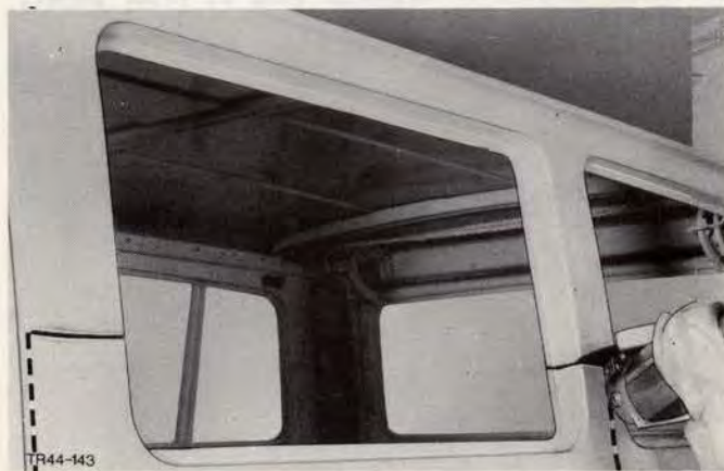
Fig.146. Cut side panel.
