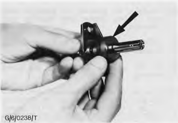
Fig. 37. Fit the control sleeve ground face uppermost
