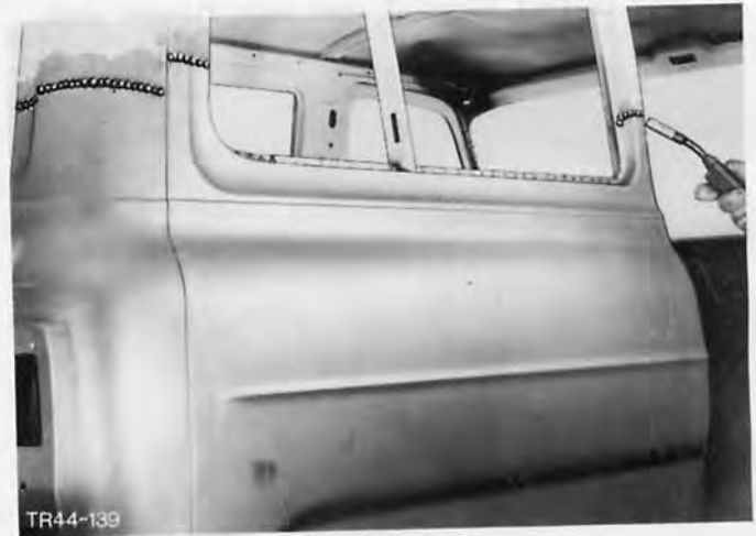
Fig.175. MIG weld side panel joint seams.
