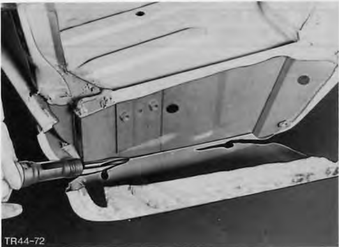
Fig.129. Cut out rear rocker panel.
