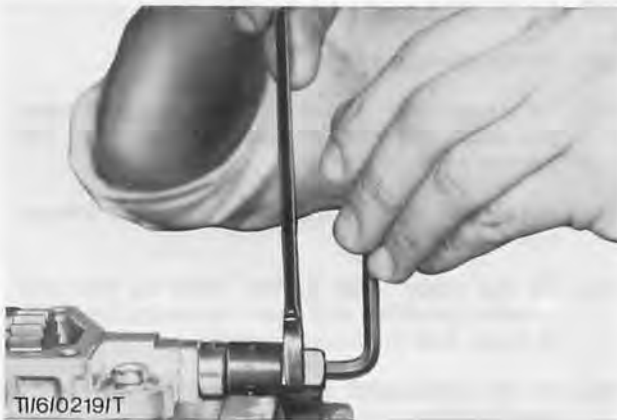
Fig. 42. Using Special Tool No. KDEP 1082 lock the governor shaft
