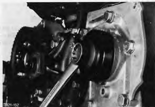
Fig. 134. Fit camshaft oil seal using Special Tool 21-017
