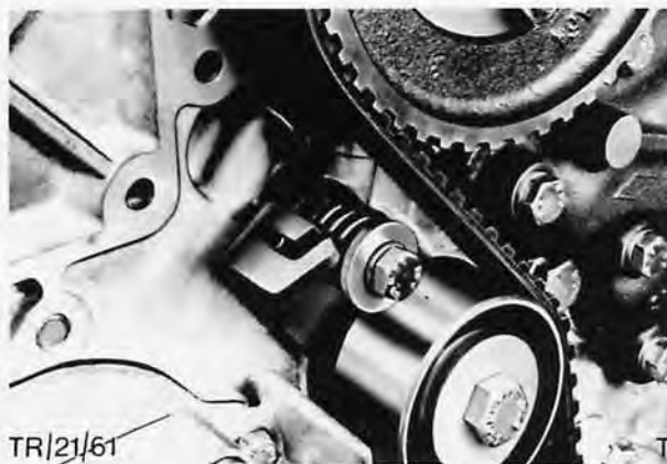
Fig. 145. Slacken toothed belt tensioner
