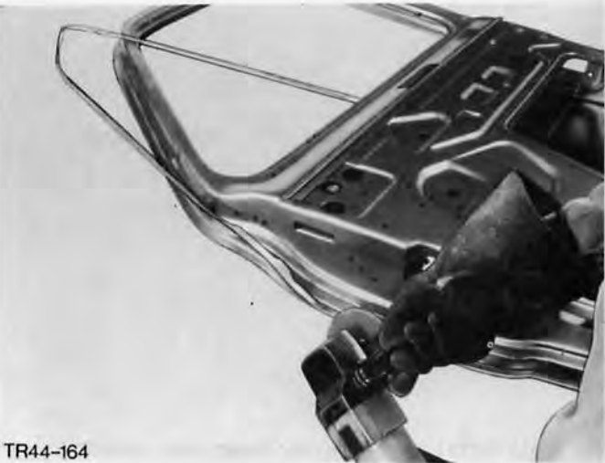
Fig.107. Cut through door surround.
