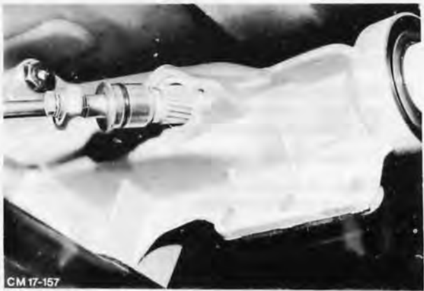
Fig. 147. Remove speedometer gear with shaft
