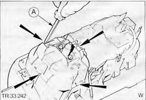
Fig. 63. Securing speed housing A - Screwdriver Screw locations arrowed
