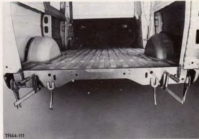
Fig.207. Secure crossmember with clamps.
