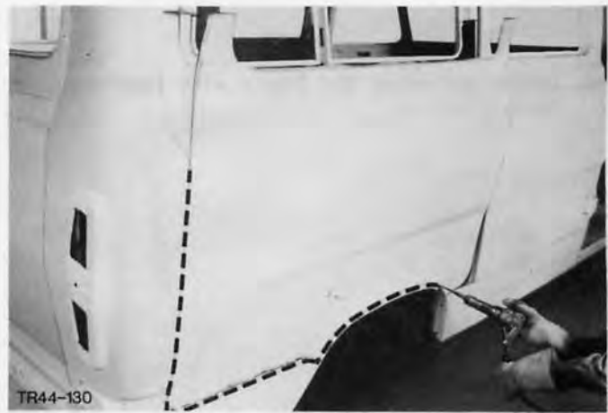
Fig.166. Cut out side panel.
