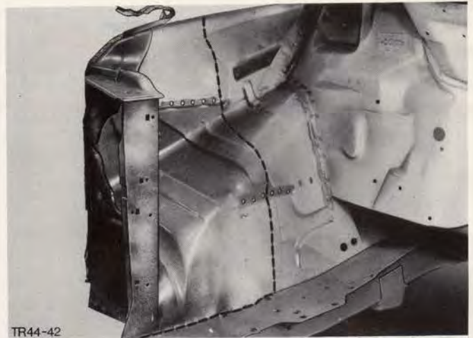
Fig.73. Cut line between side member and apron panel.
