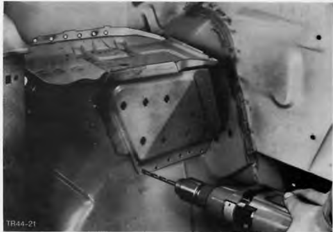
Fig.58. Drill out weld points on battery bracket.
