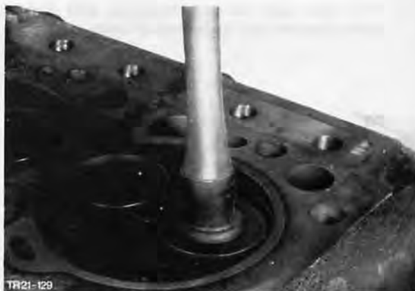
Fig. 115. Grind in valve
