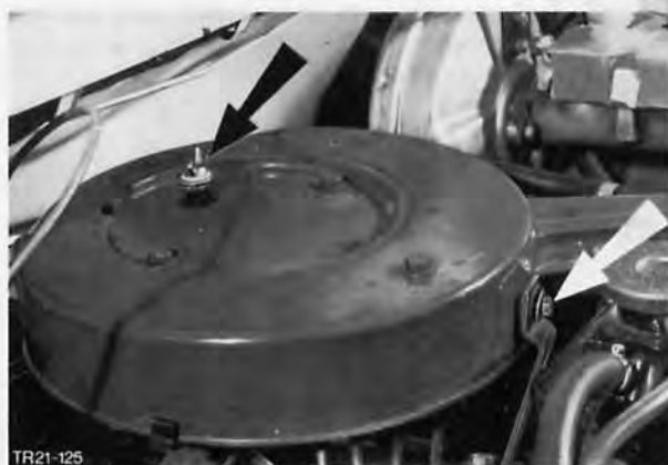
Fig. 110. Fit air cleaner
