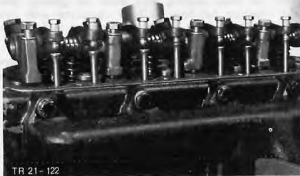
Fig. 93. Fit push rods in rocker arm sockets
