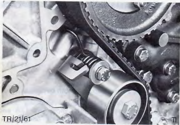
Fig. 131. Slacken toothed belt tensioner
