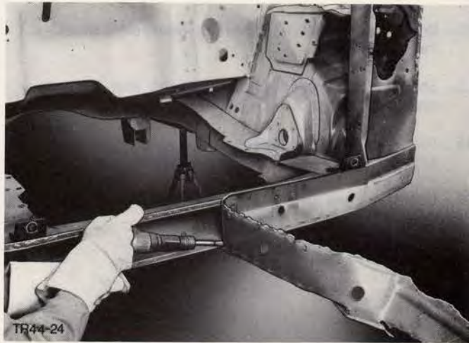
Fig.35. Cut out panel from crossmember.
