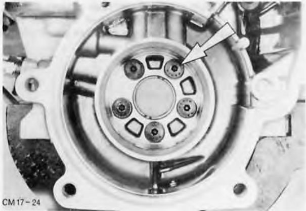
Fig. 83. One-way clutch inner ring Allen screws
