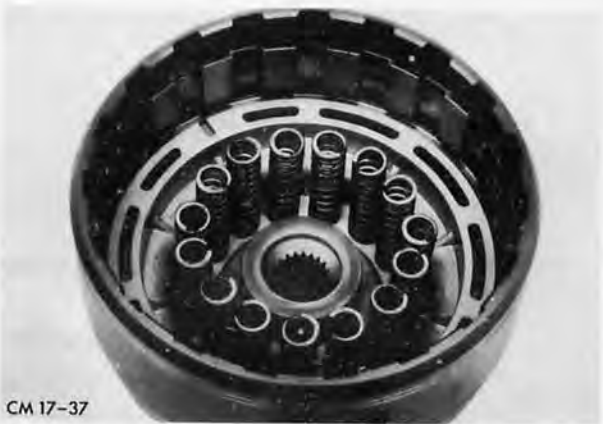
Fig. 96. Clutch body and piston, with springs fitted
