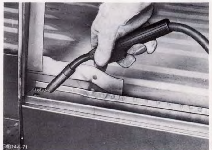
Fig.128. Plug-weld rocker panel.
