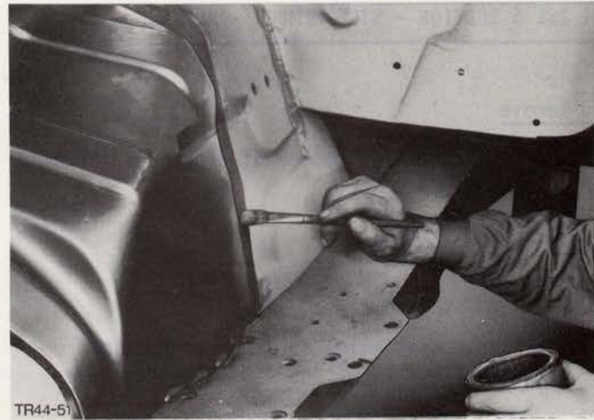
Fig.82. Coat joint seam with tinning paste.
