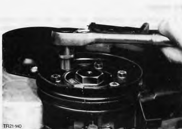
Fig. 137. Remove crankshaft pulley
