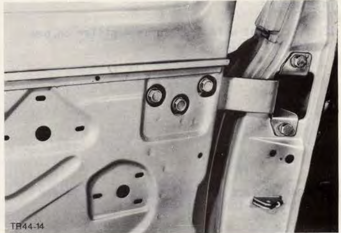
Fig.49. Take off door, by loosening 6 hinge bolts.
