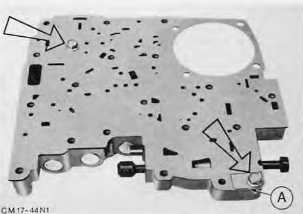
Fig. 128. Cover plate securing bolts A - Identification plate
