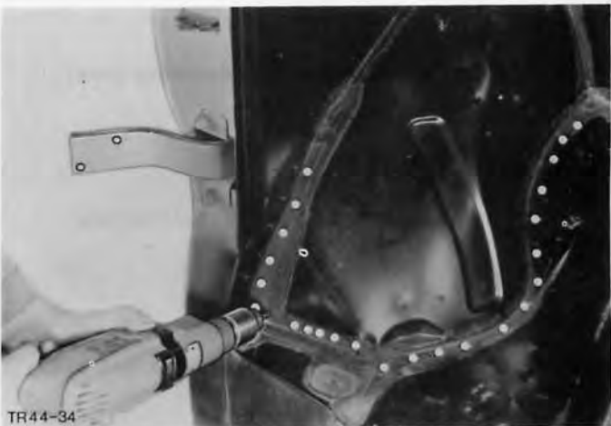
Fig.65. Drill out apron panel from passenger compartment.
