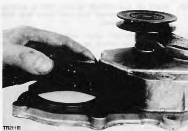
Fig. 79. Fit crankshaft front oil seal to timing cover, using Special Tool 21-025
