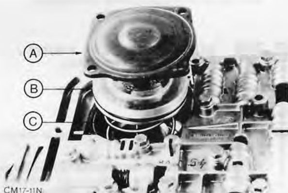
Fig. 140. Rear servo A - Servo cover B - Servo piston C - Spiral spring
