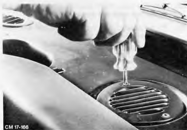
Fig. 39. Remove demister nozzle
