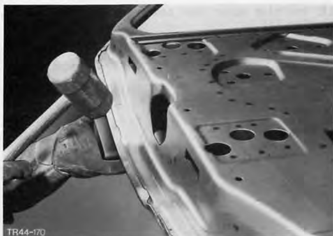
Fig.114. Turn over door flange edges.
