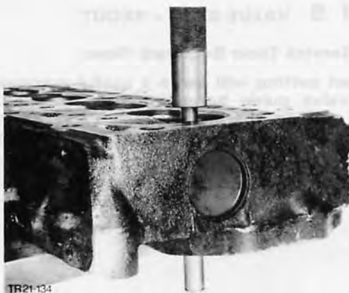
Fig. 122. Remove valve guide
