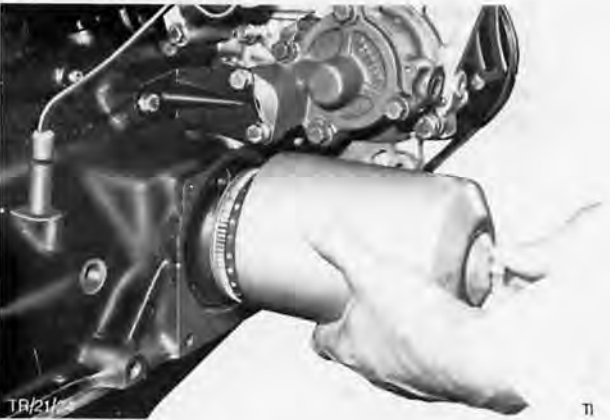
Fig. 96. Fit full-flow oil filter
