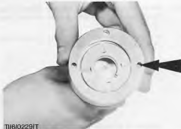
Fig. 28. Hole furthest from inner edge positioned on right when viewed from above
