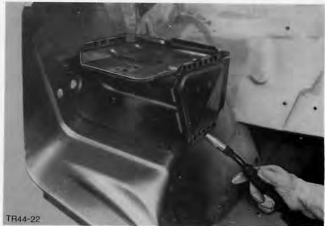
Fig.59. Plug weld battery bracket with holder on apron panel.
