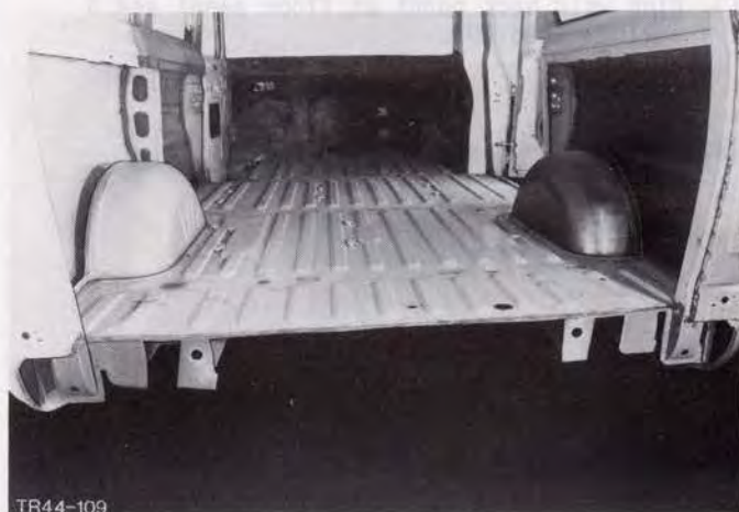
Fig.205. Crossmember cut out.
