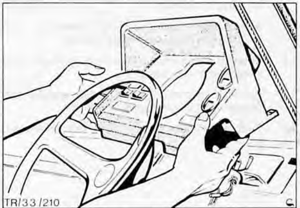
Fig. 18. Guide housing assembly from facia panel
