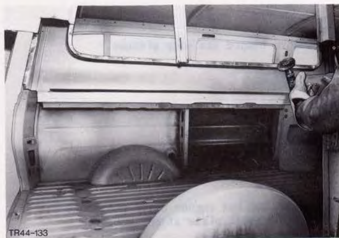
Fig.169. Dress spot weld flanges.
