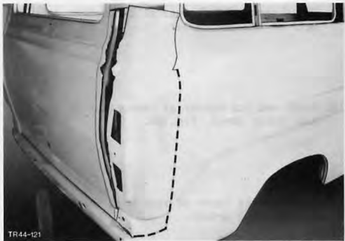
Fig.184. Cut out box corner.
