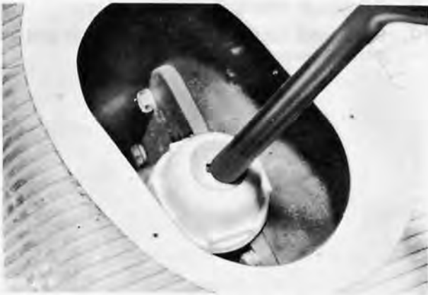
Fig. 21. Remove transmission gearshift lever nut
