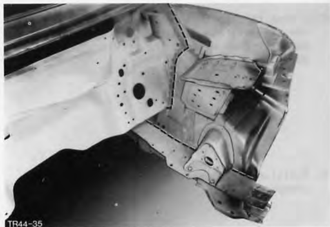
Fig.66. Mark apron panel cut line.
