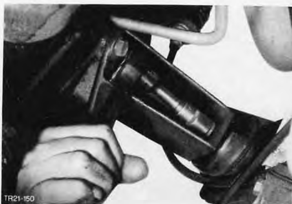
Fig. 175. Remove nuts from engine mounting rubber insulator
