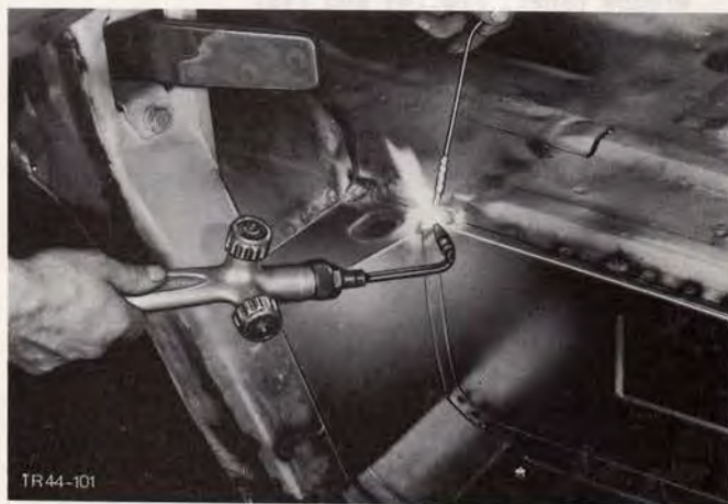
Fig.143. Braze corners of entrance step at floor panel.
