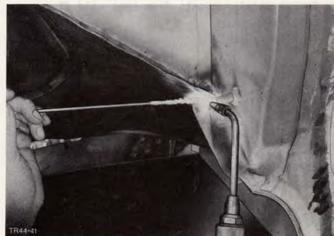
Fig.72. Braze apron panel at the corners.
