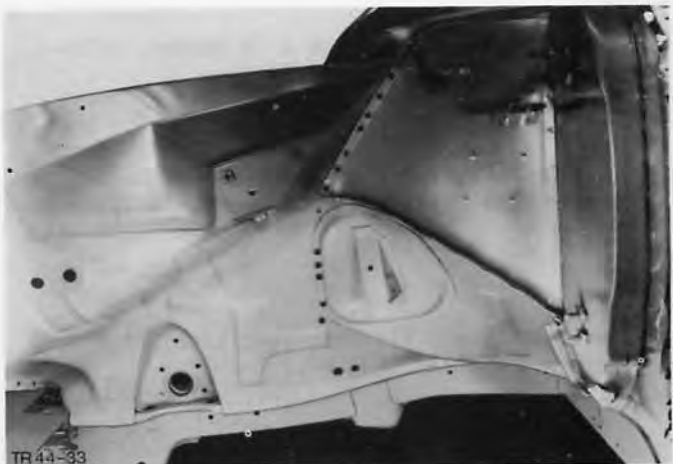
Fig.64. Drill out apron panel at outside connecting points.
