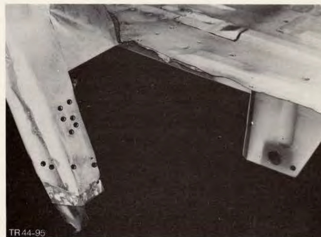
Fig.137. Metal remnants cut out from A pillar reinforcement.
