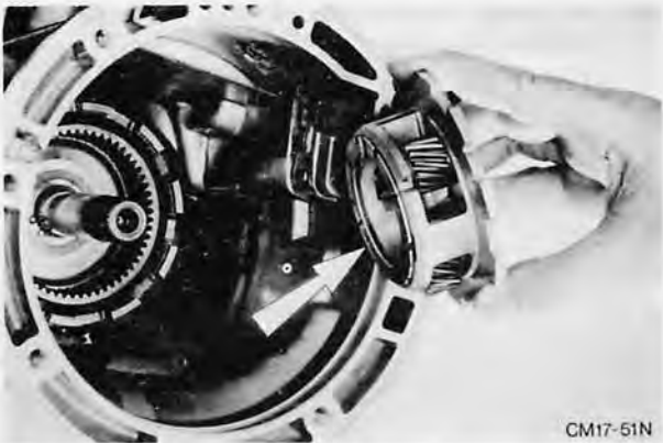
Fig. 113. Insert thrust washer No. 5 together with planet carrier into transmission housing
