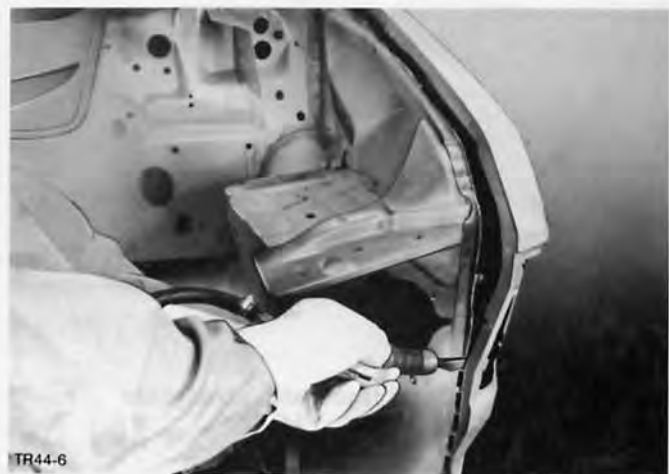
Fig.42. Cut line in area of apron panel.
