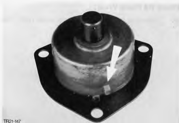
Fig. 169. Slide oil pump retainer plate behind pump housing lug
