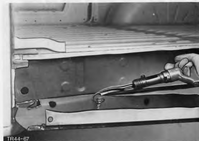
Fig.124. Cut out rocker panel.
