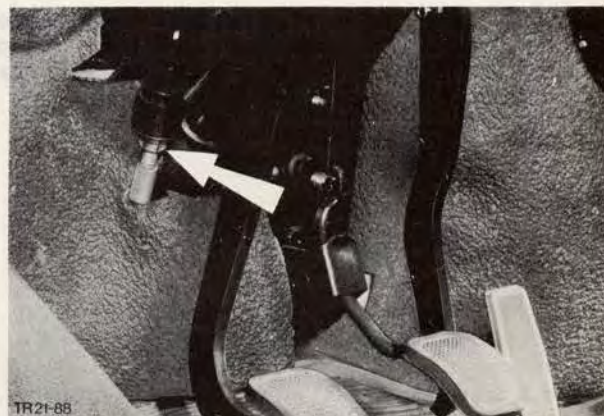
Fig. 22. Remove clutch cable from pedal bracket
