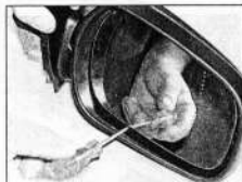
18.6a To remove the mirror glass, spread the ends of the internal spring clip apart to release the glass...
