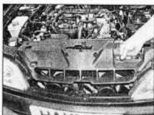
22.4 Lift up the air inlet duct and withdraw the grille from the front body panel
