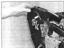
6.24 Removing the timing belt upper cover ...
