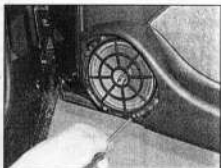
12.4a Undo the loudspeaker retaining screws ...
