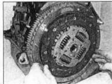
4.13 Fit the friction plate so that its spring hub assembly faces away from the flywheel
