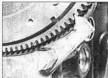
5.2 Use a fabricated tool similar to this to lock the flywheel ring gear and prevent crankshaft rotation
