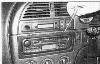
17.2 Carefully prise off the radio/cassette player trim plate
