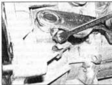
5.3a Draw out the release fork retaining pin using a nut screwed onto the threaded end ...
