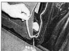
13.6 Carefully release the plastic sealing sheet from the adhesive bead on the front door
