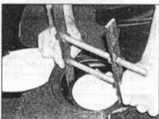
8.6a Using a home made tool, slacken the fuel pump locking ring ...
