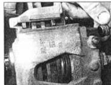
4.18 Remove the guide pin bolt dust caps ...
