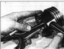
14.14b . . . and withdraw the gudgeon pin
