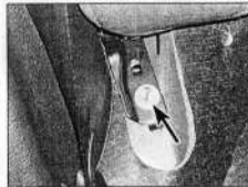
24.10 Rear seat back hinge front retaining bolt (arrowed)
