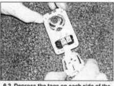
6.3 Depress the tags on each side of the bulbholder and withdraw the bulbholder from the light unit
