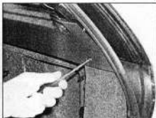
26.42c ... and at the rear of the parcel shelf support - Estate models
