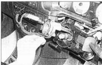
22.17b ... and withdraw the rotary connector from the steering column
