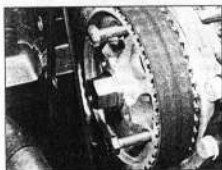
5.14 Bolts inserted through timing holes in injection pump sprocket
