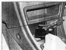
27.4a Remove the ashtray from the front of the centre console ...
