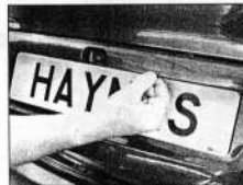
16.10a Release the number plate lamp trim moulding retaining clips ...
