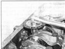
19.29b ... and, on 2.0 litre engines, additionally through the specified angle
