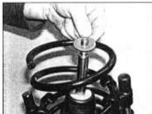
5.8e Place the flat washer in position . . .
