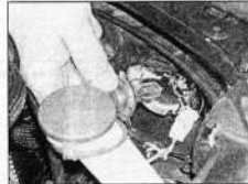
5.4b ... and withdraw the headlight bulb
