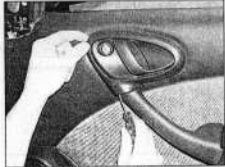
12.1 Carefully prise out the base of the front door interior handle trim surround
