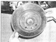
7.8b ... and remove the front brake disc
