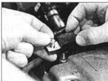
3.8a Remove radio suppressor from the right-hand end of the coil module ...
