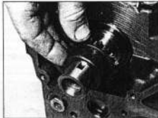
12.5b ... then slide off the drive sprocket ...
