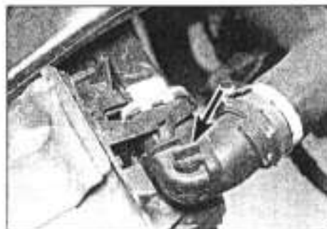
27.4a Radiator bleed screw (arrowed) – 1.4 litre engines
