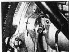
5.16a Unscrewing an injection pump front mounting nut – Bosch pump
