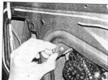
14.13a Undo the nut securing the upper edge of the regulator to the door ...
