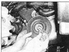
5.6 Removing the crankshaft pulley – 2.0 litre engines
