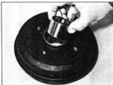
12.9a Locate the bearing in the hub ...
