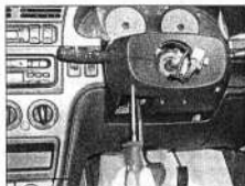
18.3a Unscrew the three lower steering column shroud securing screws ...
