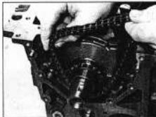
12.5a Remove the oil pump drive chain ...
