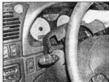
28.11b ... then unclip and lift off the upper shroud, and remove the lower shroud
