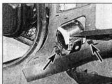
26.54 Lift the lower trim panel upwards to disengage the two lower locating lugs (arrowed)
