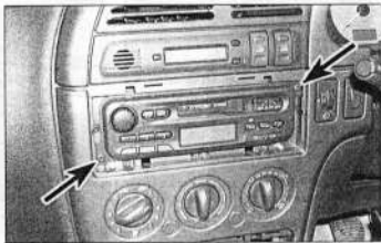
17.3 Undo the two screws (arrowed) securing the radio/cassette player to the fascia
