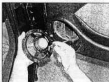
18.3b ... then withdraw the loudspeaker and disconnect the wiring plug
