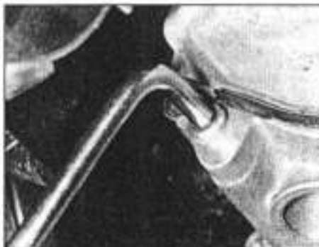
23.5 Using a square-section wrench to unscrew the transmission filler/level plug – MA transmission
