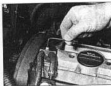
4.7a Remove the two Allen bolts ...
