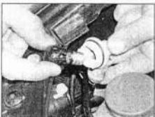
5.13 The bulb is a bayonet fit in the bulbholder
