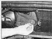
10.22a Unscrew the nuts securing the heater assembly to the bulkhead ...
