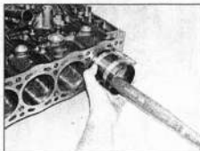
20.19c Tap the assembly into the cylinder bore until the piston crown is flush with the top of the block
