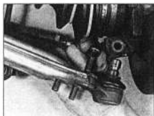
7.5a Remove the three retaining bolts ...
