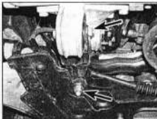
5.26 Undo the nuts and bolts (arrowed) and remove the rear engine mounting connecting link
