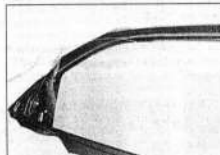
14.23b ... then remove the glass from the outside of the door, with the rear corner uppermost
