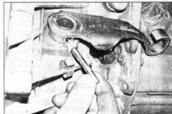
5.3b ... then remove the retaining pin from the fork
