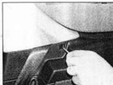
26.42b ... and the upper screws at the front ...
