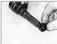
12.12a Locate a new upper seal on the body of each injector ...
