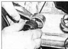
2.2a Release the clutch inner cable end fitting from the support bracket or release lever ...
