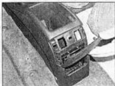
27.2b ... then carefully prise off the trim cover or switch surround
