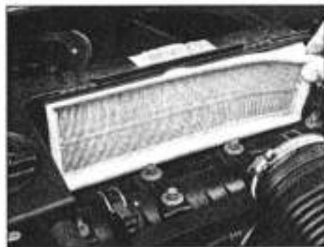
18.9d ... and withdraw the filter element
