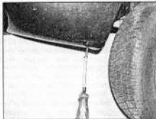
7.5 Undo the screw each side securing the splash shields and/or the wheelarch liner to the bumper
