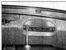
26.58b ... then undo the two screws and remove the handle
