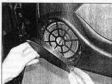
12.3 Carefully prise off the loudspeaker grille from the front door trim panel
