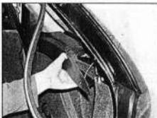
26.44a Release the parcel shelf support from its location ...
