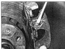
4.17 Carefully prise out the pad retaining spring from the caliper - ATE/Teves caliper
