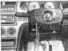
4.7a Undo the two upper screws ...
