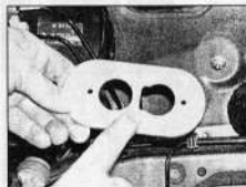
10.18b ... noting the orientation of the D-shaped cut-out
