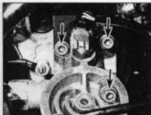
8.9a Unscrew the three securing bolts (arrowed) ...
