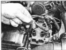
3.4 Disconnect the HT leads from the coil terminals
