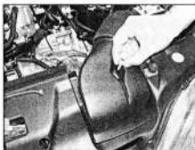
4.11 Undo the bolt securing the front of the air inlet duct to the front body panel
