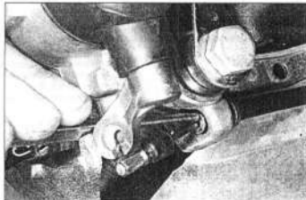
11.3b ... then tap the outer cable out from the caliper body
