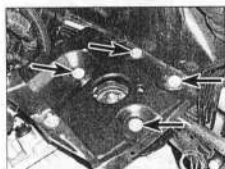
5.5 Undo the four battery mounting plate retaining bolts (arrowed) ...
