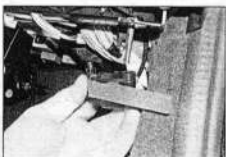
9.2 Unscrew the bonnet release lever securing nut, and withdraw the lever from the pivot stud
