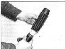
5.8b Fit the piston dust cover . . .
