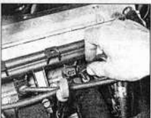
13.54 Disconnect the wiring connectors from the fuel injectors – 1.8 litre (16-valve) engines
