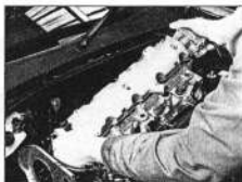
13.22 Removing the cylinder head
