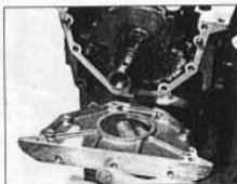
11.15 Removing the oil seal carrier from the block - XU series engines
