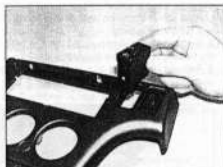
4.19b ... and remove the relevant switch from the centre panel
