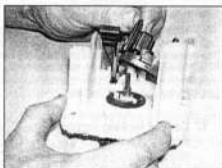
16.15b ... then lift off the end cap ...
