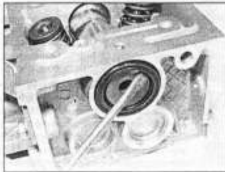
10.9a ... prise out the oil seal...
