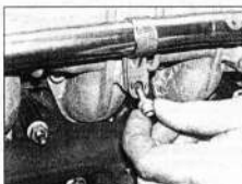
3.39 On 2.0 litre diesel engines, undo the bolts securing the EGR pipe support clips to the inlet manifold ...
