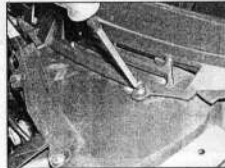
14.3 Undo the scuttle cover panel retaining screws
