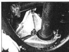
2.12a On the right-hand driveshaft, slacken the two intermediate bearing retaining bolt nuts ...
