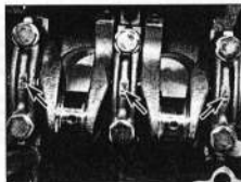
12.6 Main bearing cap identification markings (arrowed)
