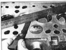
8.9 Checking the cylinder head gasket surface for distortion
