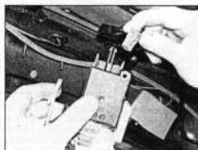
16.12b ... and the central locking motor wiring connector
