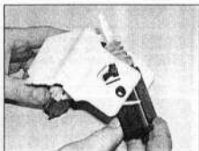
16.14b ... then twist the motor through 90° to release the side attachment lug
