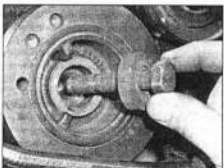
5.3a Removing the crankshaft pulley retaining bolt
