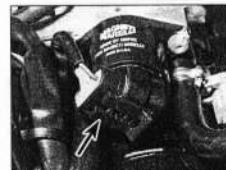
14.7 Disconnect the wiring connector from the idle speed stepper motor ...
