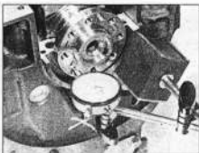
14.2 Checking crankshaft endfloat using a dial gauge
