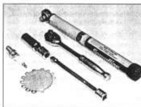
22.7 Tools required for spark plug removal, gap adjustment and refitting
