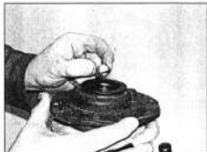
5.8k ... then fit and tighten the piston rod nut
