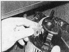
10.32b ... pull the rubber wiring grommet away ...
