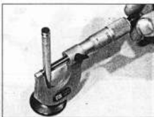
9.12 Measuring a valve stem diameter
