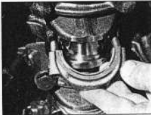
10.5 Removing a big-end bearing cap and shell
