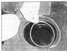
8.7b ... and recover the sealing O-ring
