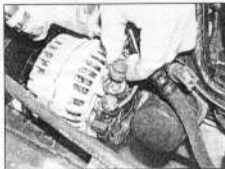
8.3a Lift off the rubber covers ...
