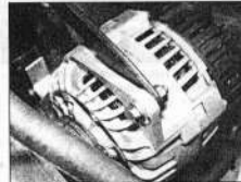
8.4 Slacken and remove the alternator upper mounting bolt ...
