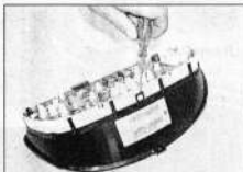
9.4a To remove the instrument panel lens hood, lift the two retaining tags ...
