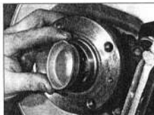
11.14d ... then fit the new hub cap
