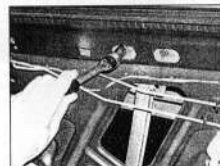
14.29 ... and the two bolts securing the top of the channel to the door
