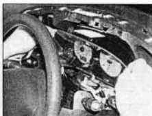
9.2b ... and withdraw the panel slightly from the fascia
