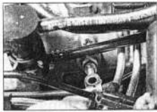
2.2c ... and the interconnecting wire from the glow plug
