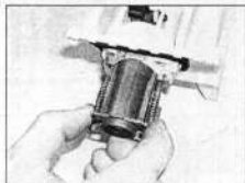
16.16a Withdraw the lock cylinder from the housing ...
