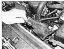
4.4 Disconnect the wiring plug from the accelerator pedal position sensor
