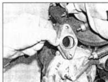
3.41b ... then withdraw the valve and pipe assembly and recover the gasket at the EGR pipe flange
