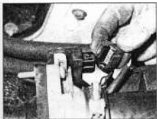
13.15 Disconnect the throttle potentiometer wiring connector – 1.6 litre engines
