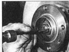
11.6b ... then tap up the rear hub staking using a hammer and suitable punch
