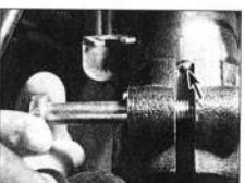
2.16 Ensure the swivel hub clamp is aligned with the lug (arrowed) on the strut prior to inserting the clamp bolt
