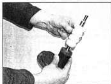
5.8a Pull the piston rod out as far as it will go and fit the damper stop
