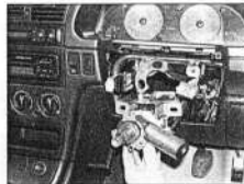
18.11b ... and withdraw the steering column from the vehicle
