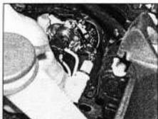
5.9 Twist the sidelight bulbholder anti-clockwise and withdraw it from the headlight unit
