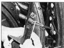
12.2c On manual door mirrors, lift the mirror control stalk plastic catch ...
