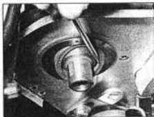
16.12 Removing the camshaft right-hand oil seal
