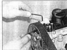
13.20 Insert feeler blades bent through 90° through the sprocket to measure the camshaft position sensor air gap
