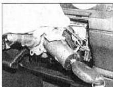
19.3b ... then remove the lock retaining screw and washer from the side of the lock
