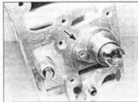
10.8 Undo the retaining bolt, and remove the camshaft thrust fork (arrowed)...
