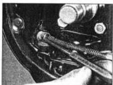
19.6 On drum brake models, drive the outer cable from the brake backplate
