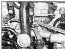
11.9a Using two spanners, unscrew the fuel pipe unions at the accumulator rail ...
