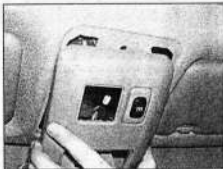
4.34b ... then lower the console from the roof ...
