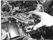
3.5 Undo the four retaining screws and remove the HT ignition coil from its mounting bracket
