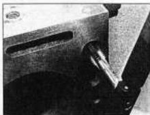
13.8 Cleaning a cylinder block threaded hole using a suitable tap
