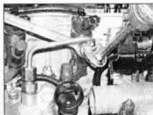
11.15 Using a torque wrench and crow-foot adaptor, tighten the fuel pipe union nuts
