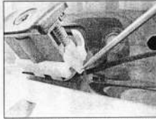
16.11 Depress the tabs on each side of the lock housing
