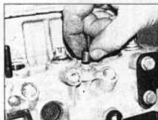
12.7 Recover the injector clamp locating dowel from the cylinder head
