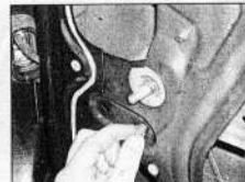
14.30a Undo the two nuts securing the regulator to the door ...
