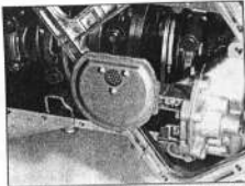
14.10b ... then refit the plate to the base of the cylinder block/crankcase
