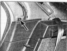
26.27a Undo the wheelarch trim panel upper retaining screw (arrowed) ...
