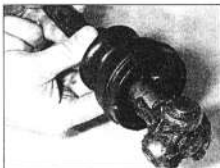
3.42b Slide the gaiter off the end of the driveshaft...
