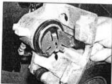
4.35b ... and, where fitted, recover the shim from the caliper piston - Lucas caliper
