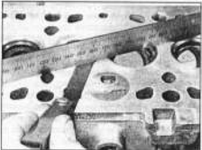
8.6 Checking the cylinder head gasket surface for distortion
