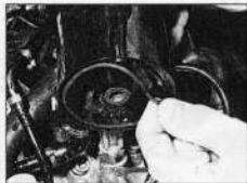
8.8c ... and recover the O-ring
