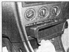
27.4b ... then prise free and remove the oddments tray
