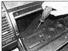
28.22b ... lower securing screws ...
