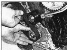
8.15a Retain the timing belt on the crankshaft sprocket and feed it around the idler roller ...
