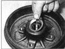
12.11a Fit the new oil seal seating ring ...
