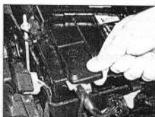
4.3 With the quick-release type of battery positive terminal fixing, lift the cover to release the clamp
