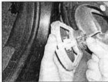
12.16b ... then withdraw the speaker and disconnect the wiring
