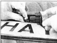
5.35b ... and disconnect the wiring connector
