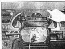
4.8a Unclip and lift off the upper shroud ...
