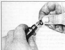
13.57 Fit new O-rings to the injectors before refitting – 1.8 litre (16-valve) engines
