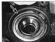
3.3 Front hub bearing retaining circlip (arrowed)
