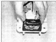
16.13b ... and remove the trim moulding from the lock cylinder
