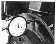
7.4 Checking disc run-out using a dial gauge
