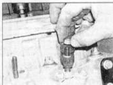
12.5a Unscrew the injector clamp retaining nut...
