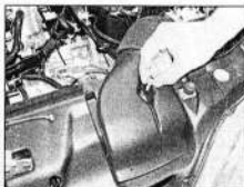
22.2 Undo the bolt securing the air inlet duct to the front body panel
