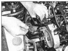
18.11 Removing the right-hand engine mounting upper bracket and rubber buffer plate
