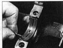
12.9 Remove the upper main bearing shells from the cylinder block/crankcase, and store them with their lower shells
