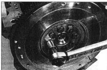
18.12 ... then refit the flywheel, and tighten the bolts to the specified torque
