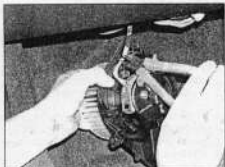
10.32a Cut the cable tie securing the wiring to the motor cover ...
