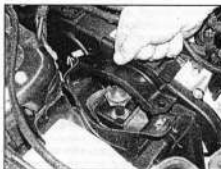
5.27a Remove the right-hand engine mounting curved retaining plate ...
