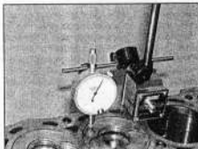
6.20 Measuring piston protrusion
