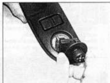
4.22b ... and remove the switch from the panel
