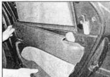
12.20 Pull the trim panel outwards, then lift it up and remove it from the door
