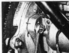
5.16a Unscrewing an injection pump front mounting nut – Bosch pump
