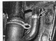
10.6a Disconnect the main breather hose (arrowed) from the filler neck ...
