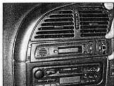
4.14b ... and remove the surround from the facia upper switches
