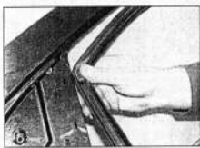
14.22a Release the rear door window glass weatherstrip from the upper corners of the window aperture ...
