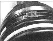
3.21j ... then fold the buckle firmly down onto the clip to secure the clip in position
