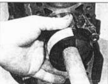
19.20 Tap the piston into the bore using a hammer handle
