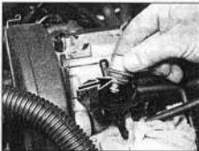
13.61b ... and ease the regulator from the fuel rail. Check the sealing ring condition (arrowed) before refitting – 1.8 litre (16-valve) engines
