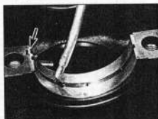
16.39 Ensure each bearing shell tab is located (arrowed), and apply clean oil – TU series aluminium block engines
