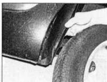
7.6a Ease the wheelarch liner forward for access ...
