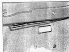
6.13 Prise the light unit from its location in the luggage compartment
