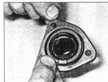
4.27 Fit a new O-ring/gasket (as applicable) to the rear of the guide sleeve
