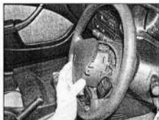
22.8 Gently pull the air bag unit from the centre of the steering wheel
