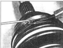
3.21g Fit the outer gaiter retaining clip and, using a hook fabricated out of welding rod and a pair of pliers, pull the clip tightly to remove all slack
