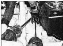
2.2b ... then depress the retaining tabs and release the outer cable from the transmission
