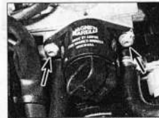
14.8 ... then remove the two screws and withdraw the motor from the throttle housing – 1.4 litre engines
