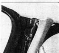
2 Release the upper trim panel from the pillar, and disengage it from the lower panel
