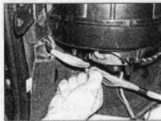
10.14a Release the wiring harness from the cable ties and clips on the blower motor ...
