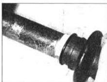
3.21c ... and seat the gaiter inner end on top of the plastic bush
