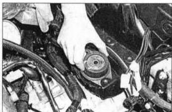
7.16 Undo the two retaining bolts and remove the left-hand engine/transmission mounting
