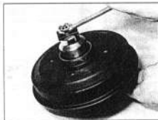
12.9b ... then draw the bearing into position
