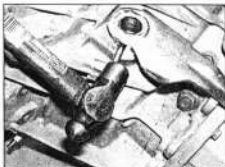
5.10 Secure the release lever to the shaft by tapping in a new roll pin or retaining pin
