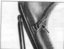
26.62b ... and disengage their lower locating pegs (arrowed) from the intermediate trim panel
