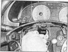
4.3 Disconnect the wiring connector from the steering wheel switches circuit board
