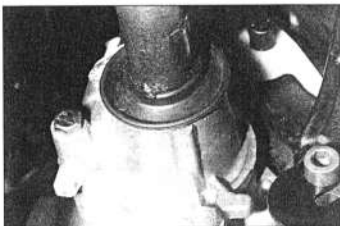
2.32 Secure the intermediate bearing in position, then slide the dust seal up tight against the driveshaft oil seal
