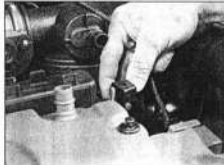
3.9 Remove the hose clip support bracket from the left-hand end of the coil module
