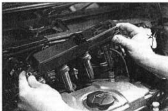
3.10b ... and lift the ignition coil module from its mounting studs
