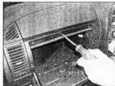
28.22a Undo the glovebox upper securing screws ...
