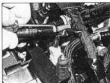
6.17 Disconnect the fuel supply and return hose quick-release fittings – 2.0 litre engines
