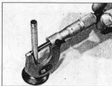
6.11 Measuring a valve stem diameter
