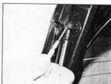
15.6 Prise out the support strut clips and pull the struts from the balljoints on the tailgate
