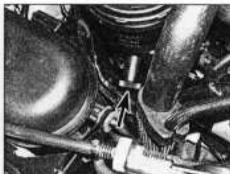
4.14 Fuel filter water drain plug location (arrowed) – 2.0 litre engines
