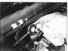
3.5 Carefully prise the bellcrank link rod balljoint off the transmission lever - MA transmission
