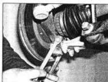
2.9 Undo the nut and withdraw the lower suspension arm balljoint clamp bolt from the swivel hub
