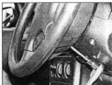
22.7 Move the steering wheel as necessary for access, and undo the two air bag securing screws
