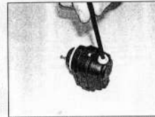
7.8 Before refitting the adjuster motor, turn the height control adjuster using an Allen key to fully extend the adjuster rod
