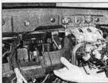
10.13b Release the duct from the heater unit and withdraw it from the steering column support bracket
