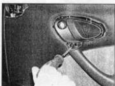
12.6 Undo the trim panel retaining screw from the base of the interior handle ...
