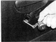
13.15b ... then remove the lock cylinder and link rod from the outside of the door
