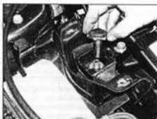
5.27b ... then undo the domed buffer nut, and the upper bracket retaining nut
