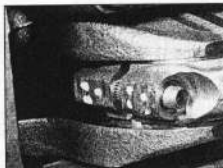
10.3 Connecting rod and big-end bearing cap identification marks (No 3 shown)
