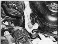
3.13 Disconnect the wiring connector from the coolant level sensor
