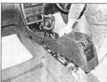
27.11 Pull the centre console rearward, then lift it up and over the handbrake lever and gear/selector lever
