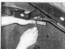
26.30a Carefully prise the luggage compartment light unit from the side panel ...
