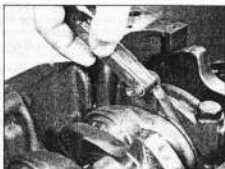
14.3 Checking crankshaft endfloat using feeler blades
