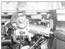
19.5 Depress the retaining lug on the side of the lock...
