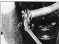
18.6 Remove the turbocharger oil return hose (arrowed) from the pipe on the cylinder block – DHY (XUD9TE engine) models
