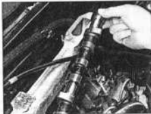
11.9 ... then lift the camshaft away from the cylinder head – 8-valve engines
