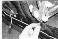
14.28 Undo the bolt securing the base of the lifting channel to the rear door ...
