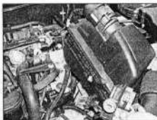
4.10 Lift the air cleaner housing upwards at the rear and disengage the two front locating lugs
