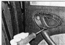
12.17 Undo the trim panel retaining screws, one at the base of the interior handle...
