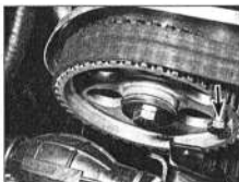
3.6a Bolt (arrowed) inserted through timing hole in the camshaft sprocket
