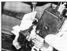
16.12a Withdraw the lock housing assembly from inside the tailgate and disconnect the operating rod ...
