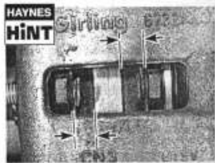
For a quick check, the thickness of friction material on each brake pad can be measured through the aperture in the caliper body.
