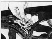
5.10 Lift out the relay mounting plate, disconnect the wiring and remove the relevant relay
