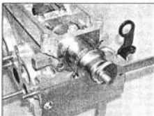
11.26b ... then use a bolt and socket or similar arrangement to press the seal into place – 2.0 litre engines
