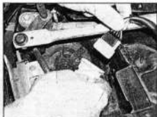
14.6 Separate the two halves of the wiper motor wiring connector
