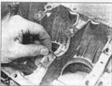
18.16 On TU series engines, the grooved bearing shells are fitted to Nos 2 and 4 main bearing journals
