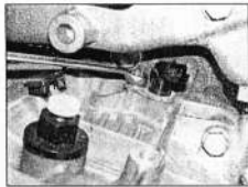
13.11 Slacken the bolt securing the sensor to the bellhousing
