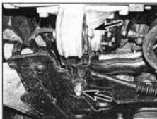
5.26 Undo the nuts and bolts (arrowed) and remove the rear engine mounting connecting link
