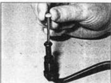
18.9 Removing the filter from the oil feed pipe – DHY (XUD9TE engine) models
