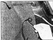
26.32 Undo the bolt securing the tie-down strap to the rear of the side panel - Hatchback models
