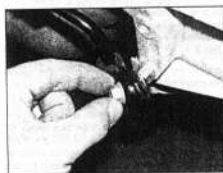
5.13a Release the power steering pipe retaining clips on the transmission ...
