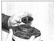
5.8i Locate the collar over the mounting plate . . .
