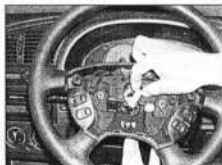
17.14 ... and feed the wiring harness through the wheel as it is withdrawn
