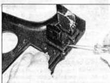
4.19a Depress the retaining catches at the rear of the facia lower switches ...
