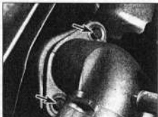
21.7b Catalytic converter-to-turbocharger securing bolts (arrowed) – viewed from engine compartment
