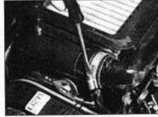
20.2b ... and the air inlet duct from the right-hand end of the intercooler
