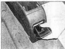
27.2a Remove the ashtray from the rear of the centre console ...
