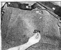
26.33b ... then undo the screw securing the hook to the side panel - Hatchback models
