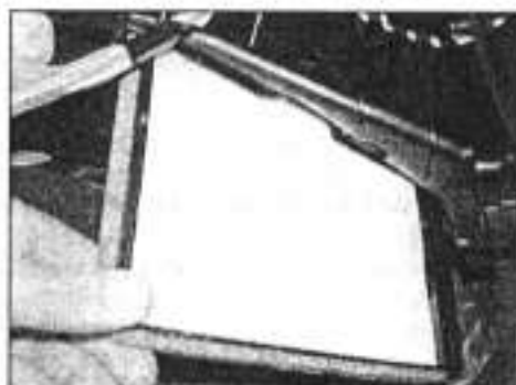
7.3 Withdraw the pollen filter from the housing
