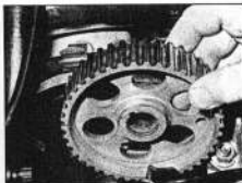
8.7 Withdrawing the camshaft sprocket
