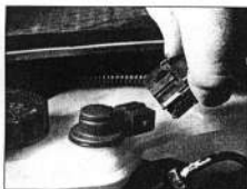
13.2 Disconnecting the wiring connector from the master cylinder fluid level sender
