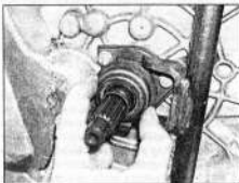
5.2 Unhook the release bearing from the fork, and slide it off the input shaft
