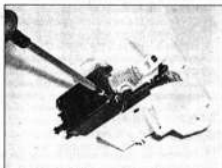
16.14a Undo the central locking motor retaining screw ...
