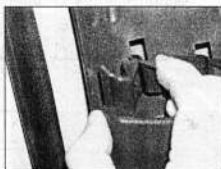
26.53 Release the lower trim panel upper securing clips
