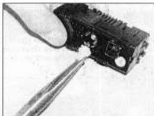
6.23 Twist the bulbholder anti-clockwise and remove it from the rear of the clock
