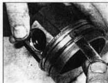
14.2 Removing a piston ring with the aid of a feeler blade
