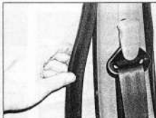
26.50 Prise the weatherstrips from both sides of the centre pillar
