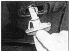
5.15b ... release the rear of the unit from the front wing and withdraw the light unit
