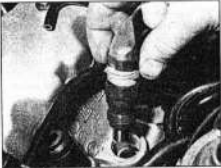
10.6 Unscrew the injectors, and remove them from the cylinder head
