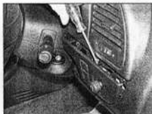
4.21a Carefully prise the driver's side switch panel from the facia ...
