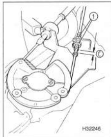
5.4 Reconnect the cable, and check that clearance (c) is as given in the text. Adjust by repositioning the locknuts (1) – 4 HP 14 transmission
