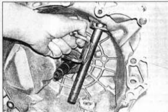
5.4 Lift the release shaft up to disengage it from the lower bush, and manoeuvre it from the transmission
