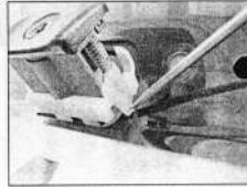
16.11 Depress the tabs on each side of the lock housing
