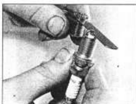
22.12 Measuring the spark plug gap with a feeler blade
