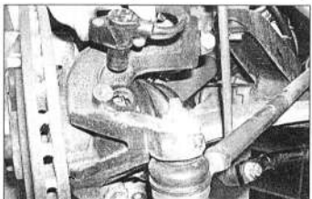
24.20b ... and withdraw the front wheel sensor from the swivel hub
