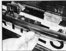
16.10b ... and remove the moulding from the tailgate
