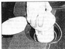
8.7a Lift the fuel pump and sender unit assembly out of the fuel tank ...
