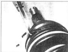
3.21h Bend the clip end back over the buckle, then cut off the excess clip
