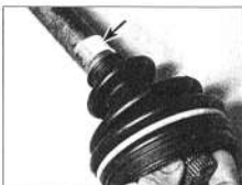
3.21b ... then slide on the new plastic bush (arrowed), and seat it in its recess in the shaft. Slide the gaiter onto the shaft ...
