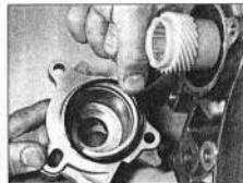
6.7b ... and remove the speed sensor extension housing, O-ring and drive pinion from the transmission (transmission removed for clarity)
