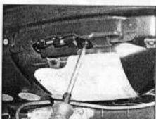
15.8a Unscrew the two lock securing screws, and withdraw the lock from the tailgate ...
