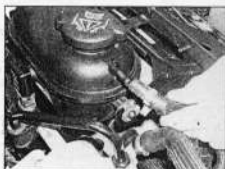
3.12 Disconnect the upper hose at the coolant expansion tank
