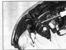
7.7a To remove the headlight electric adjuster motor, lift the tag and turn the adjuster motor through 90°...
