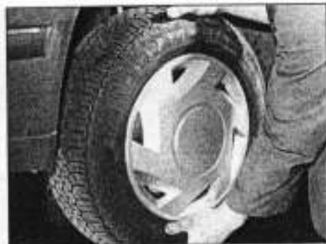
10.4 Check for wear in the hub bearings by grasping the wheel and trying to rock it
