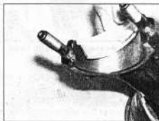
20.5a Fit the big-end bearing shells ensuring that the tab engages in the notch in the connecting rod ...
