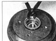
12.2 Extracting the rear hub bearing circlip
