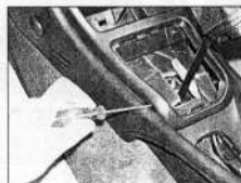
27.7a Release the gear lever gaiter surround retaining clips ...
