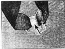
25.23 Rear centre seat belt retaining bolt (arrowed)
