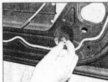
14.10 Unscrew the nut securing the lower end of the rear lifting channel to the door
