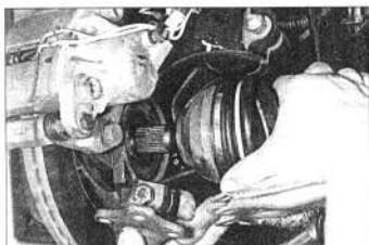
2.31 Pull out the swivel hub assembly, and locate the outer constant velocity joint splines with those of the swivel hub
