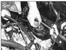
18.21a Remove the centre nut and washer from the left-hand mounting ...
