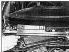
14.5 Undo the securing screws and remove the wiper motor cover panel
