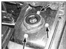
4.8 Suspension strut upper mounting bolts (arrowed)
