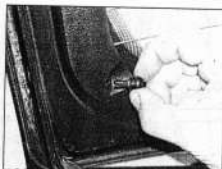
26.61b ... then remove the lifting string pegs from the tailgate side trim panels
