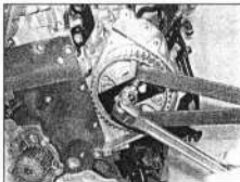
9.56 Using the home-made tools to remove the fuel pump sprocket - 2.0 litre engines
