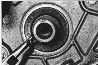
17.2 Using a self-tapping screw and pliers to remove the crankshaft oil seal
