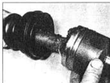
3.42a Release the inner gaiter retaining clips, and remove the joint outer member
