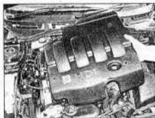
4.2 Undo the four plastic nuts and lift off the engine cover
