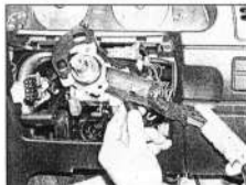
19.6 ... then withdraw the lock assembly and feed the wiring through the column tube
