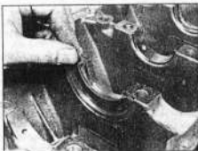
16.38 Refitting a crankshaft thrustwasher – TU series aluminium block engines
