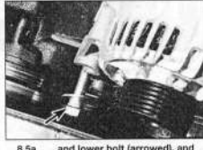
8.5a ... and lower bolt (arrowed), and remove the alternator – 1.8 litre petrol engine model
