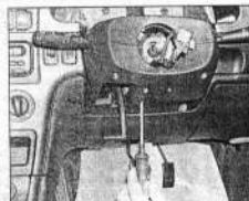
4.7b ... and the lower screw securing the steering column shrouds to the steering column
