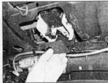
16.8 Remove the plastic cover over the central locking motor and lock housing assembly
