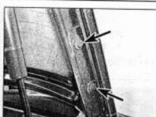
15.7a On Hatchback and Coupé models, unscrew the two bolts (arrowed) securing the hinges to the tailgate ...
