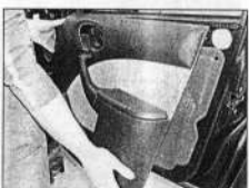
12.10 Pull the trim panel outwards, then lift it up and remove it from the door
