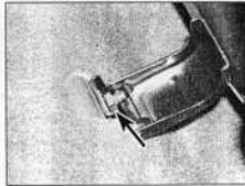
24.15 Rear seat cushion retaining bolt (arrowed)
