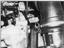
6.9 Coolant temperature sensor (arrowed) – 2.0 litre diesel engine models
