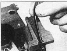
18.70 Fitting a sealing strip to No 1 main bearing cap - XU series engines
