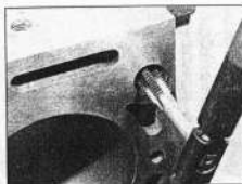
12.9 Cleaning a cylinder block threaded hole using a suitable tap
