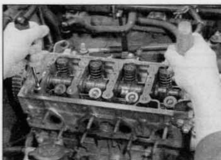
11.16 Use two stout screwdrivers to rock the cylinder head free from the block – 1.4 litre engines
