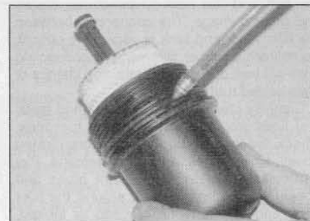
3.14b ... and apply a little clean engine oil to the O-ring seal
