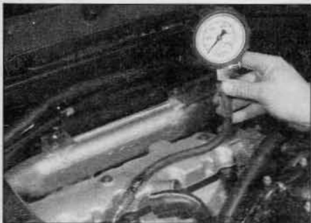
2.2 Performing a compression test
