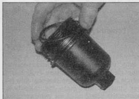
3.11b ... and recover the O-ring seal
