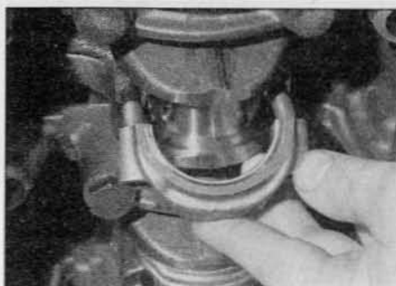
9.5 Remove the big-end bearing shell and cap
