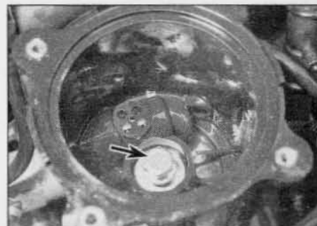
8.8a Unscrew the securing bolt (arrowed) ...
