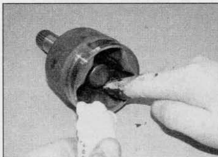
4.22g ... then pack the outer member with the remaining grease
