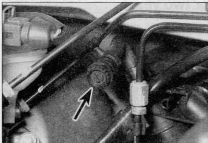
25.4a Heater hose bleed screw (arrowed)
