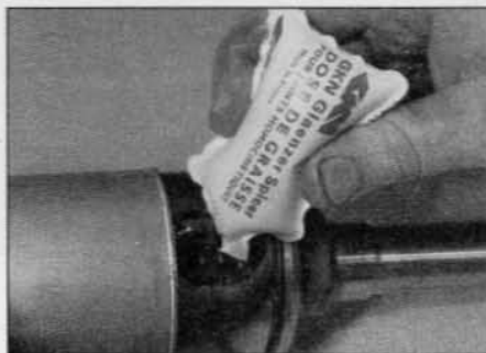
3.26b ... then apply the remainder of the grease ...
