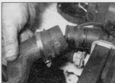
2.5 Disconnecting the radiator top hose
