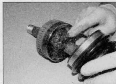
4.12j ... working it well into the ball tracks while twisting the joint
