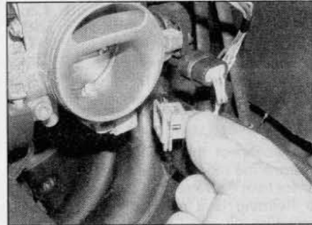
13.47 Disconnect the wiring connector . . .
