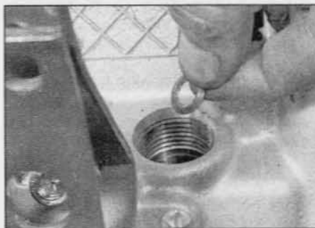
10.9b ... fire seal washer ...
