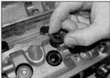
8.3b . . . then place the spring retainer over the spring
