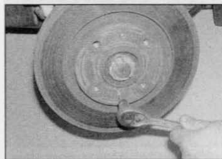
6.8a Undo the two retaining screws ...
