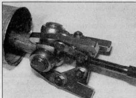
3.17a Using a three-legged puller to remove the inner tripod joint
