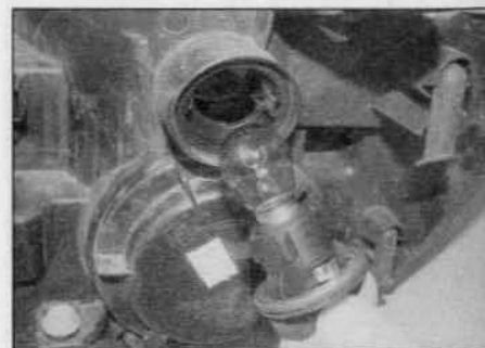
5.25a Rotate the direction indicator bulbholder anti-clockwise to release it...
