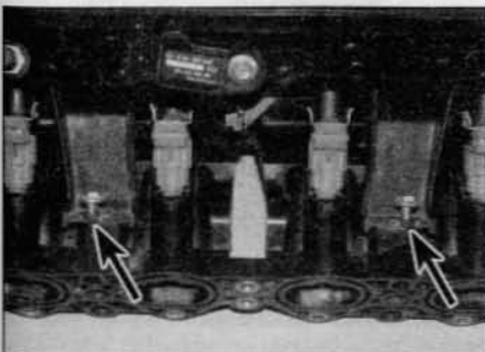
13.14 Undo the two bolts (arrowed) and remove the fuel rail from the manifold – 1.6 litre models
