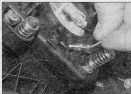
21.9a Disconnect the horn push earth connector ...
