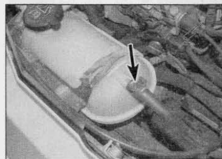
3.10 Disconnect the upper hoses (left-hand hose arrowed) at the coolant expansion tank on diesel models
