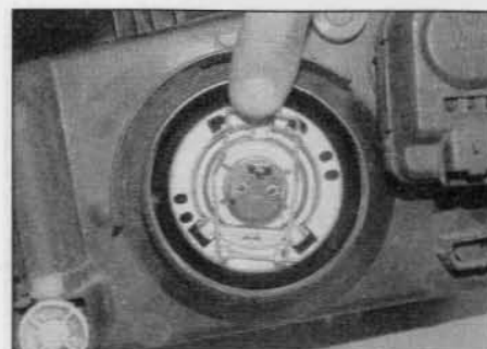
5.3a Release the spring clip ...
