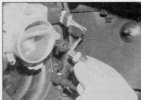
13.22 Disconnect the wiring connector from the throttle potentiometer ...
