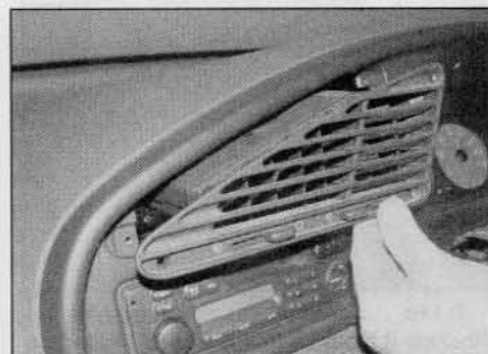
9.3b ... and remove the centre vent unit from the facia – early models
