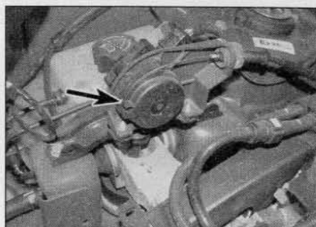
4.4 Detach the accelerator inner cable from the pedal position sensor (arrowed) – later 2.0 litre models
