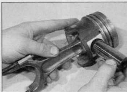
13.13b ... withdraw the gudgeon pin ...
