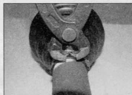
4.12m Locate the gaiter inner end in the shaft groove or against the mark made on removal, slide the clip in place and compress the raised portion using pincers or side-cutters
