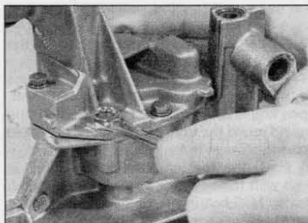
15.5a Remove the oil pump cover retaining bolts ...
