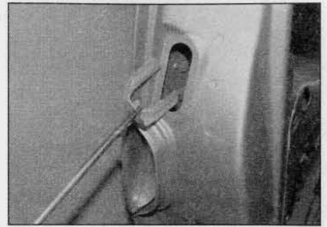
12.10b Using a suitable removable tool, extract the retaining clip from the lock cylinder
