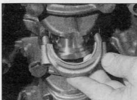
10.5 Removing a big-end bearing cap and shell
