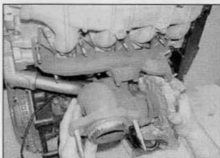
18.24a Withdraw the turbocharger and manifold ...
