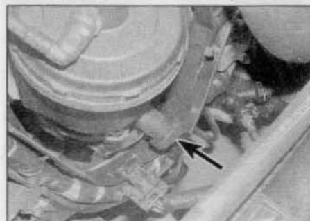
4.13 Fuel filter drain plug location – 2.0 litre engines
