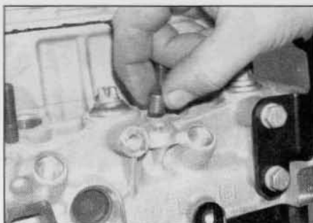
15.18 Recover the injector clamp locating dowel – 2.0 litre models
