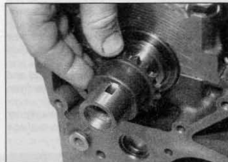
11.5b ... then slide off the drive sprocket ...
