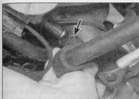
13.8 Disconnecting the coolant hose (arrowed) from the rear of the cylinder head
