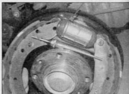
5.20 Manoeuvre the partially assembled brake shoe assembly into position on the backplate
