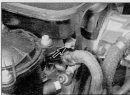
3.5 Front air distribution housing securing bolt (arrowed)
