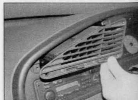
30.5b ... and remove the centre vent unit from the facia
