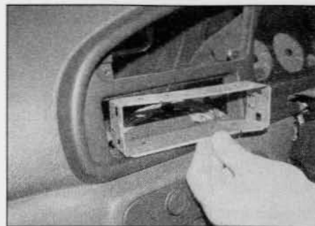
17.6 ... then remove the mounting frame from the facia
