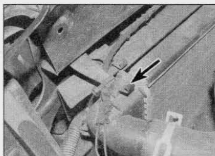
3.6 Lift the ends of the radiator retaining clips (arrowed) and move the top of the radiator toward the engine
