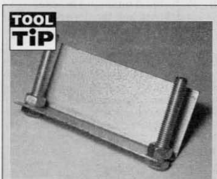
TOOL TIP Fabricated tool for holding tensioner plunger in the engine mounting bracket.
