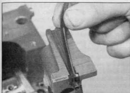
18.9a Fitting a sealing strip to No 1 main bearing cap
