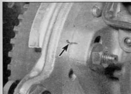
5.15 Mark the injection pump in relation to the mounting bracket (arrowed)
