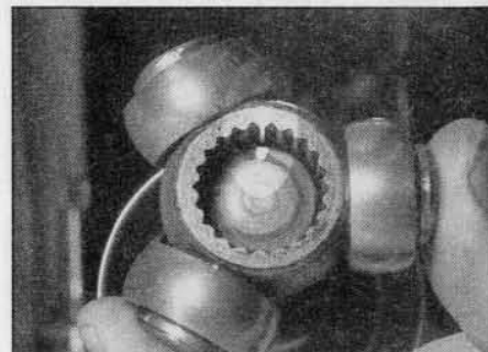
3.17b Withdrawing the inner tripod joint. Note the alignment marks (made in the previous paragraph)
