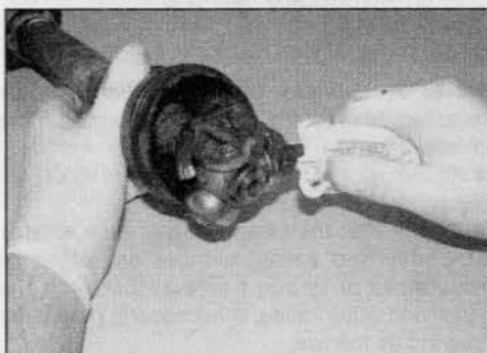
4.22d Pack the tripod and the gaiter with half the recommended quantity of the grease ...
