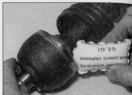
3.8 Pack the joint with the grease supplied in the repair kit
