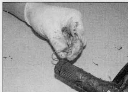
4.6 Remove the circlip from the groove in the driveshaft splines
