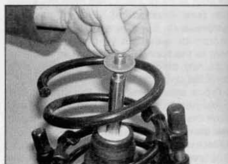
5.8e Place the flat washer in position ...
