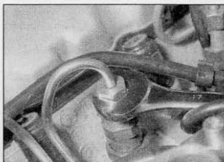
15.3 Unscrewing an injector pipe nut – 1.9 litre models
