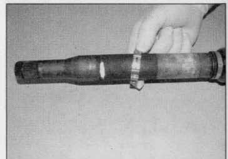
4.12a Slide the new gaiter inner retaining clip on the driveshaft . . .
