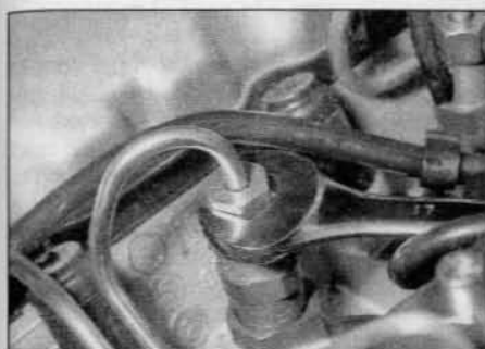
5.12a Unscrewing a fuel pipe-to-injector union
