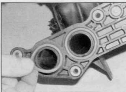
14.10 Ensure the new sealing rings are correctly fitted to the manifold prior to refitting
