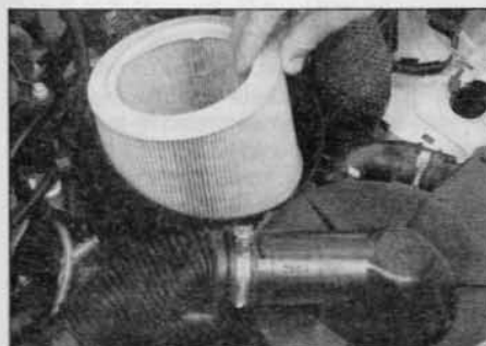
20.3 ... and withdraw the filter element – XUD series engines
