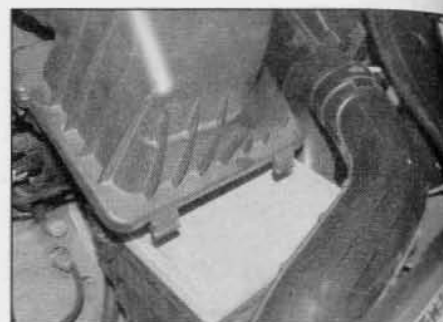
12.45b ... disengage the two retaining lugs and lift the lid from the air cleaner housing – 2.0 litre models
