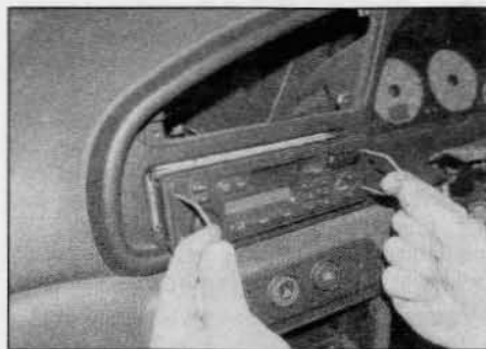
17.3 Insert the removal tools into the holes on the audio unit and withdraw the unit from the facia
