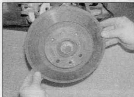
6.8b ... and remove the front brake disc
