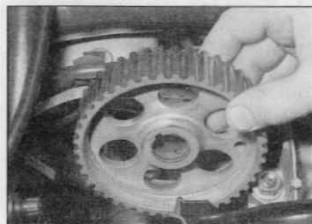
8.7 Withdrawing the camshaft sprocket
