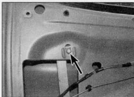
15.10 Undo the upper bolt (arrowed) securing the window glass rear guide channel to the door
