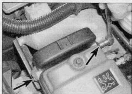
5.1a Unscrew the retaining bolts (arrowed) ...
