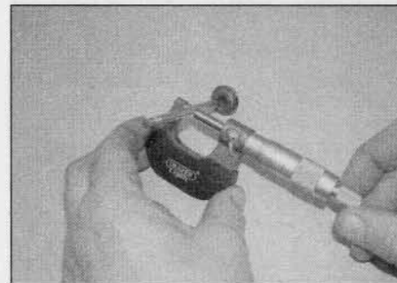
7.10 Measure the valve stem diameter with a micrometer
