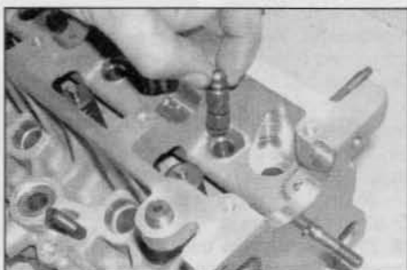
11.12b ... and hydraulic tappets out from the cylinder head – 2.0 litre engines
