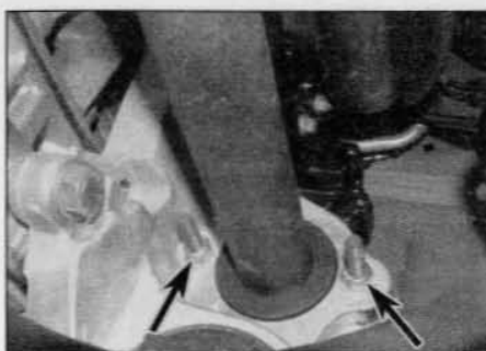
2.13 On the right-hand driveshaft, slacken the intermediate bearing retaining bolt nuts (arrowed), then turn the bolts through 90°
