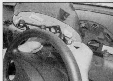
9.12 Turn the instrument panel over and disconnect the wiring connectors – later models
