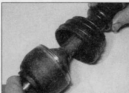
3.7 Sliding the outer joint gaiter onto the driveshaft
