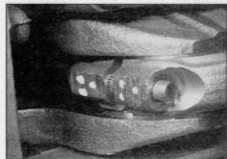
10.3 Connecting rod and big-end bearing cap identification marks (No 3 shown)
