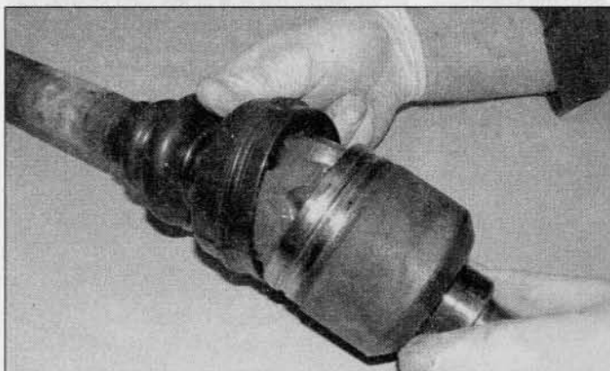
4.17a Withdraw the joint outer member from the tripod . . .
