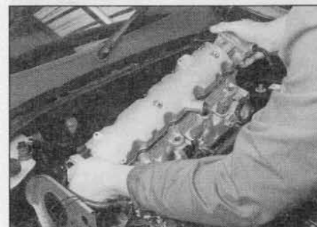
13.22 Removing the cylinder head
