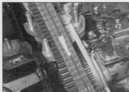
7.10a Mark the timing belt with an arrow to indicate its running direction
