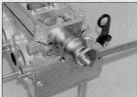
10.4 Using a socket, a length of stud and a nut to press the camshaft oil seal into position
