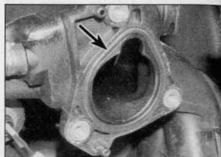
12.5 On refitting ensure the new sealing ring is correctly fitted to the manifold – 1.4 litre model shown
