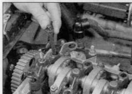
11.14 Slacken and remove the cylinder head bolts – 1.4 litre engines
