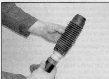
5.8b Fit the piston dust cover ...
