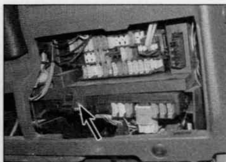
22.5 On early models, undo the retaining screw (arrowed) then release the clip and pivot the BSI unit downwards
