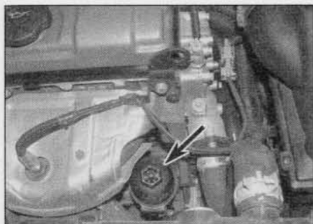
3.7 Cartridge type oil filter housing location (arrowed) - later models
