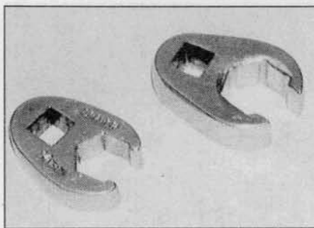
2.7 Two crow-foot adaptors will be necessary for tightening the fuel pipe unions
