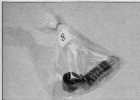
7.8 Place each valve and its associated components in a labelled polythene bag
