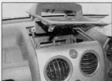
31.6 Carefully prise the multi-function display surround from the fascia
