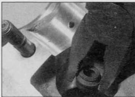
7.5e Remove the valve stem oil seal using a pair of pliers ...
