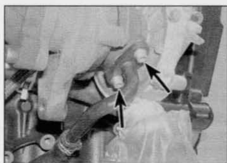
18.20a Undo the oil return pipe flange securing bolts (arrowed) ...
