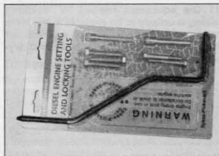
3.5a Suitable tools available for locking the engine in the TDC position
