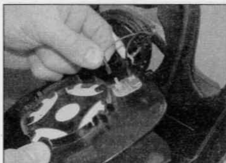
19.7 Withdraw the mirror glass, and disconnect the wiring connector
