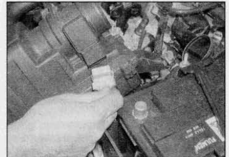
3.23a Disconnect the wiring connector from the airflow meter . . .
