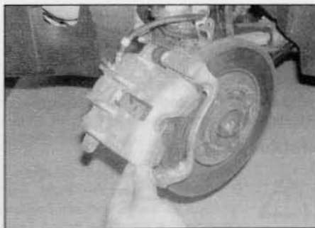
4.5 Slacken the upper guide pin bolt, and pivot the caliper upwards off the brake pads
