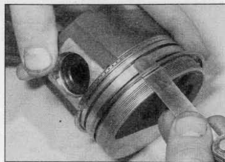
12.2 Remove the piston rings with the aid of a feeler gauge
