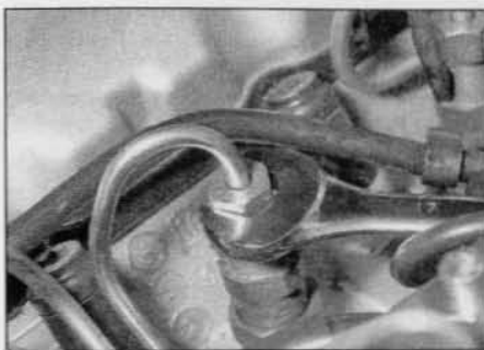
10.7 Unscrewing an injector pipe union nut
