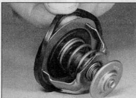
4.6 Removing the sealing ring from the thermostat flange
