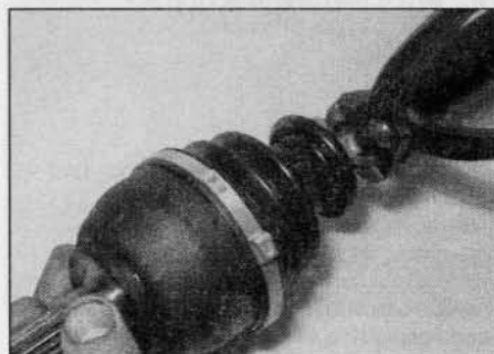
3.10 Securing a gaiter securing clip using side-cutters
