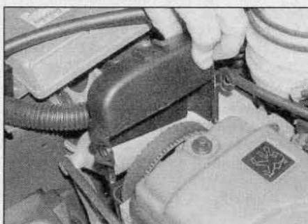
5.1b ... and remove the timing belt upper cover
