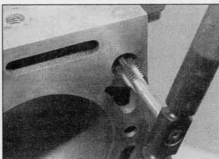
11.9 Use a suitable tap to clean the cylinder block threaded holes
