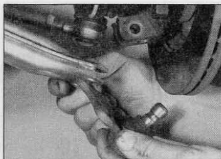
7.5b ... and remove the lower arm balljoint
