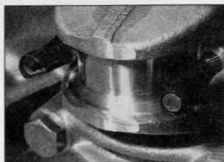
10.6 To protect the crankshaft journals, tape over the connecting rod stud threads
