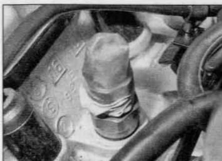
5.12b Cover the open end of the injector to prevent dirt entry
