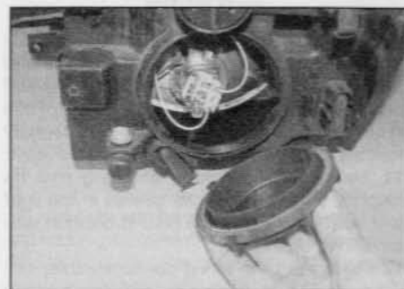
5.7 Remove the plastic cover from the light unit – later models
