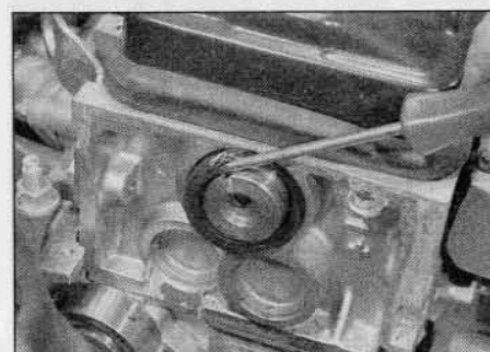
8.3 Carefully prise the camshaft oil seal out with a flat-bladed screwdriver
