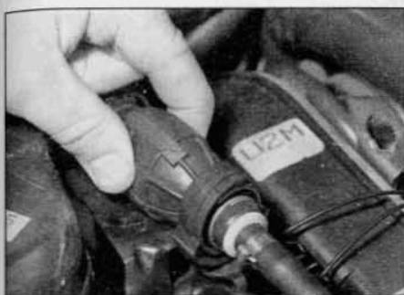
2.2 Hand-operated fuel system priming pump
