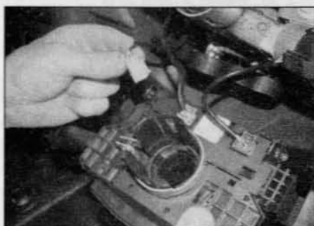
4.11d Turn the unit over and disconnect the wiring connectors - later models
