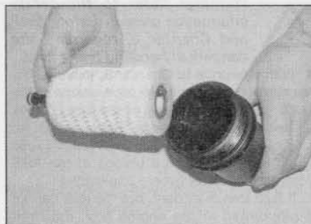
3.14a Fit the new element into the cover ...
