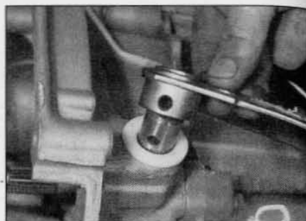
5.4b ... and remove the release lever from the top of the release fork shaft – MA5 and BE3/5 transmissions
