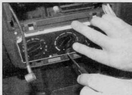
10.4 Release the lug at the lower centre of the heater/ventilation control unit and withdraw the unit from the facia
