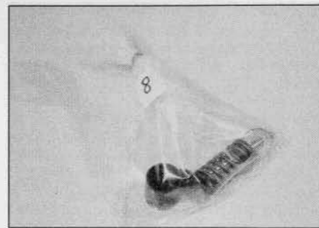
6.8 Place each valve and its associated components in a labelled bag
