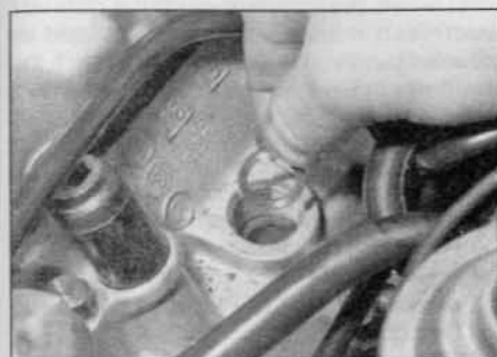
10.9a Removing a fuel injector copper washer ...
