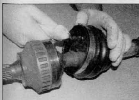
4.12k Fill the gaiter with the remaining grease ...
