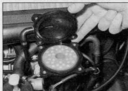
19.4 Lift off the fuel filter cover ...
