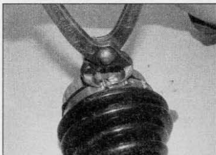
4.12n Secure the gaiter outer retaining clip in the same way
