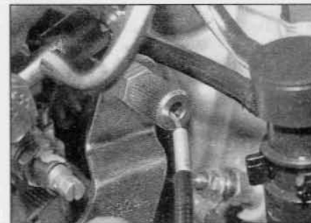
4.5 Sliding the fast idle cable from the adjustment screw – Bosch pump
