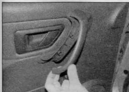
11.2b ... lift the handle trim off the upper locating lug and remove it from the handle
