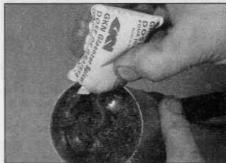
3.24 Pack the joint and gaiter/cover with grease
