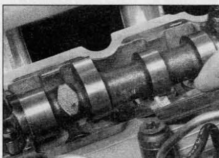
12.8 Measuring a valve clearance using a feeler blade
