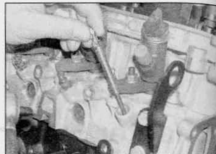
2.6 Unscrew the glow plug(s) and remove them from the cylinder head (2.0 litre engine shown with fuel rail removed)
