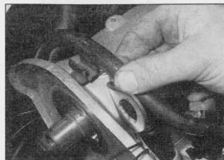
13.10 Unclip the fuel return hose from its brackets
