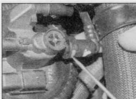
19.36 Disconnect the fuel supply and return hose quick-release fittings – later 2.0 litre engines
