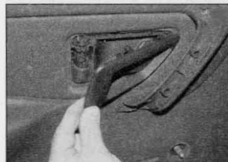
11.4b ... and disengage it from the handle
