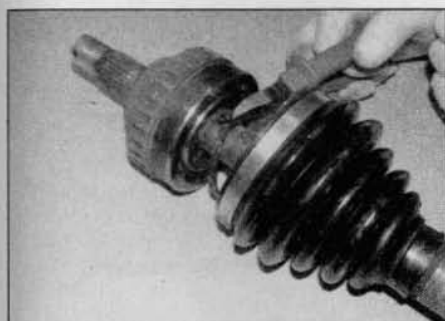
4.12h With the joint in place, cut off the cable tie
