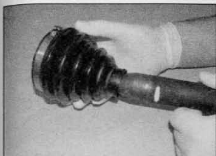
4.12b ... followed by the new gaiter with the outer retaining clip in place
