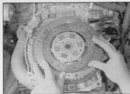
4.4b . . . then remove the friction disc, noting which way round it is fitted
