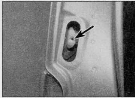
12.10a The lock cylinder retaining clip has a hole (arrowed) in its side to allow a threaded removal tool to be screwed into it
