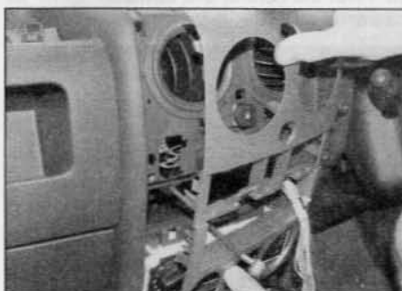
31.11 Carefully prise the centre panel away from the facia to release the side retaining clips
