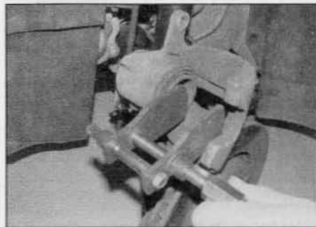
4.10a Use a suitable tool to retract the caliper piston ...
