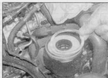
19.26b ... remove the metal sealing ring ...
