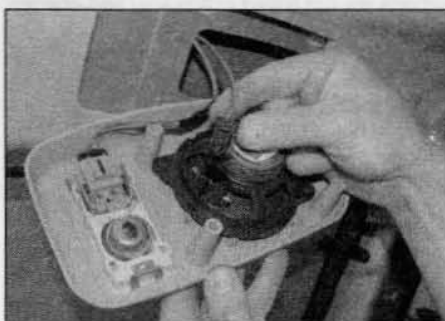
18.4a Disconnect the speaker wiring...
