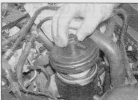
19.26a Lift off the filter housing cover ...
