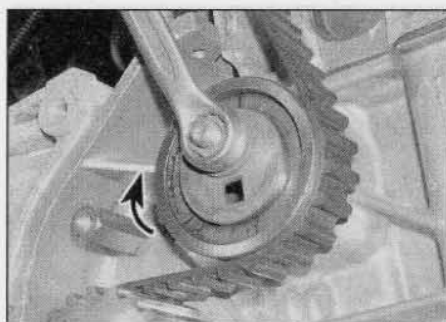
6.8 Slacken the nut then pivot the tensioner pulley clockwise to relieve the timing belt tension – 1.4 litre engines
